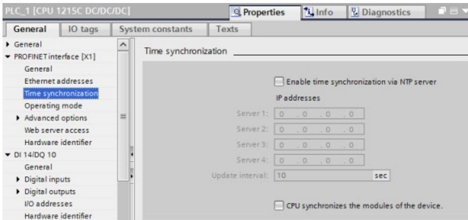
However, only configure one time source for the station. Receiving time synchronizations from more than one source (NTP server or CP module, for example) could cause conflicting time updates. Time synchronizations from multiple sources could adversely affect instructions and events based on time of day.
