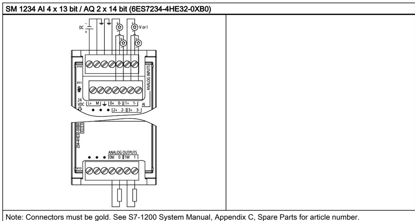
Table 13 Connector pin locations for SM 1234 AI 4 x 13 bit / AQ 2 x 14 bit (6ES7234-4HE32-0XB0)
