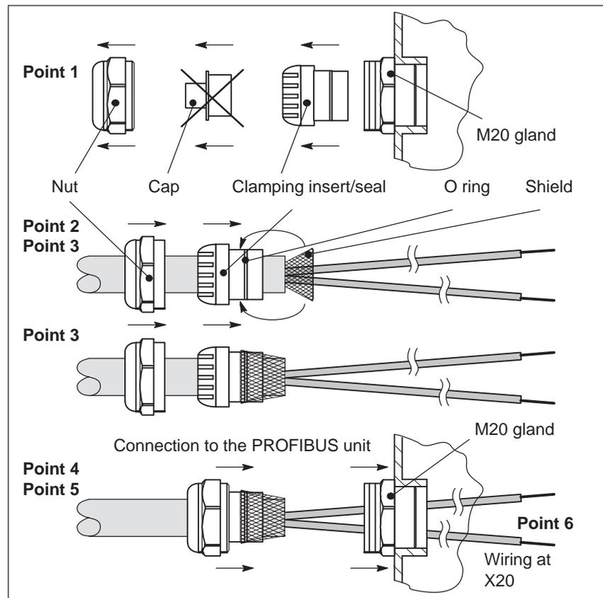
Fig. 2-24 How are the prepared cables installed?
