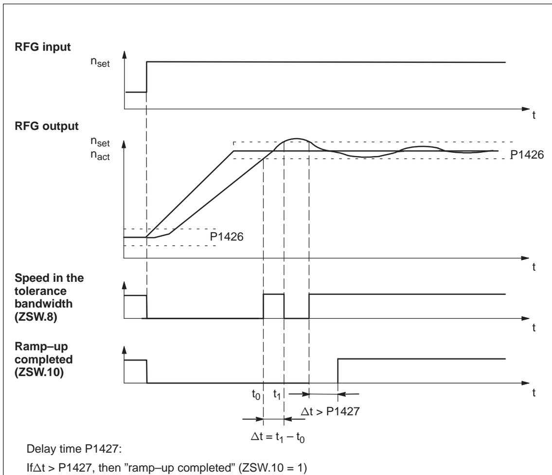
Fig. 5-2 Signal characteristics for the ramp-function generator
