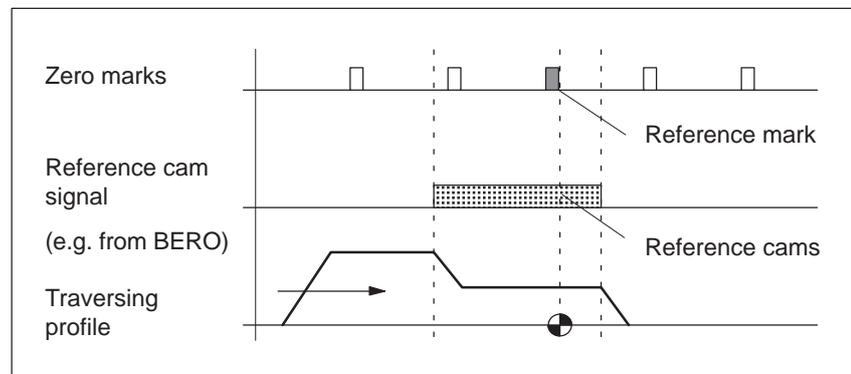
Fig. 5-5 Reference travel to BERO without direction reversal
