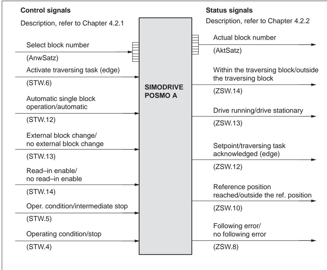
Fig. 5-4 Signals for traversing blocks and programs
