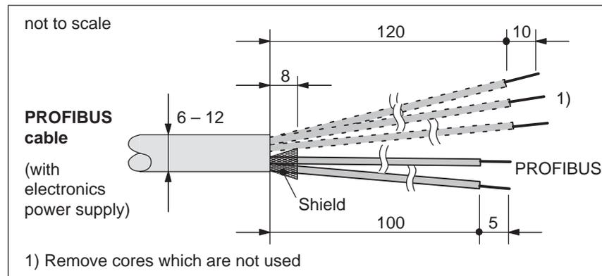
Fig. 2-20 Preparing The PROFIBUS cable with electronics power supply
