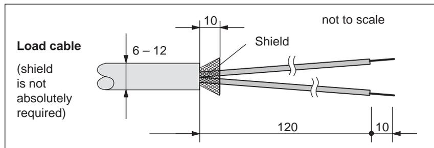
Fig. 2-18 Preparing Cable for the load power supply
