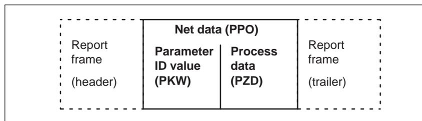
Fig. 4-2 Telegram structure for cyclic data transfer
