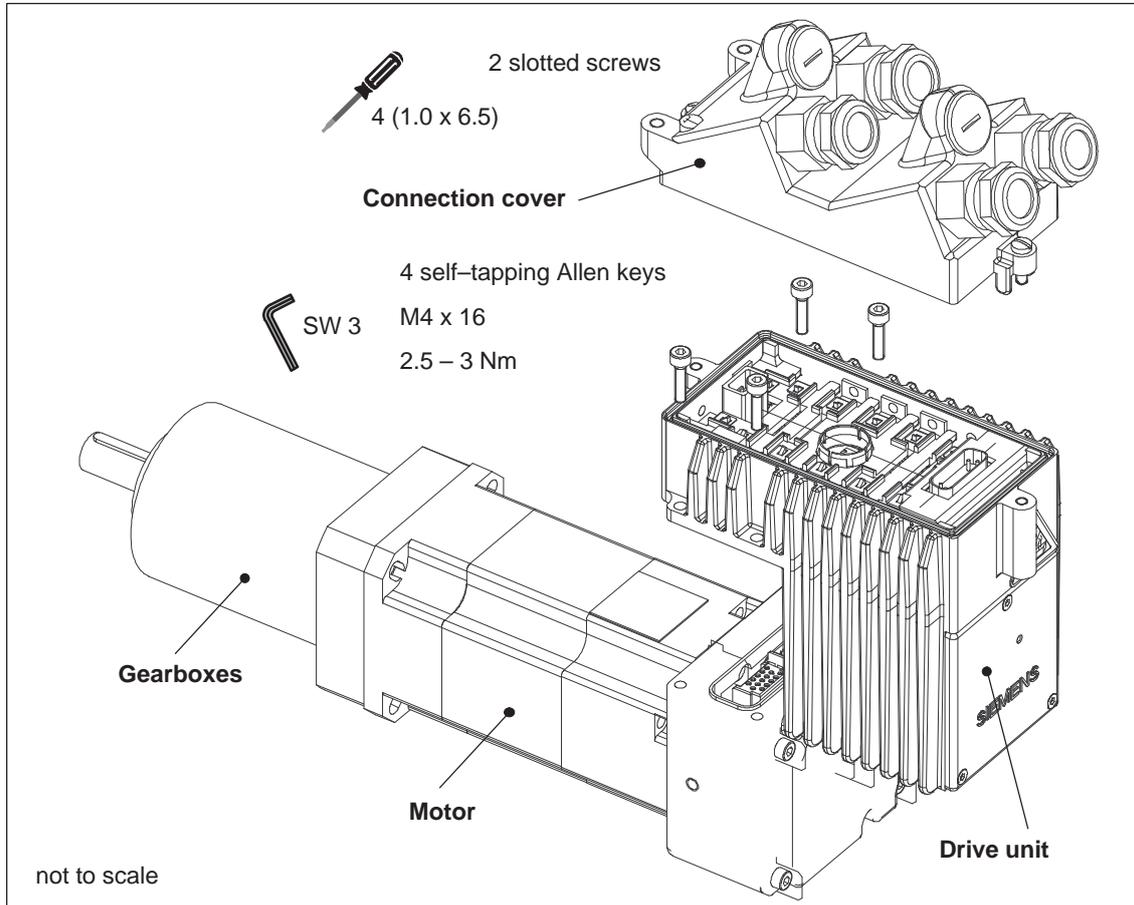
Fig. 7-1 Replacing the drive unit
