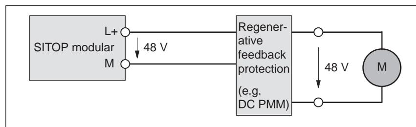
Fig. 2-5 SITOP modular 48 V/20 A with regenerative feedback protection
