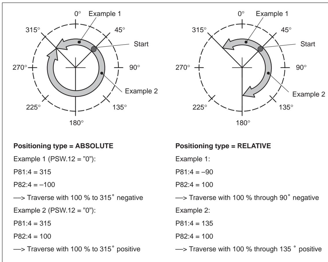
Fig. 5-12 Example: Programming rotary axes
