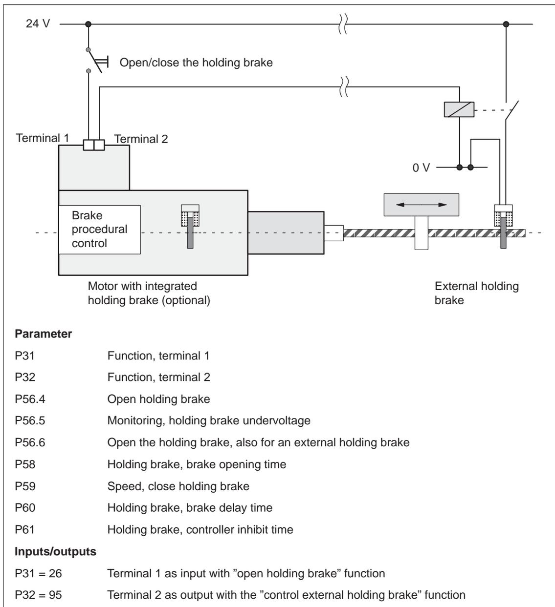
Fig. 5-20 Example: Integrated holding brake – external holding brake
