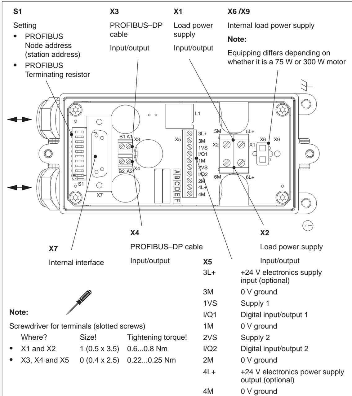
Fig. 2-15 SIMODRIVE POSMO A connection cover from the bottom
