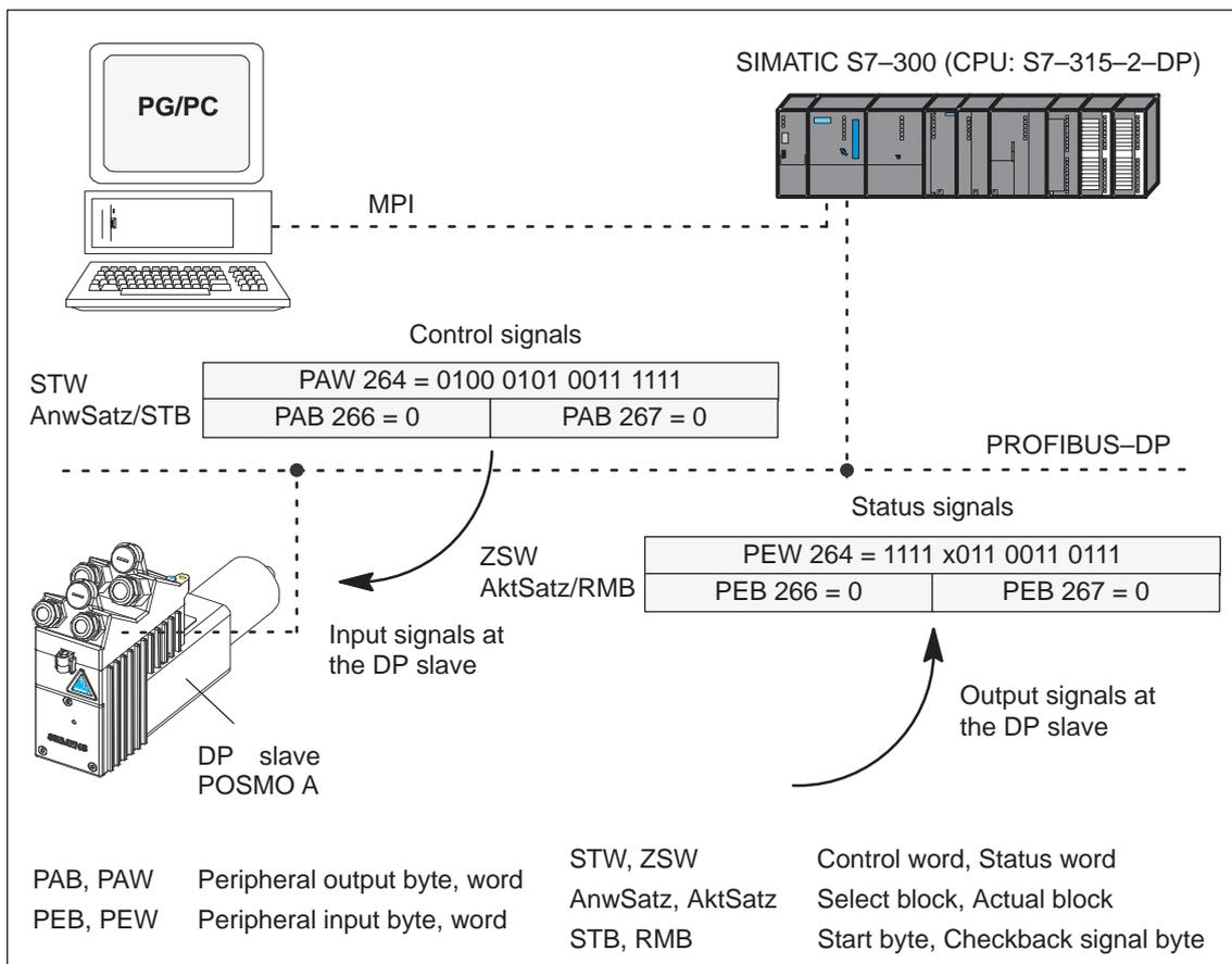
Fig. 4-3 Example: Operating the drive with jogging 1
