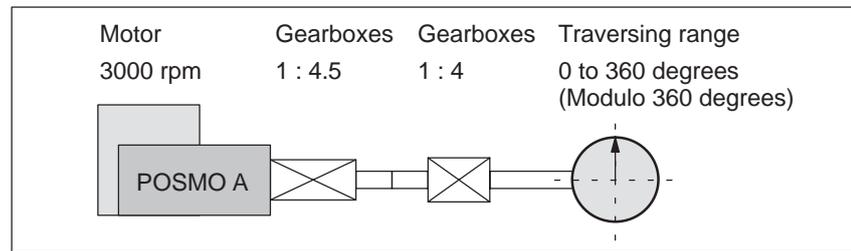
Fig. 3-8 Example: Parameterizing a rotary axis
