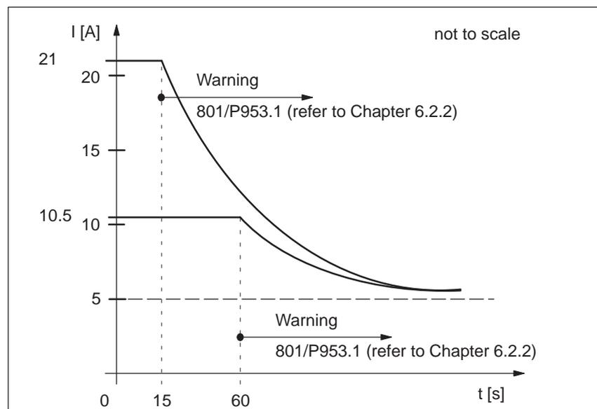
Fig. 2-8 i<sup>2</sup>t characteristic with 300 W motor
