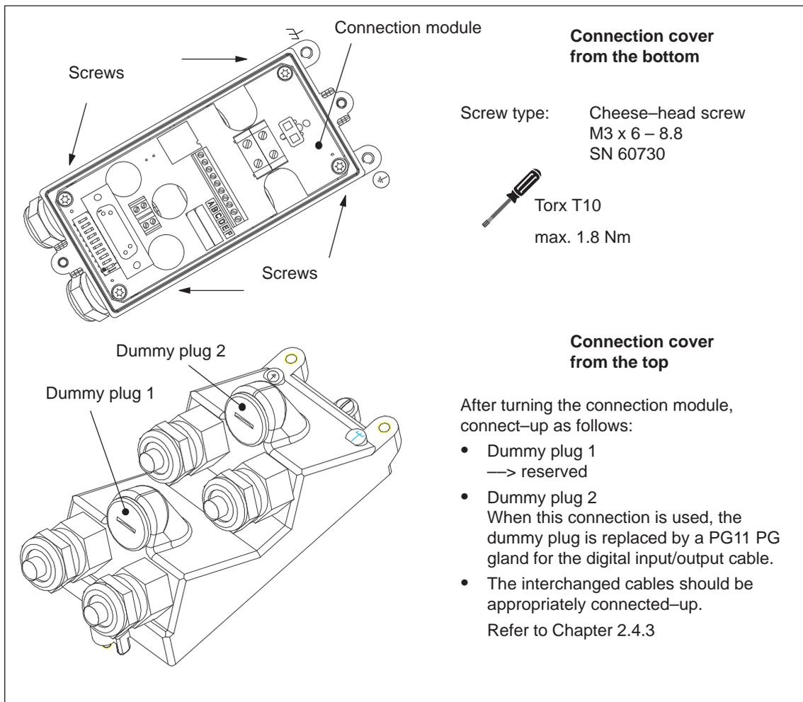
Fig. 2-16 Connection cover: Changing the cable outlet direction
