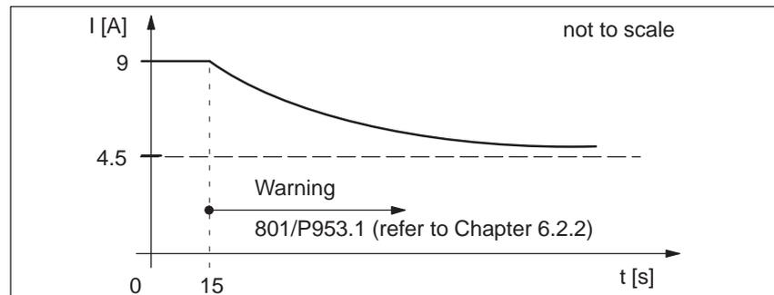
Fig. 2-7 i<sup>2</sup>t characteristic with 75 W motor
