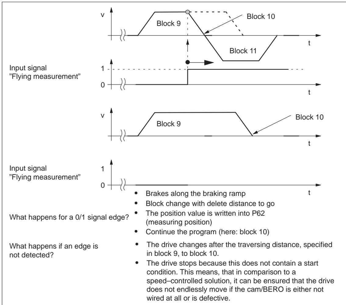
Fig. 5-10 Example: Position-controlled traversing motion to cam/BERO with stop
