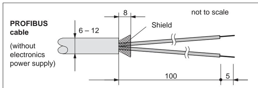
Fig. 2-19 Preparing the PROFIBUS cable
