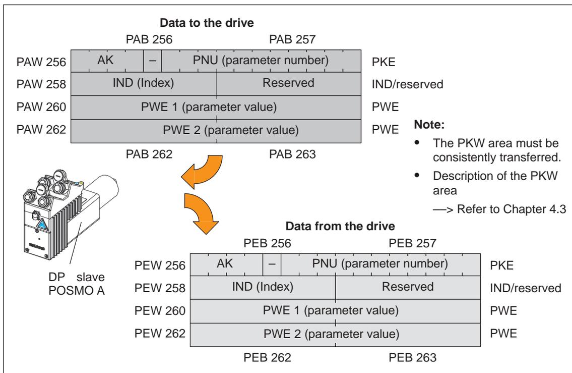
Fig. 3-4 Data transfer in the PKW area (addresses are only example addresses)
