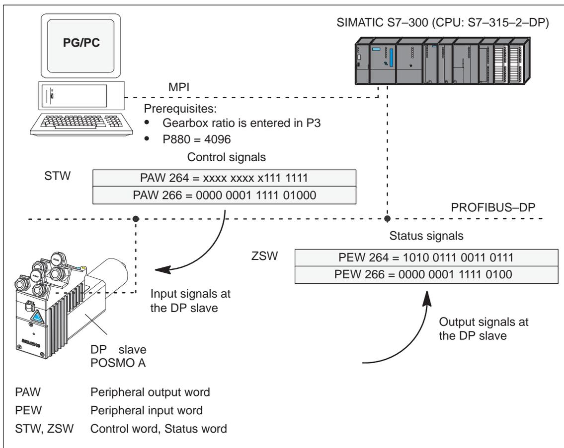
Fig. 4-4 Example: Drive should traverse with n-set
