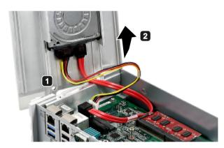
Set the rear panel with the drive vertically against the device's side panel and prop it up.
