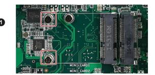
Remove the screw head of the full-size min card holder.
