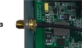
Secure the antenna in the device through the hole.
