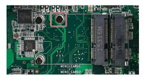
Remove the screw head of the half-size min card holder.
