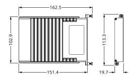
Figure 5.4 Line Module Dimensions
