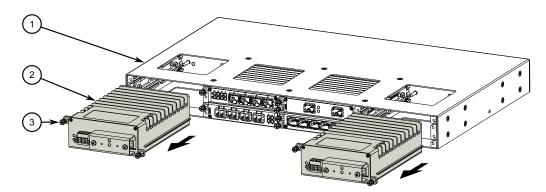
Figure 4.5 Removing a Power Supply
