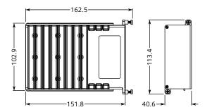
Figure 5.5 Power Module Dimensions
