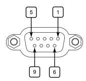
Figure 3.2 Serial DB9 Console Port
