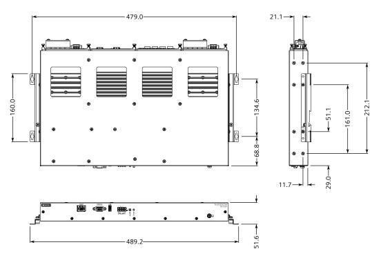
Figure 5.3 Panel and Din Rail Mount Dimensions
