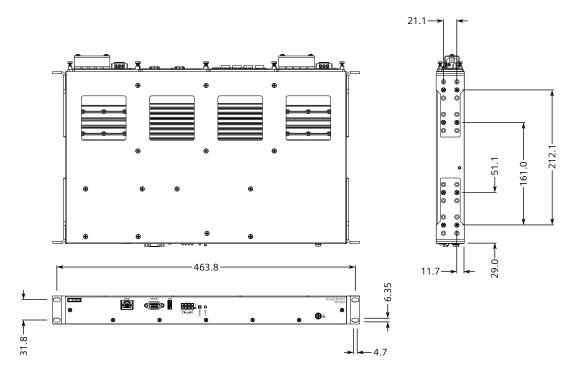
Figure 5.2 Rack Mount Dimensions
