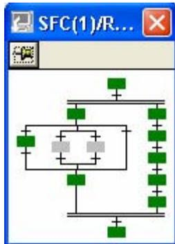
When the overview window is open, the current status of the SFC is displayed in color. The assignment of the colors to the respective states can be user-configured and is applied globally to all SFC in WinCC Explorer.
