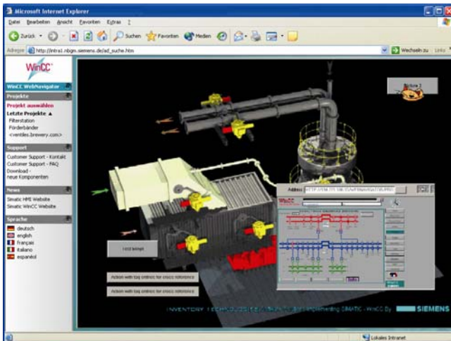
Figure 73 Operator control and monitoring of the plant via an intranet or the Internet
