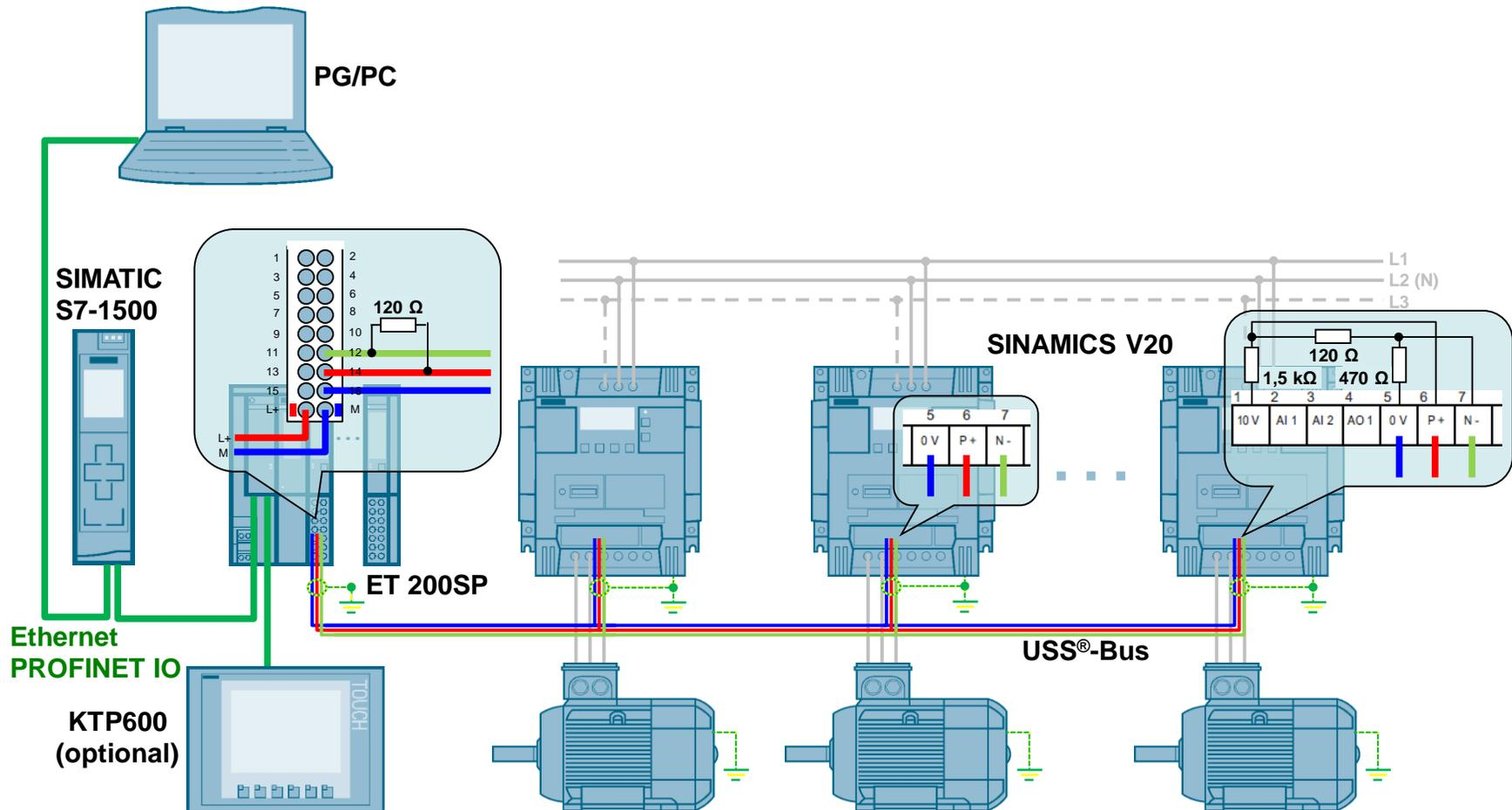
The bus cable consists of three wires and has to be shielded:
