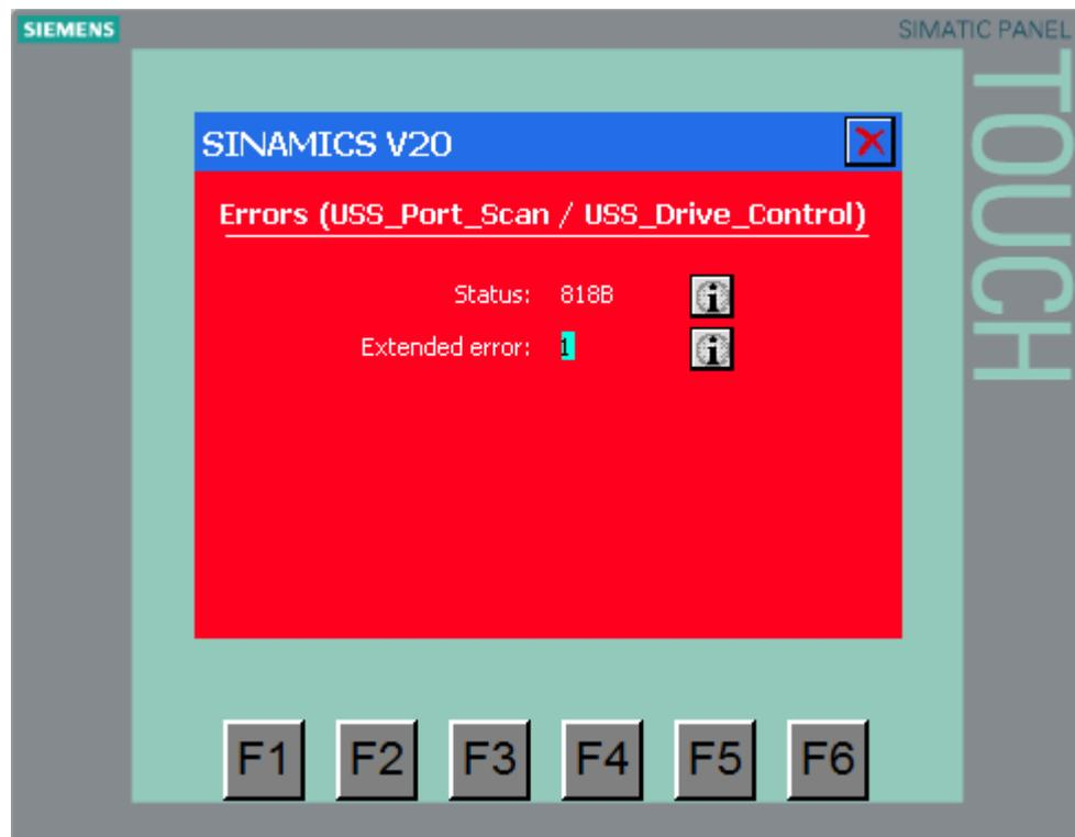
The error status and for some errors an expanded error information of the instruction creating the error is displayed which includes the address of the affected SINAMICS V20. The information always relates to the error that occurred last at the USS\_Port\_Scan or USS\_Drive\_Control. A new error overwrites the previous error information.
