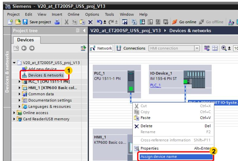
For this purpose, right click the PROFINET IO system in the “Devices & networks” editor on and select “Assign device name” from the context menu.
