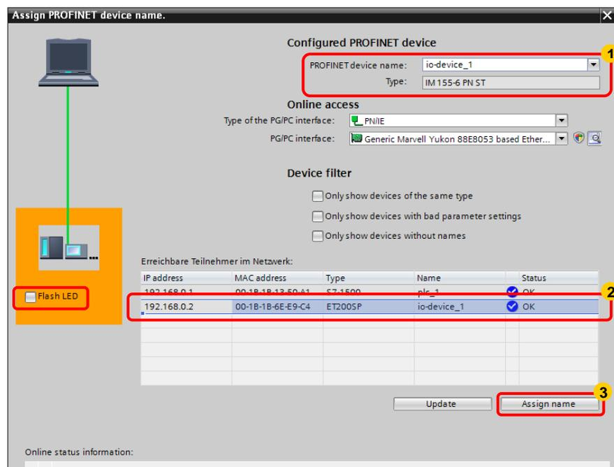
1. Select the configured PROFINET device – here the interface module of ET 200SP – from the dropdown menu.
