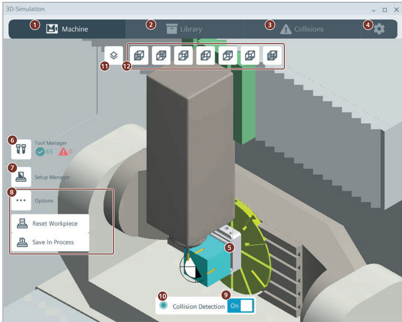
Figure 12-1 3D Simulation, operating areas and functions using the example of a milling machine
