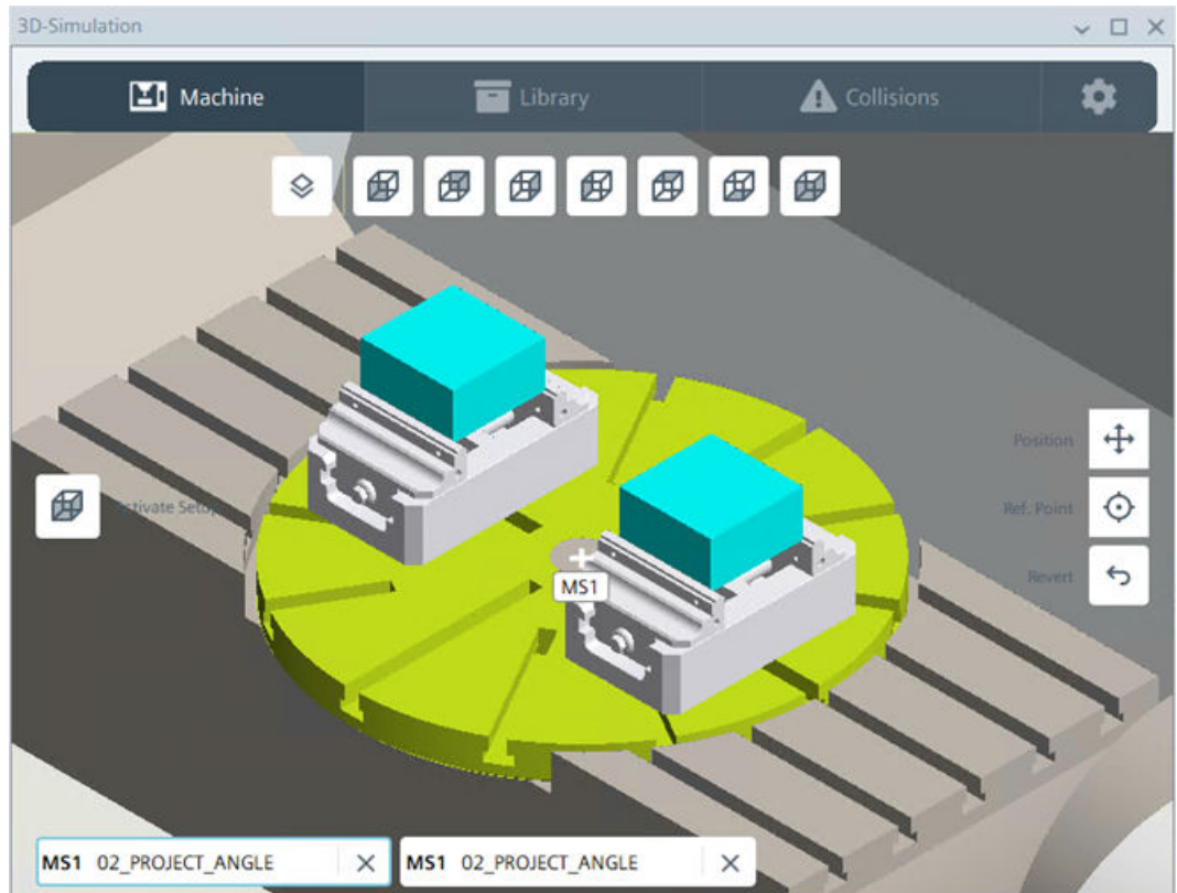
Figure 12-78 Example of milling machine with one Mount Station (MS1): Two setups are imported and activated
