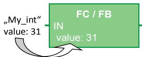
Figure 3-17: Copying of the value to the input parameter
