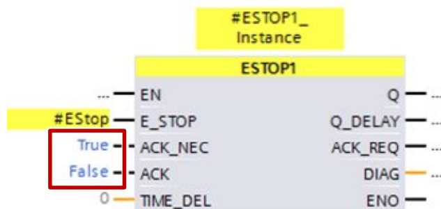
Figure 5-5: “TRUE” and “FALSE” signals as actual parameter
