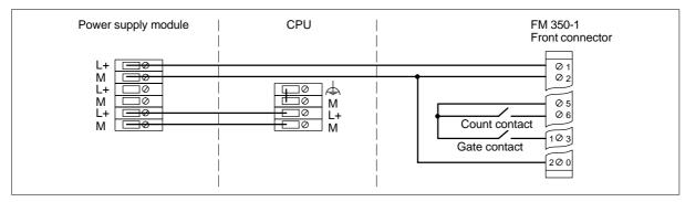
Insert the front connector in the FM 350-1 and snap it into place.
