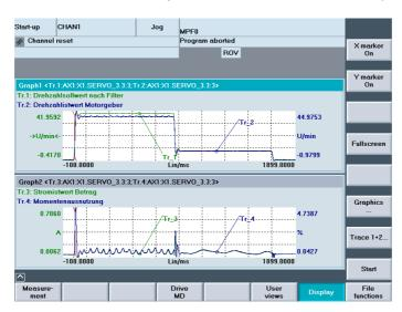
Figure 11-16 Drive trace recording
