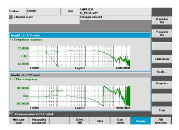
Figure 11-8 Optimized speed control loop
