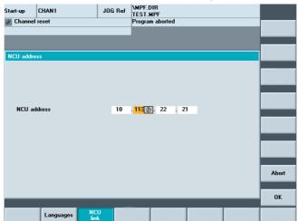
Figure 11-1 Startup tool -> 802D sl PCU IP address
