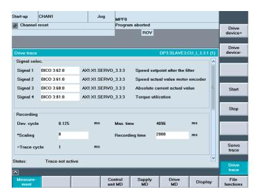
Figure 11-13 Basic "drive trace" display
