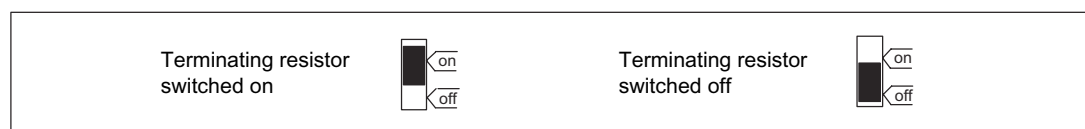
Figure 9-5 Terminating resistor switched on and off
