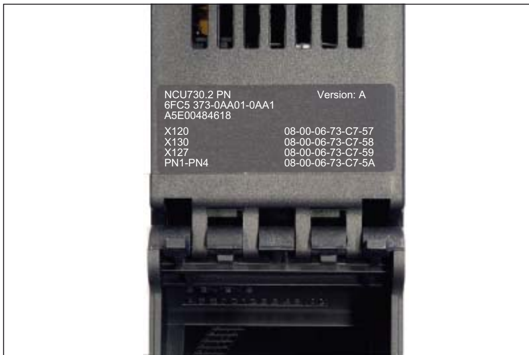
Figure 6-6 MAC addresses of the PROFINET/Ethernet interfaces
