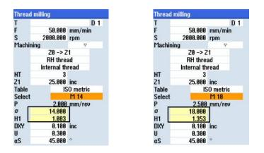
As soon as the line "Table ISO metric" is selected, the table is activated for the various threads.
