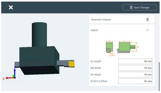
Figure 9-24 Defining a parametric adapter using a turning tool as an example
