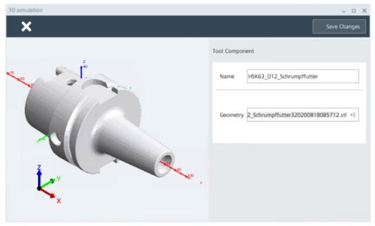
Figure 9-9 Tool component: example milling cutter holder
