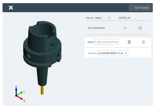
Figure 9-26 Tool holder from the library assigned to the tool
