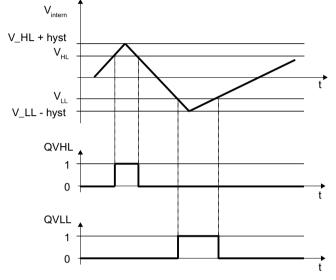
Figure A-2 Limit monitoring of the F\_INT\_P
