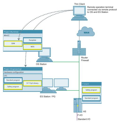
Figure C-1: Diagram of Engineering Station and Operator Station in projects with safety applications
