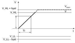
Figure A-1 Step response of the F\_INT\_P
