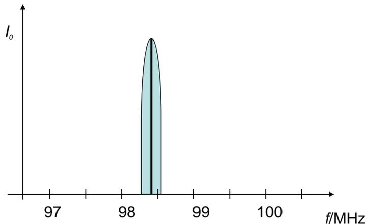
The example shown in the above figure illustrates the behavior of a VHF transmitter. Aside from the actual carrier frequency (approx. 98.4 MHz), a frequency band is used on both sides (blue). In this case, the band width is exaggerated; in reality 40 kHz are sufficient for an FM signal.
