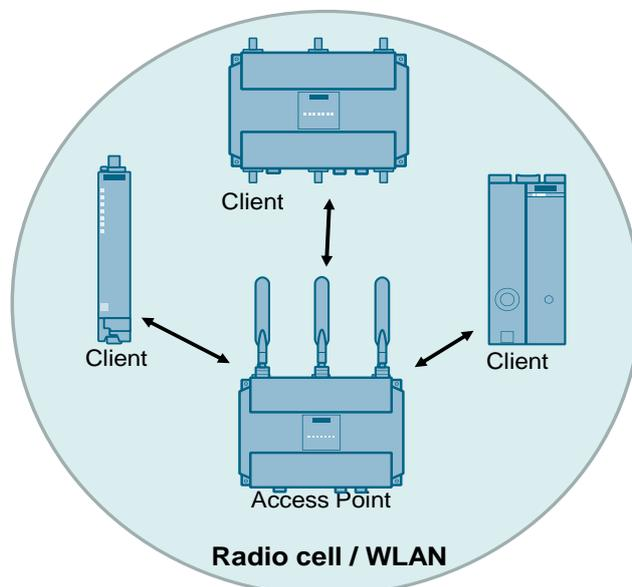
The above figure shows such a standalone network. It includes an access point which coordinates the data communication of the other bus nodes and via which the entire traffic is directed. The access point determines the “SSID” (“Service Set Identifier”) of the network, in other words, its “name”.
