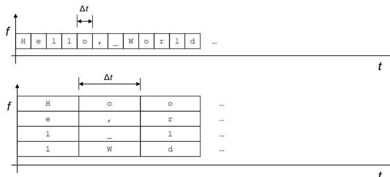
The top of the figure shows the “conventional” way of transmitting, the bottom shows the transmission with OFDM. The representation clearly shows how the transmission time  $\Delta t$  for an individual character is increased without compromising the overall data rate of the transmission.
