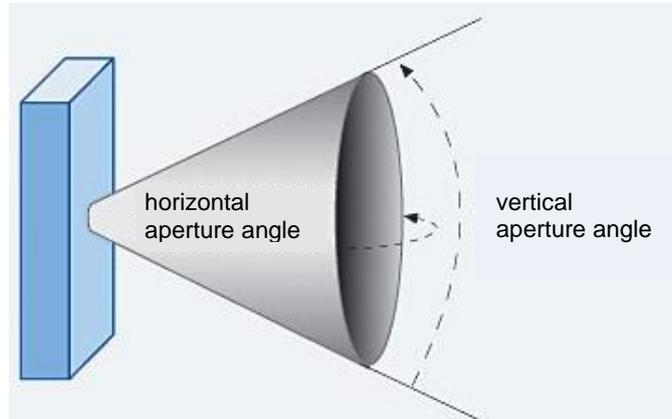
In the maximum field intensity direction the transmission range of a directional antenna is typically ten times as large as the range of an omnidirectional antenna.
