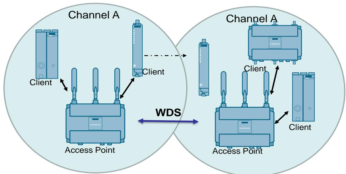
The above figure illustrates the principle of operation, compare also Figure 4-4. Several nodes connected via WLAN (clients) are located within the radio field covered by the access points (red circles above). Additionally, the access points maintain a further radio connection between each other.
