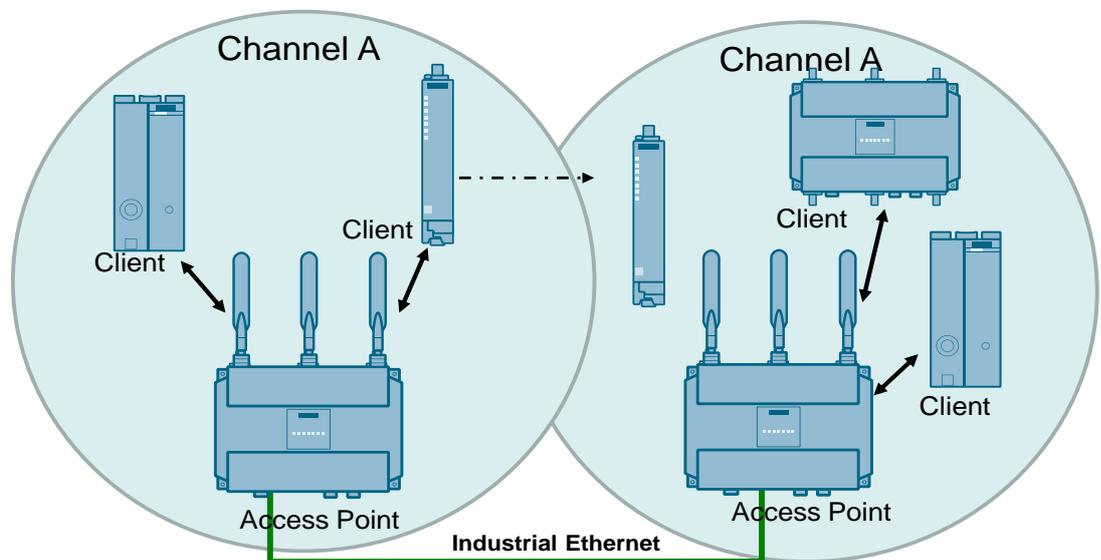
A number of access points are connected by a wire-bound Ethernet line. (Any other stationary nodes can also be connected to the Ethernet segment.) Several nodes connected via WLAN (clients) are located within the radio field covered by the access points (red circles above).
