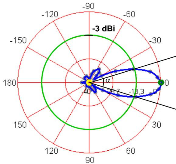
The horizontal and vertical aperture angles of an antenna usually differ depending on the geometry.
