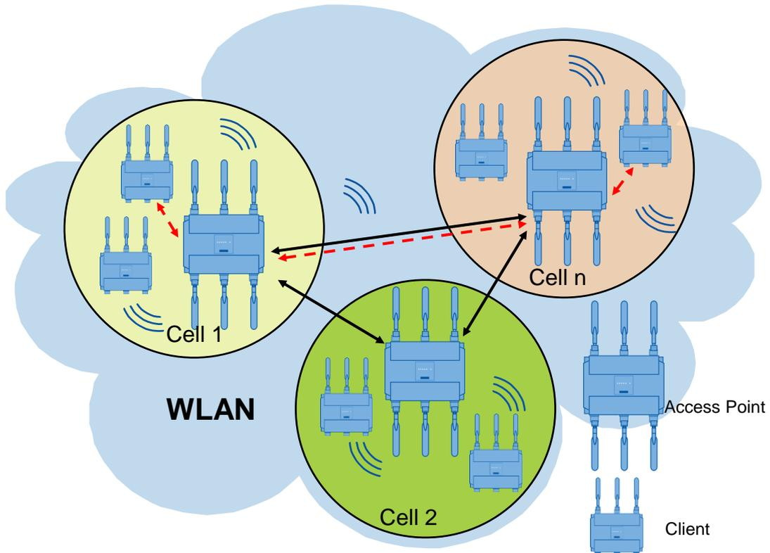
The figure shows the division of a WLAN into three radio cells (yellow, red, green) with a number of clients and one respective access point. The red arrows follow the communication path between a client of the yellow cell and a client of the red cell.
