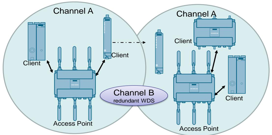
The access points do not communicate with each other on the primary frequency but on the second frequency with a second set of antennae.
