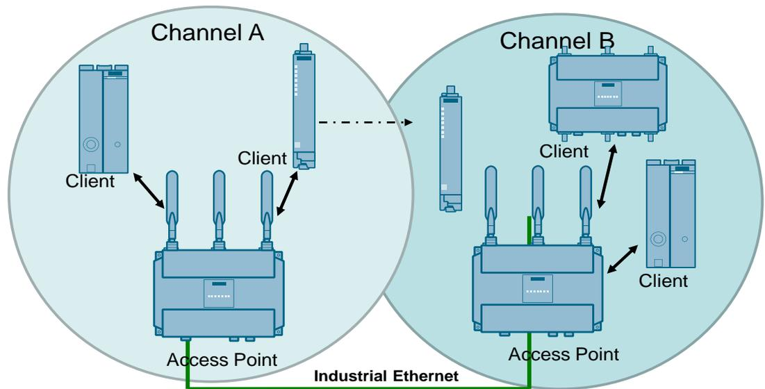
In this configuration, the individual access points form a backbone, and are connected to one another via a cable-based Ethernet cable. (Other stationary nodes do not have to be connected to the Ethernet segment.) Several nodes connected via WLAN (clients) are located within the radio field covered by the access points. The different frequencies on which the access points transmit are indicated by circles in different colors.
