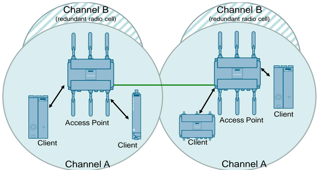
The access points establish an independent radio cell per radio interface, where primarily only one radio cell is used.
