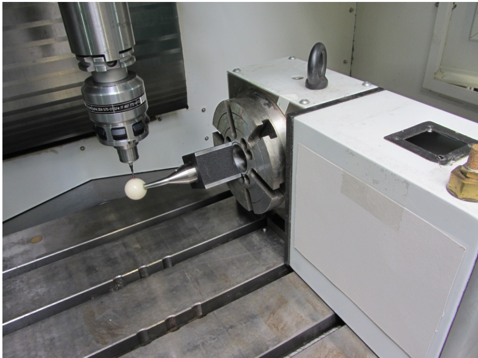
Fig. 2-2-1 Part indexing table as rotary axis with calibration sphere and workpiece probe
