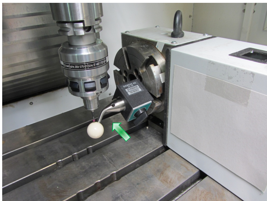
Fig. 4-13 Third CYCLE996 measurement at the part indexing table
