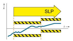
Figure 4-11 Safely-Limited Position
