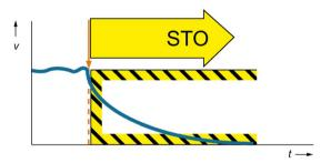
Figure 4-2 Safe Torque Off
