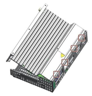
2. Insert the two plastic clips of top housing into the clip holes on heatsink.
