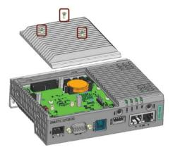
2. Use a screwdriver to poke the battery holder's tab, then remove the battery.
