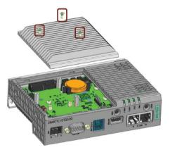
2. Drill holes with a corresponding diameter at the marking shown for mini PCle installation accessory. There are four reserved antenna-holes, two on each side of the top housing.
