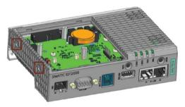
3. Insert the Mini PCle card in the Mini PCle interface and fix it with two M2 screws. For half size Mini PCle card, you need to move one standoff from A to B. Then install the half size Mini PCle card and fix it with a M2 screw.
