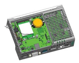
5. Get the cable of mini PCIe installation accessory out of the housing through the hole drilled.
