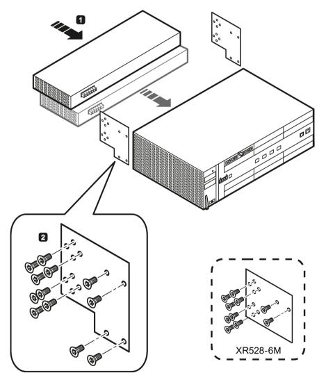
Figure 5-5 Rear panel mounting of the SCALANCE XR552-12M. SCALANCE XR528-6M is used analogously.
