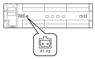
Figure 6-11 Position of the signaling contact on a SCALANCE XR552-12M. SCALANCE XR528-6M is analogous.
