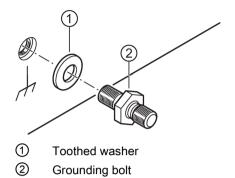
To fit the grounding bolt for a SCALANCE XR552-12M and SCALANCE XR528-6M, follow the steps below:
