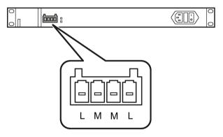
Figure 6-5 Position of the socket X2 on the PS598-1 power supply unit
