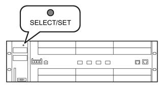
Figure 4-2 SELECT/SET button on the SCALANCE XR552-12M SCALANCE XR528-6M is analogous.
