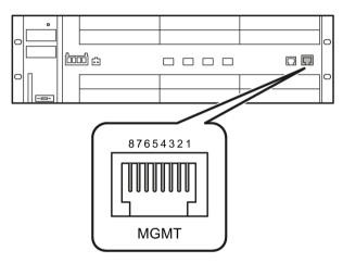
Figure 6-15 Position of the out-of-band interface on a SCALANCE XR552-12M. SCALANCE XR528-6M is analogous.
