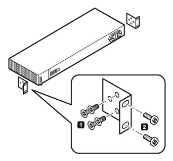
Figure 5-4 19" rack mounting of the power supply unit
