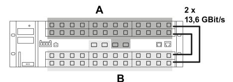
Figure 6-16 Block architecture of the SCALANCE XR552-12M
