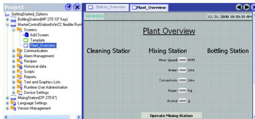
The shift manager uses the station overview screen to obtain information about essential operational data of the MixingStation: the fill levels of the reservoirs and the mixer speed.
