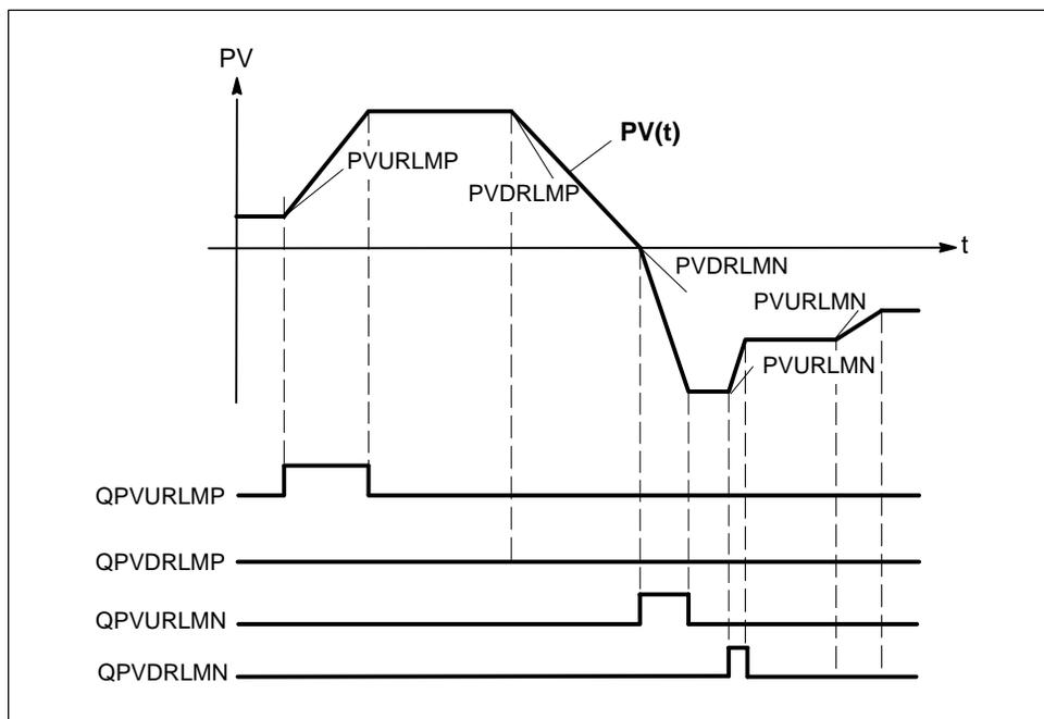
Figure 4-22 Monitoring the Rate of Change (Slope) of the Process Variable  $PV(t)$
