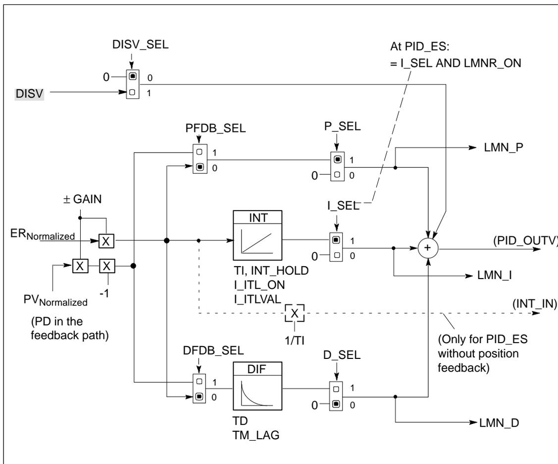
Figure 2-14 Signal Flow Diagram of the Control Function
