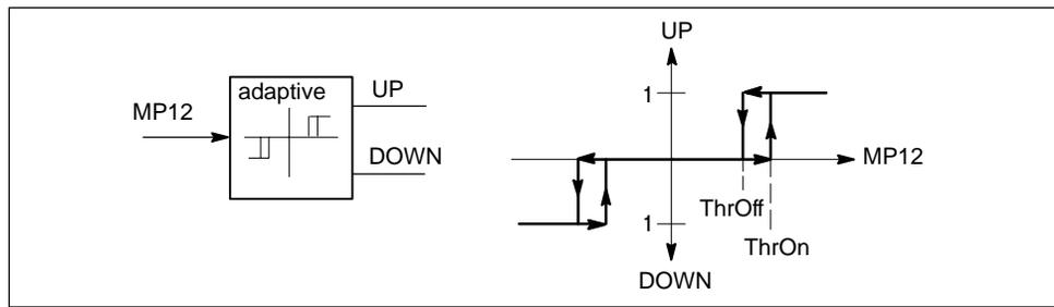
Figure 6-11 Functions of the Three-Step Element THREE\_ST
