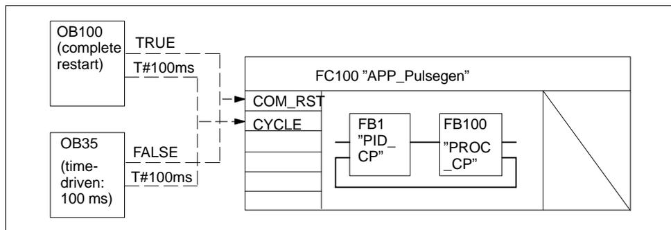
Figure 7-27 Blocks for Example6 Interconnection and Calling
