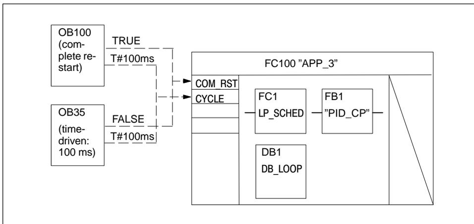
Figure 7-17 Blocks for Example3 Interconnection and Calling
