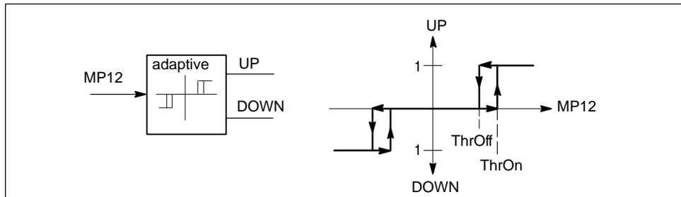
Figure 6-17 Functions of the Three-Step Element THREE\_ST
