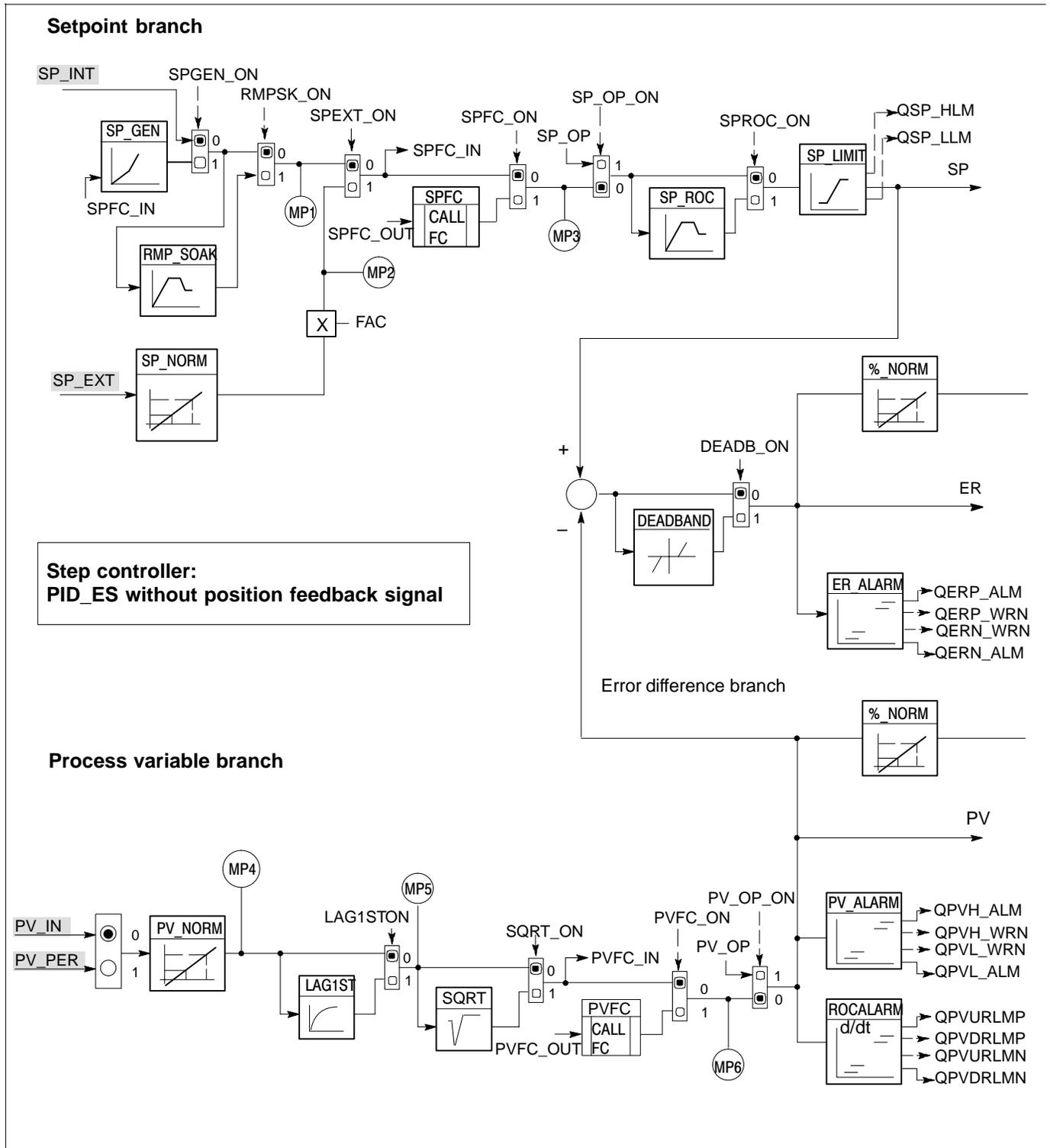
Figure 8-3 Block Diagram of the Step Controller: PID\_ES (without position feedback signal “LMNR\_ON = FALSE”)
