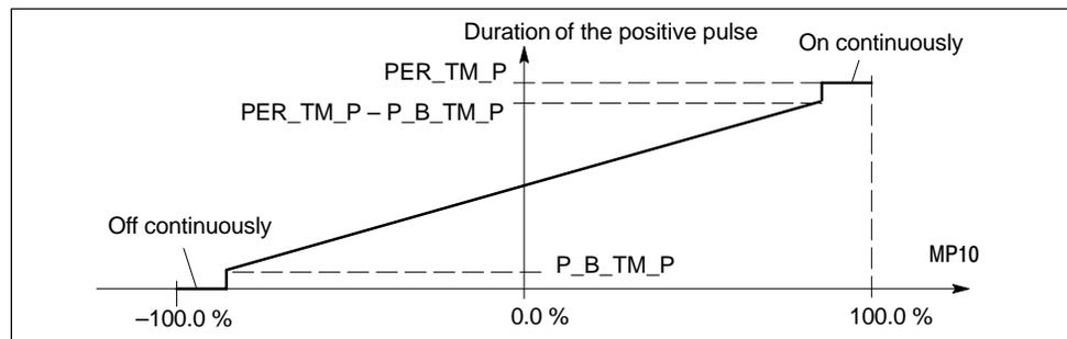
Figure 5-19 Two-Step Controller With Bipolar Range (-100% to 100%)
