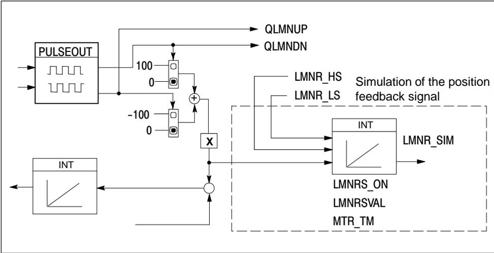
Figure 6-18 Simulation of the position feedback signal
