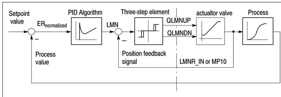
Figure 6-1 Step Controller With a Position Feedback Signal
