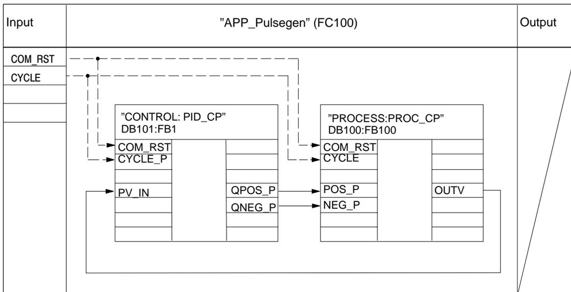
Figure 7-28 Interconnection and Calling the FC100 (APP\_Pulsegen)
