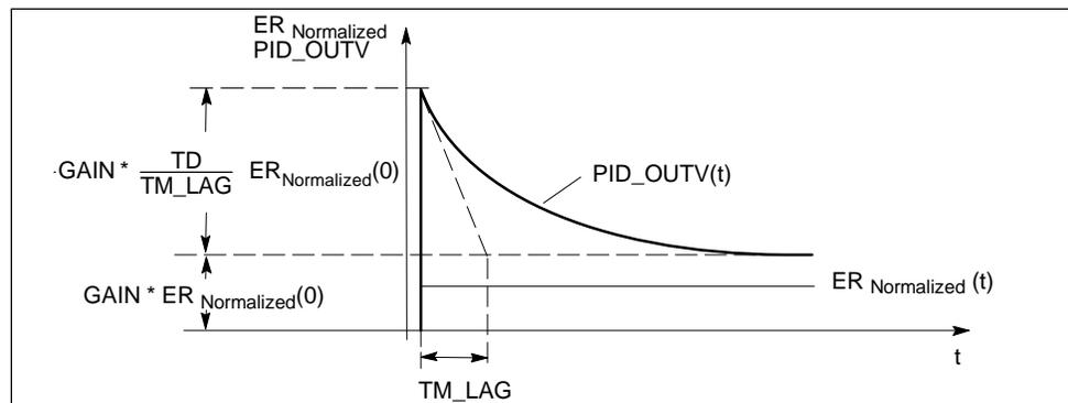
Figure 4-35 Step Response of the PD Controller
