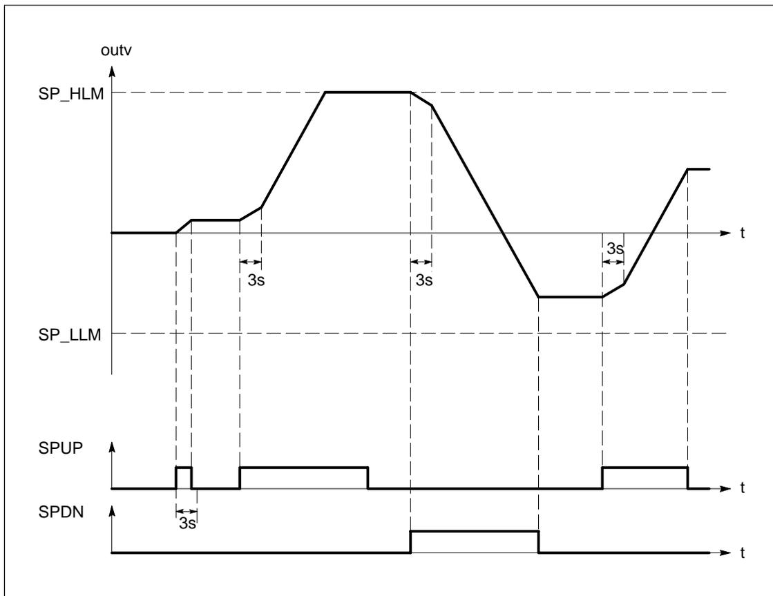
Figure 4-1 Changing outv as a function of the switches SPUP and SPDN
