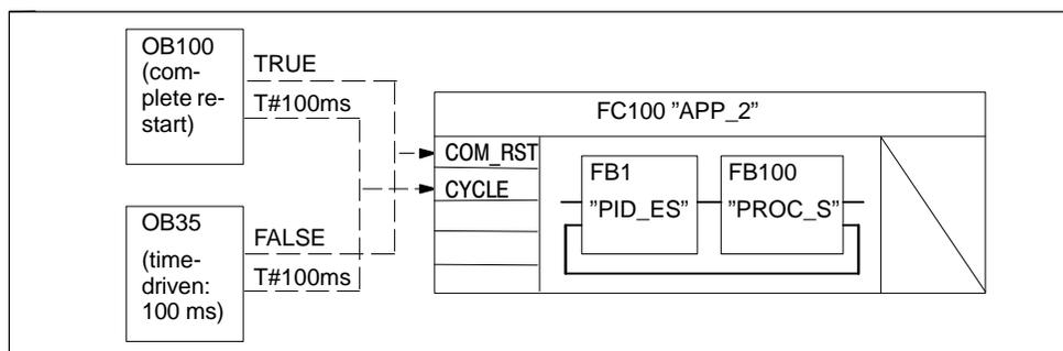
Figure 7-12 Blocks for Example2 Interconnection and Calling
