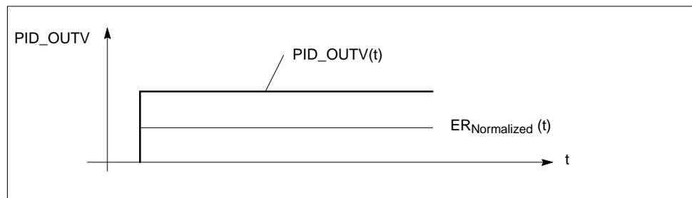
Figure 4-32 Step Response of the P Controller
