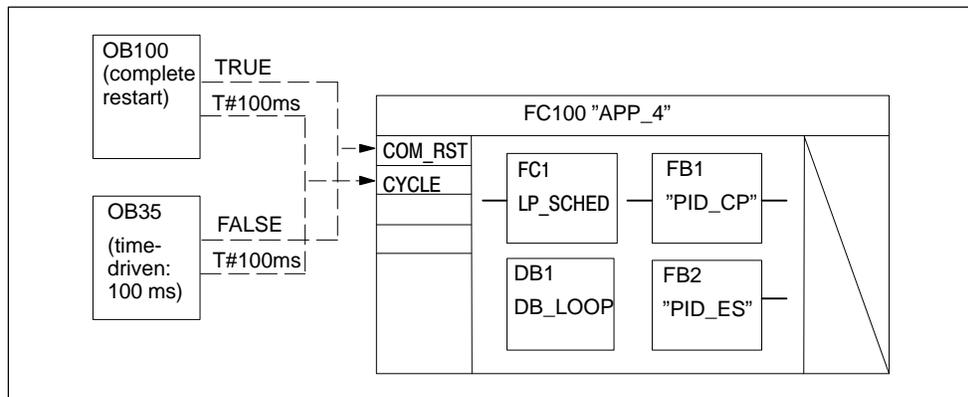
Figure 7-20 Blocks for Example4 Connection and Call
