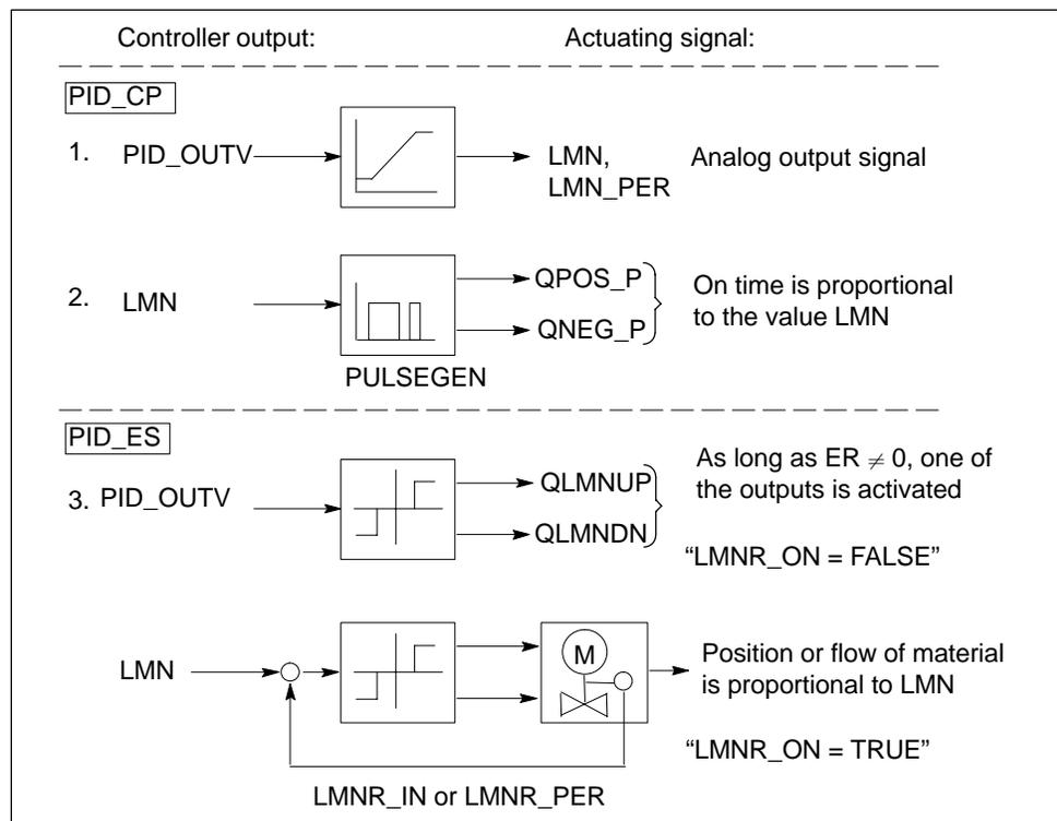
Figure 3-3 Actuating Outputs of Standard PID Control
