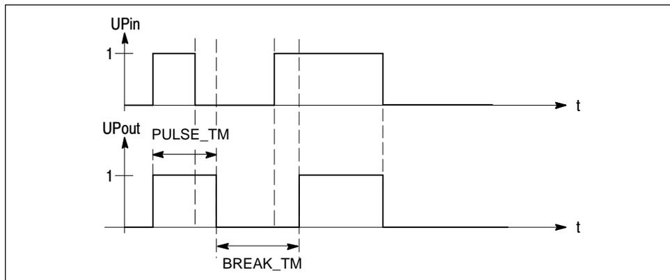
Figure 6-12 Functions of the Pulse Generator PULSEOUT
