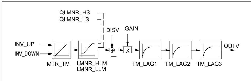
Figure 7-5 Structure and Parameters of the Process Block PROC\_S
