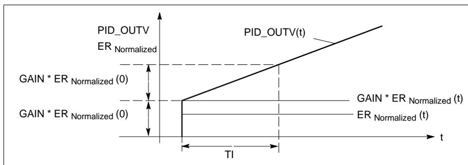
Figure 4-33 Step Response of the PI Controller
