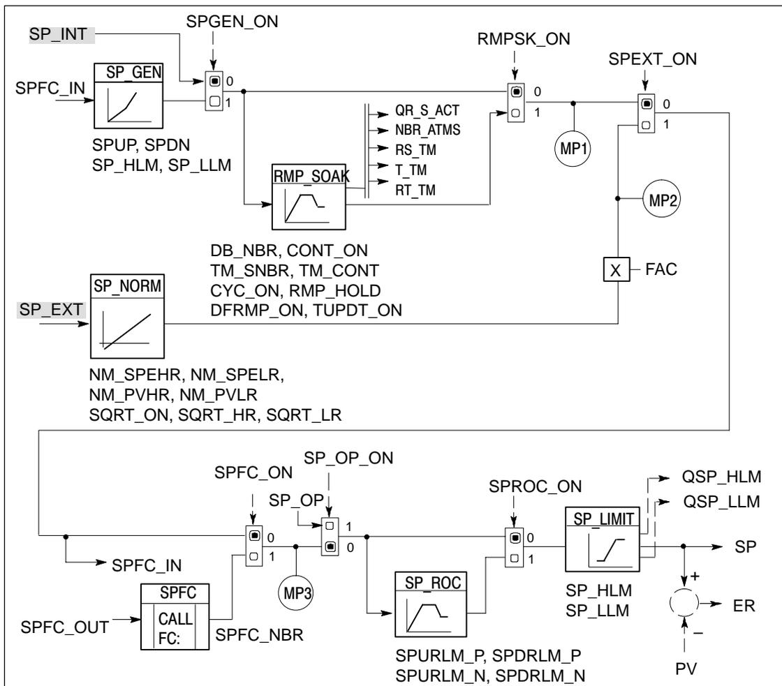
Figure 2-12 Signal Flow Diagram of Setpoint Processing
