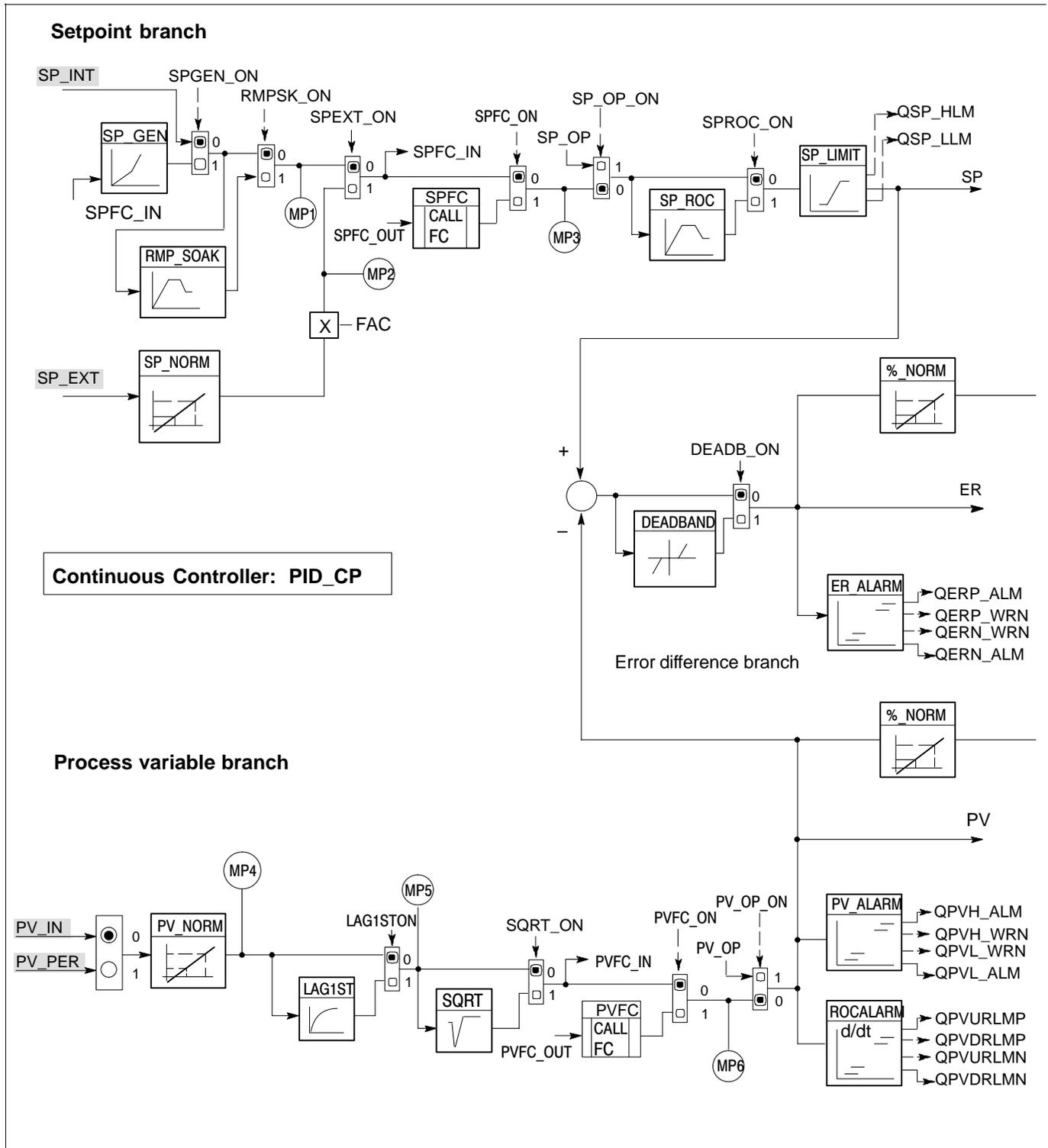
Figure 8-1 Block Diagram of the Continuous Controller: PID\_CP
