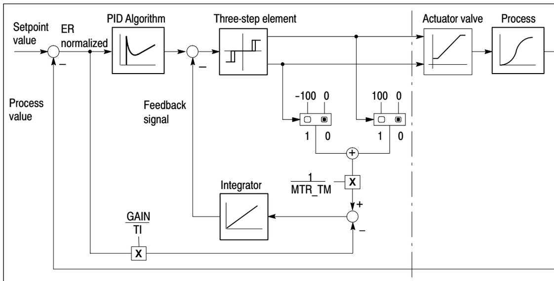
Figure 6-2 Step Controller Without Position Feedback Signal
