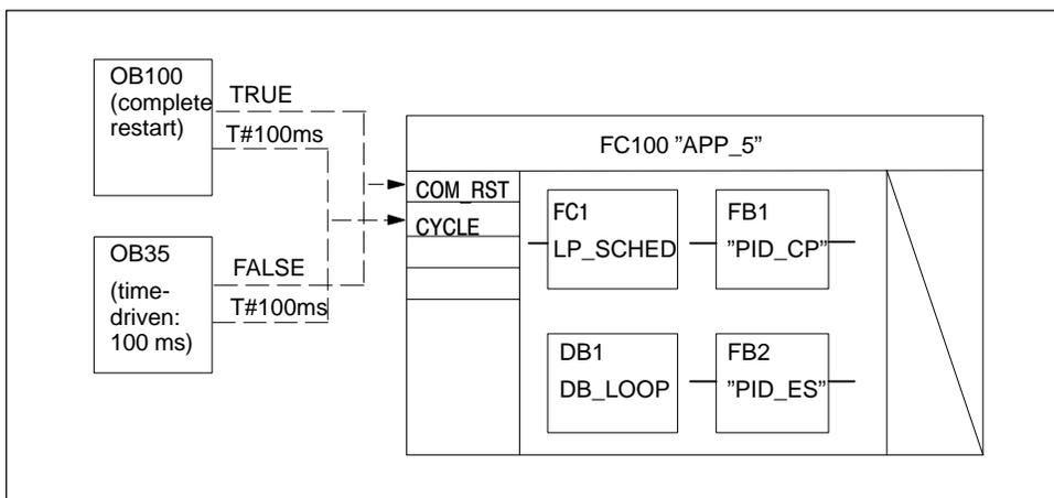
Figure 7-23 Blocks for Example5 Interconnection and Calling
