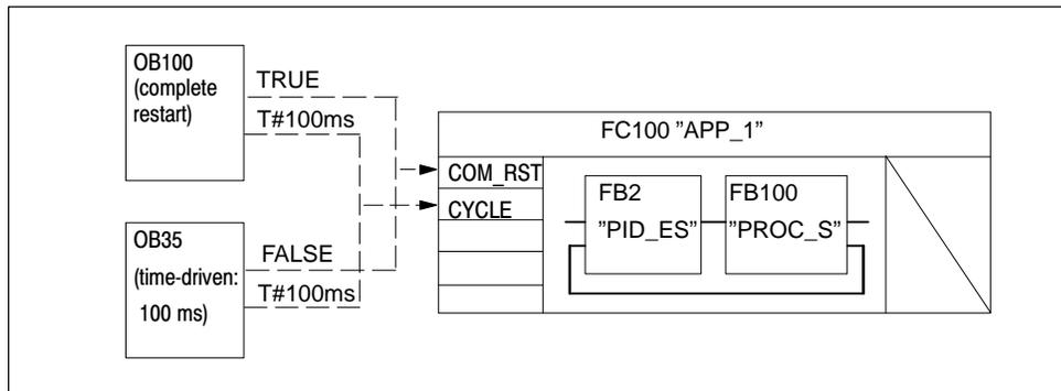
Figure 7-6 Blocks for Example 1: Interconnection and Calling
