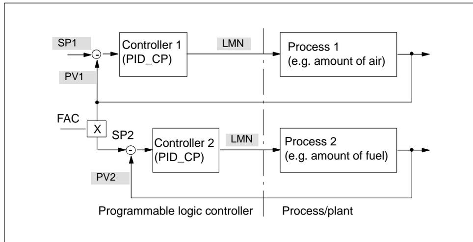
Figure 2-5 Ratio Control With Two Loops (Example3)
