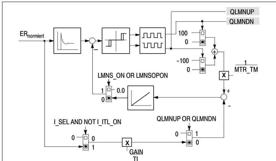
Figure 6-14 Step Controller Without Position Feedback Signal
