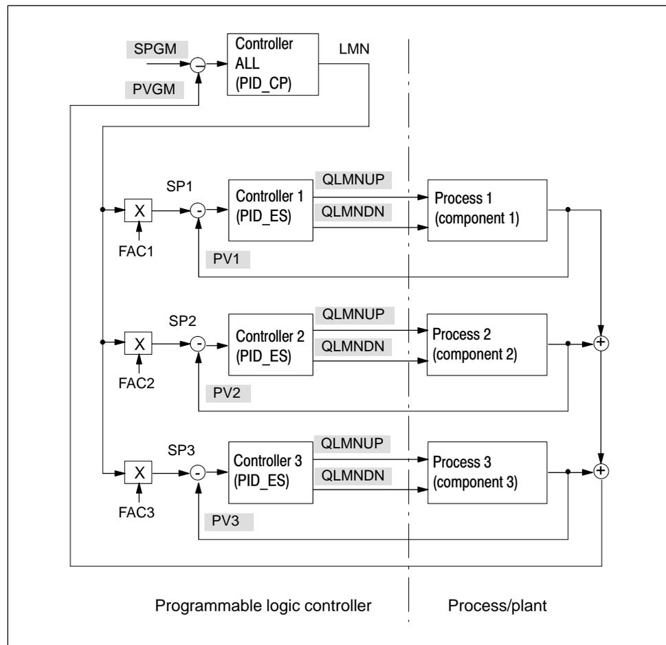
Figure 2-6 Blending control for three components (Example4)
