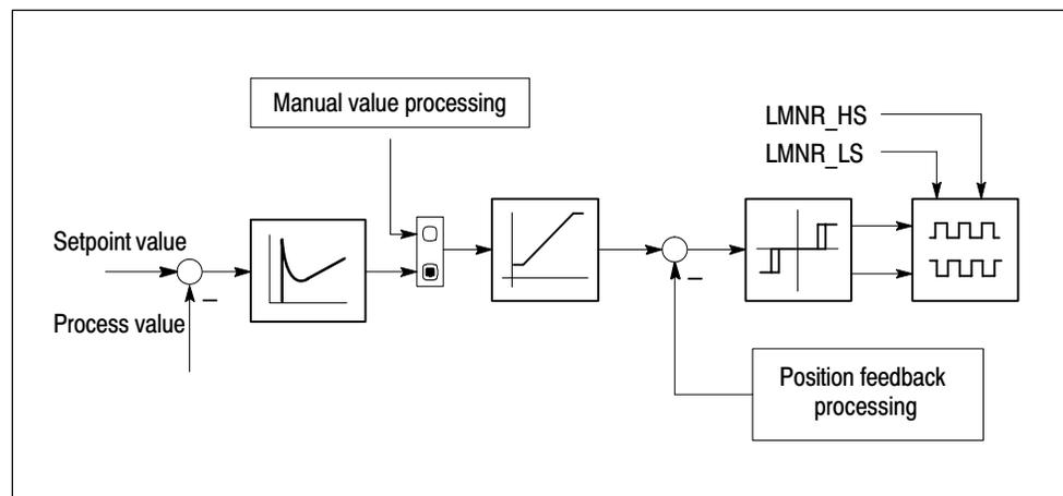
Figure 6-3 Step controller with position feedback signal
