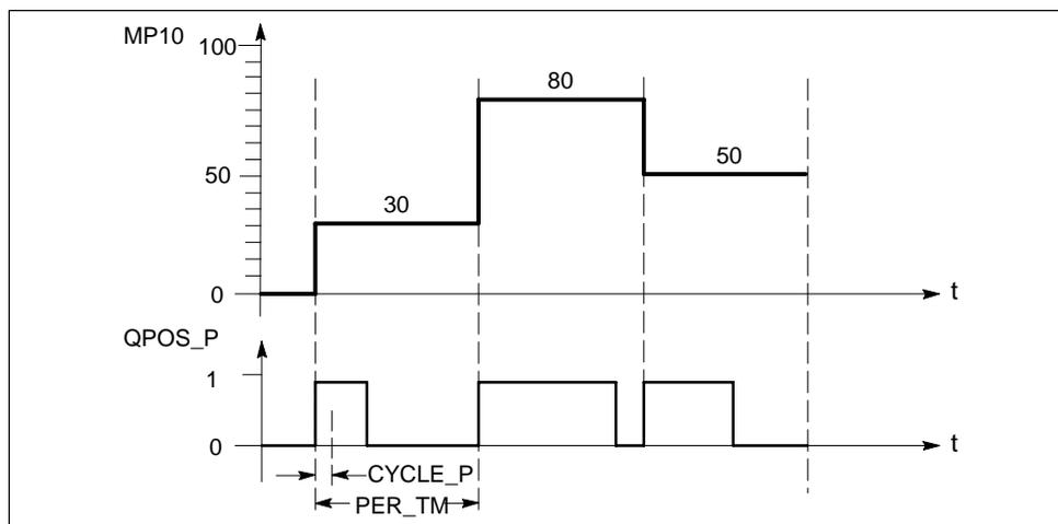
Figure 5-15 Pulse Duration Modulation
