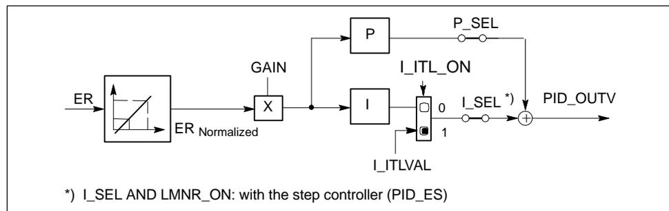
Figure 4-31 P Controller with Operating Point Setting
