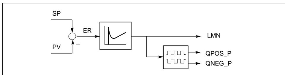
Figure 5-1 Block Diagram of the Controller with Continuous Actuating Signal ("Standard PID Control" Software Package)
