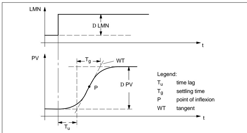
Figure 1 Step Response of a Self-Regulating Third Order Process
