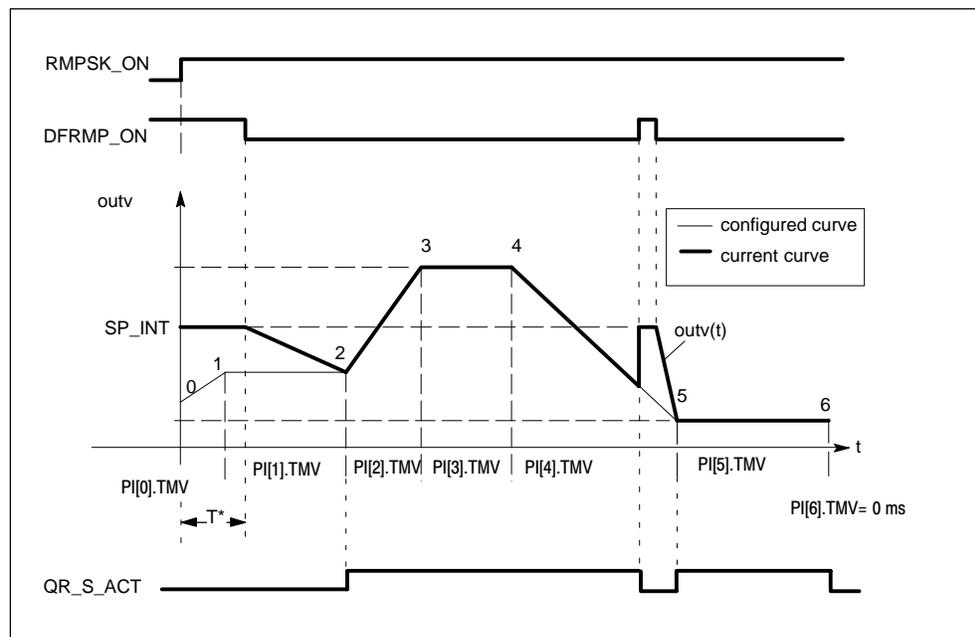
Figure 4-5 Influencing the Ramp Soak with the Default Signal `DFRMP_ON`
