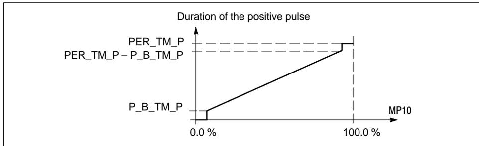
Figure 5-20 Two-Step Controller With a Monopolar Range (0% to 100%)
