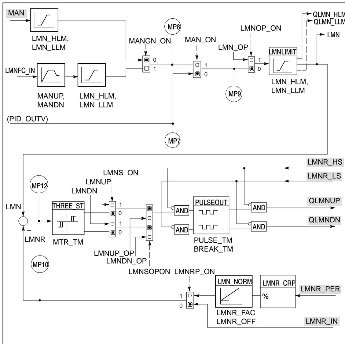
Figure 2-16 Signal Flow Diagram of Manipulated Variable Generation on the Step Controller with Position Feedback Signal (LMNR\_ON = TRUE)
