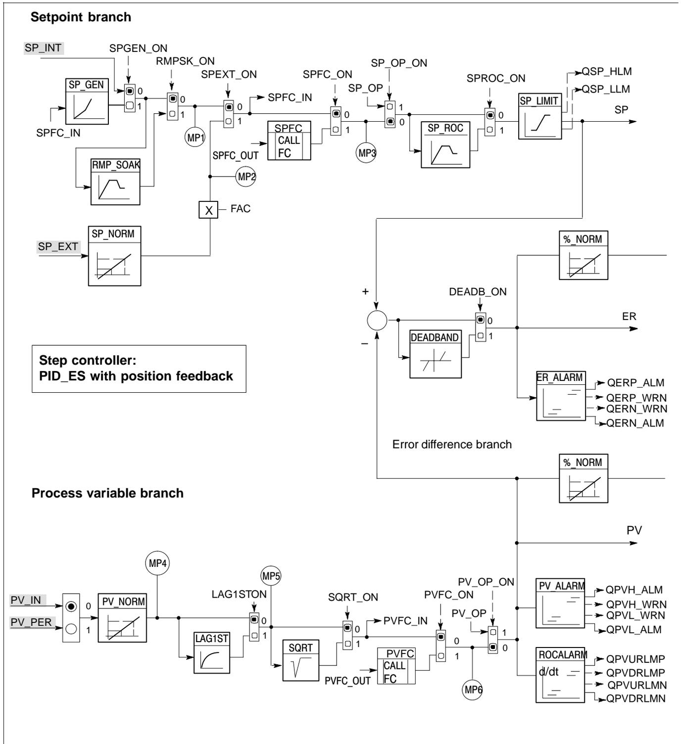
Figure 8-2 Block Diagram of the Step Controller: PID\_ES (with position feedback signal "LMNR = TRUE")
