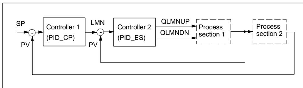
Figure 7-22 Two-Loop Cascade Control System (Example 5)
