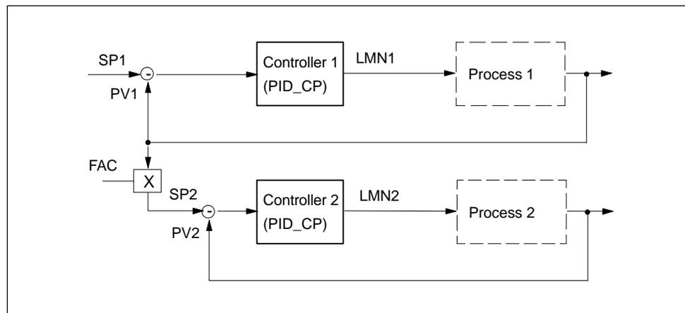
Figure 7-16 Ratio Control With Two Loops (Example 3)
