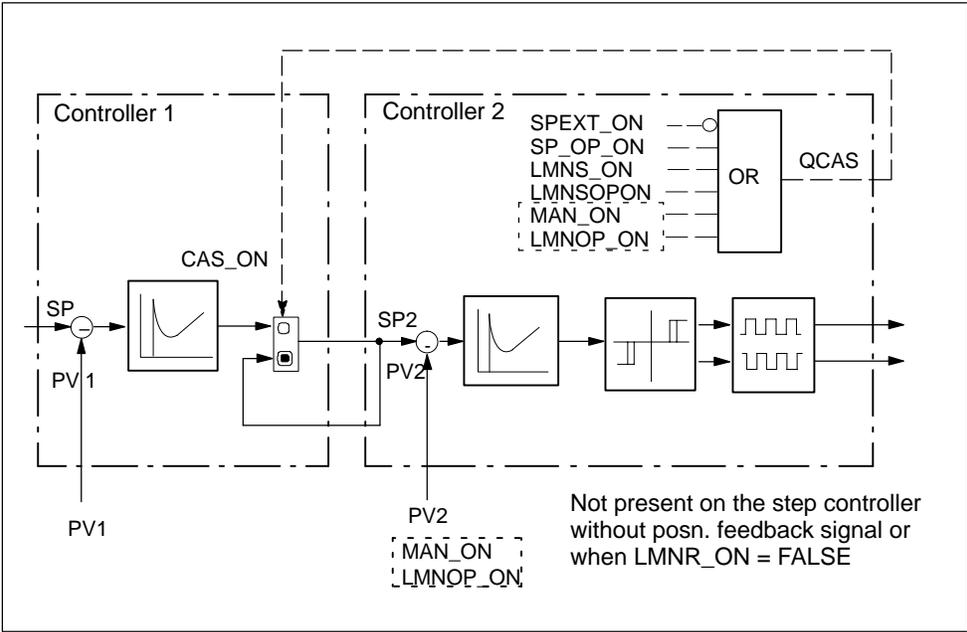
Figure 6-20 Two-Loop Cascade Control With a Step Controller
