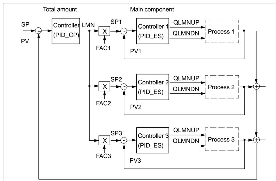
Figure 7-19 Blending Control for Three Components (Example4)
