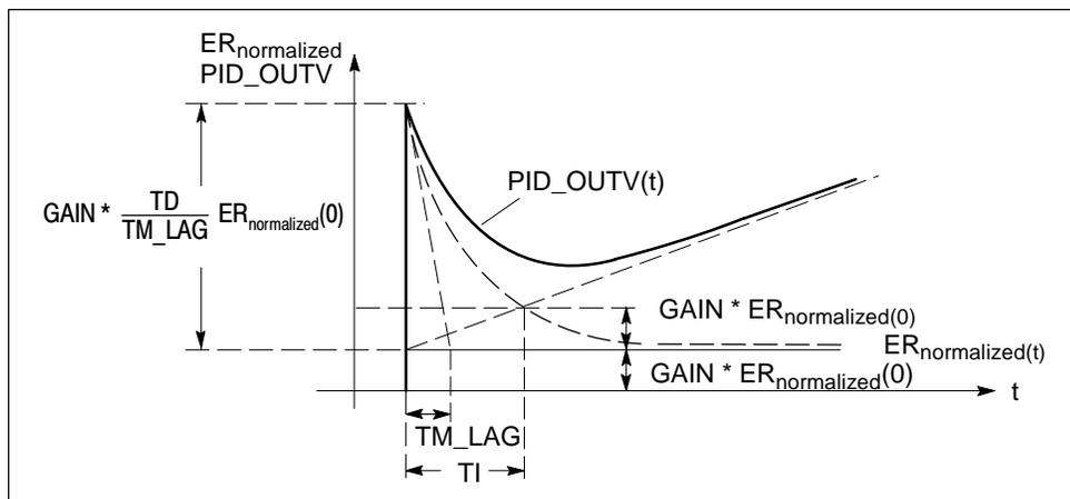
Figure 4-36 Step Response of the PID Controller
