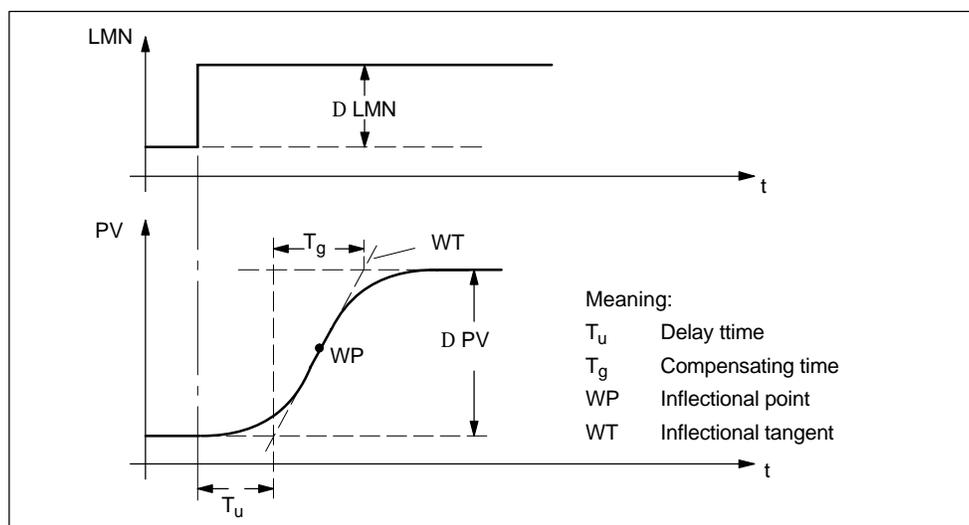
Figure 1-1 Transition function of a PT3 process
