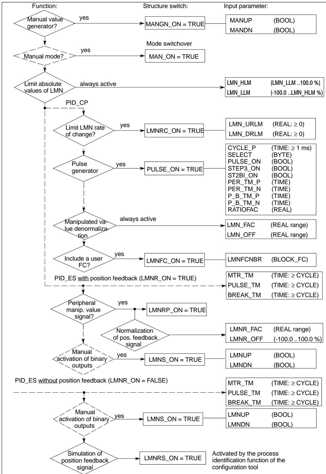
Figure 3-6 Configuration of the Manipulated Value (checklist point 8.)
