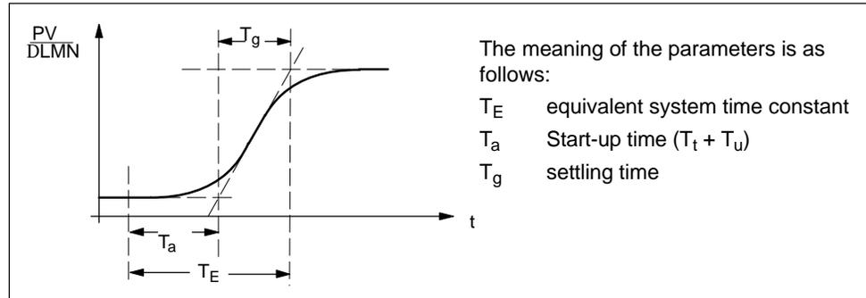
Figure 3-8 Determining the Equivalent System Time Constant  $T_E$
