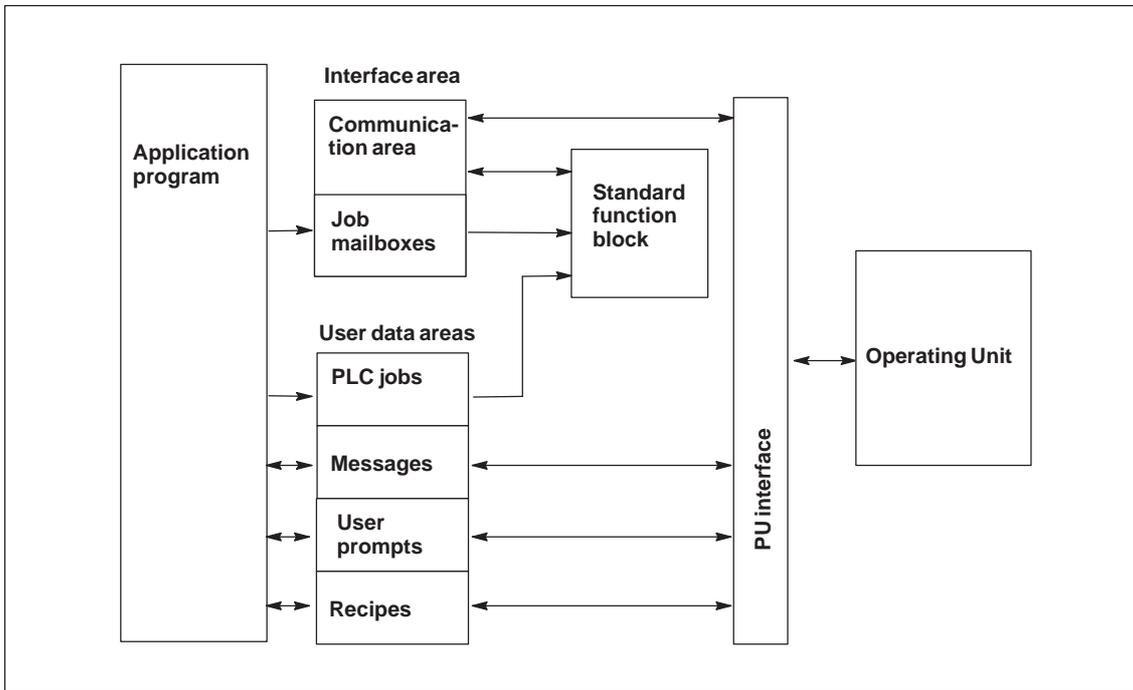
Figure 3-1 AS511 Communication Structure for Group 2 PLCs
