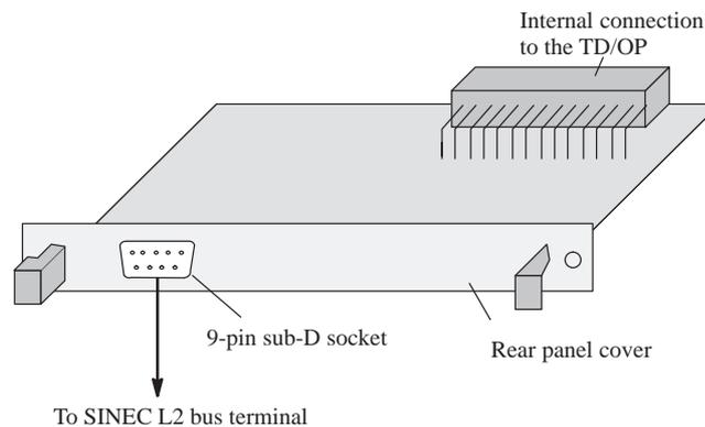
Figure C-5 Structure of the L2-DP interface module
