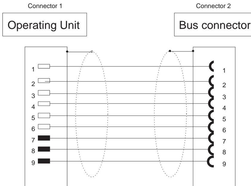
Cable: 9 x 0.14 mm<sup>2</sup>, shielded; length 5 cm
