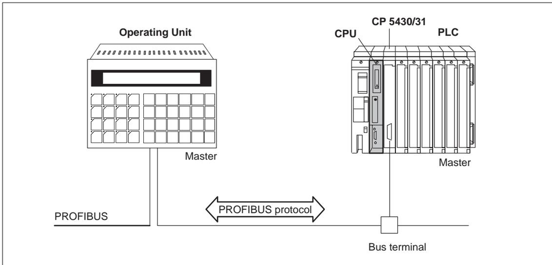
Figure 1-5 PROFIBUS Connection
