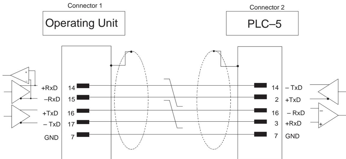
Cable 3 x 2 x 0.14 mm<sup>2</sup>; shielded; max. length 60 m
