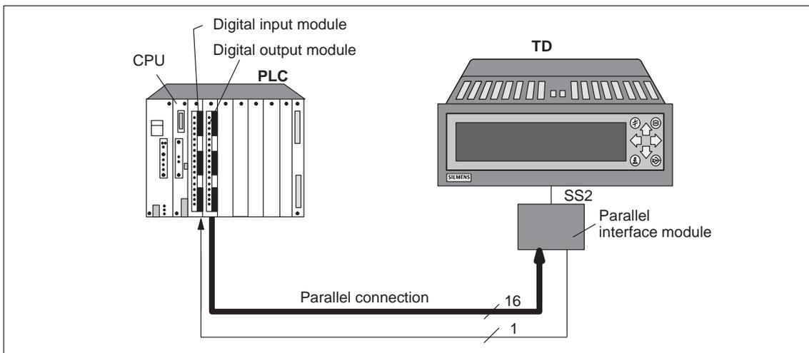
Figure 9-1 Parallel connection: standard configuration
