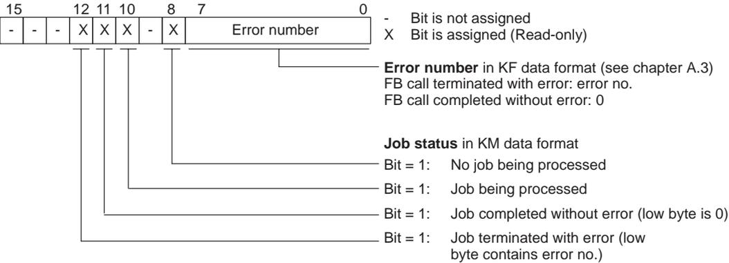
Figure 3-2 Contents of AKKU 1 after Invoking Standard FB
