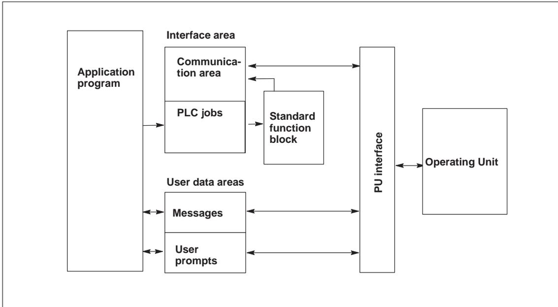
Figure 4-1 AS511 Communication Structure for Group 1 PLCs
