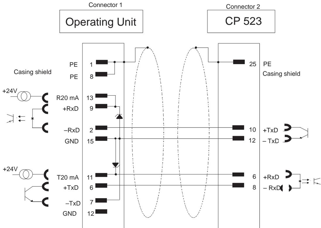
For TTY cables with special lengths > 10m, 2 Zener diodes (12 V) must be soldered in the 15-pin connector for the operating unit (TTY active):
