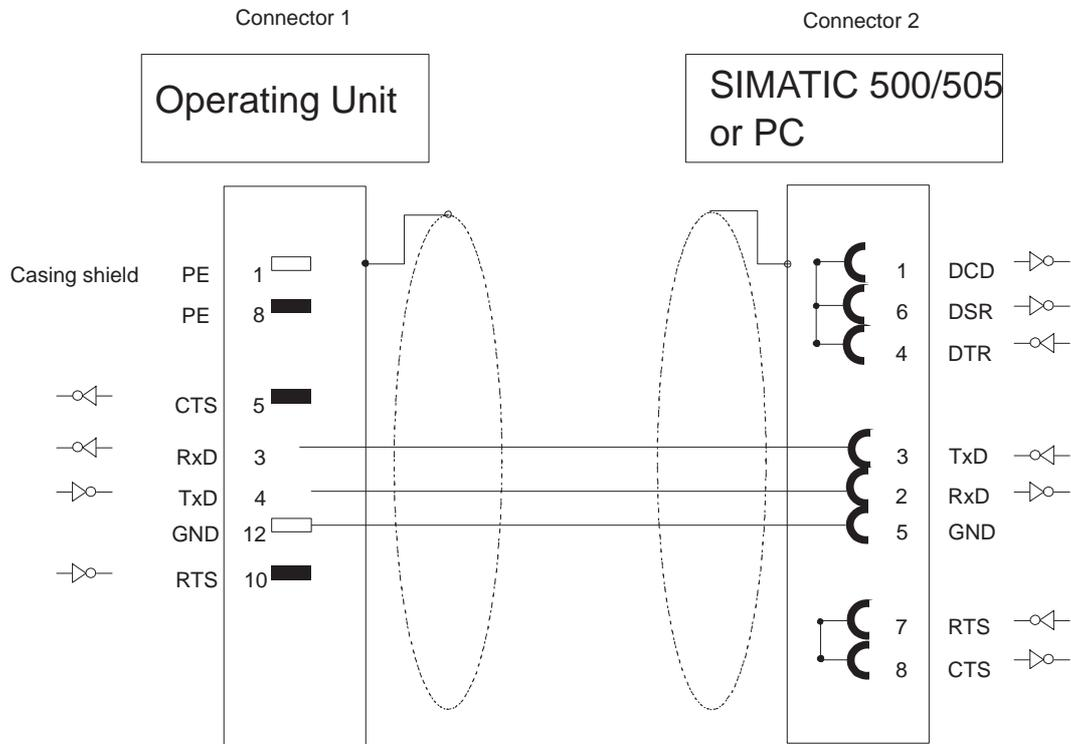
Shielding connected at both ends to casing with large contact area
