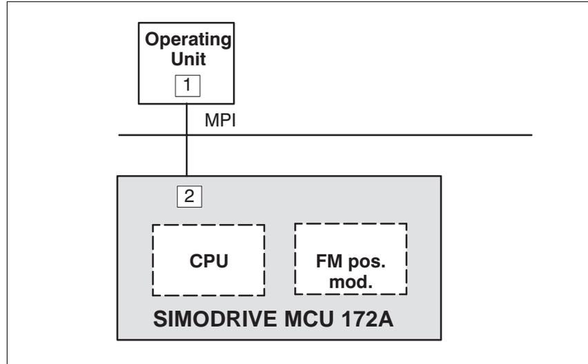
Figure 12-15 Network Configuration with SIMODRIVE MCU 172A and Operating Unit – MPI Profile
