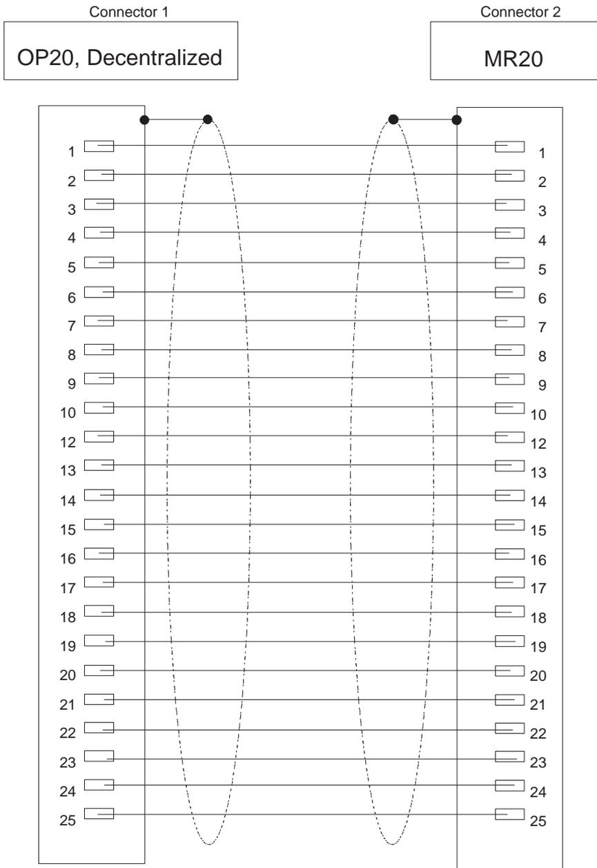
Cable 26 x 0.18 mm<sup>2</sup>; shielded; max. length 3.2 m
