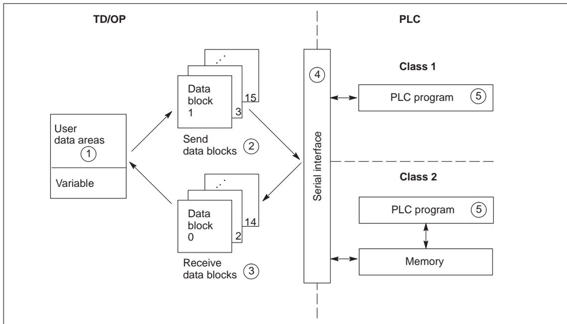
Figure 18-1 Communication structure for connecting other PLCs
