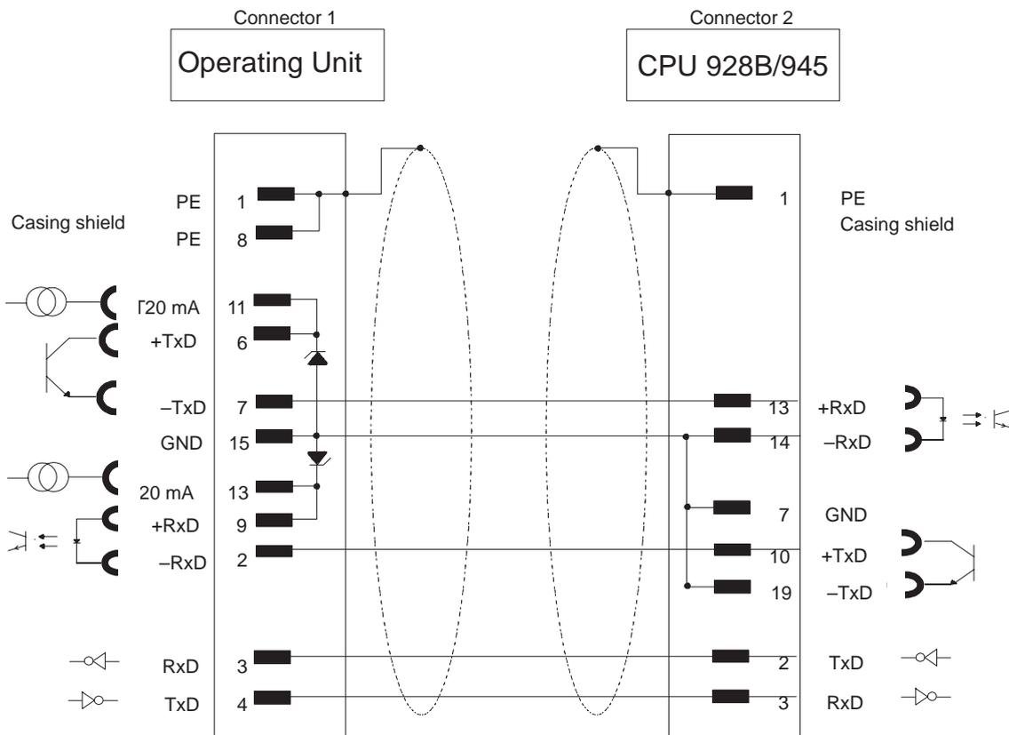
Cable: 5 x 0.14 mm<sup>2</sup>; shielded; max. length 1000 m
