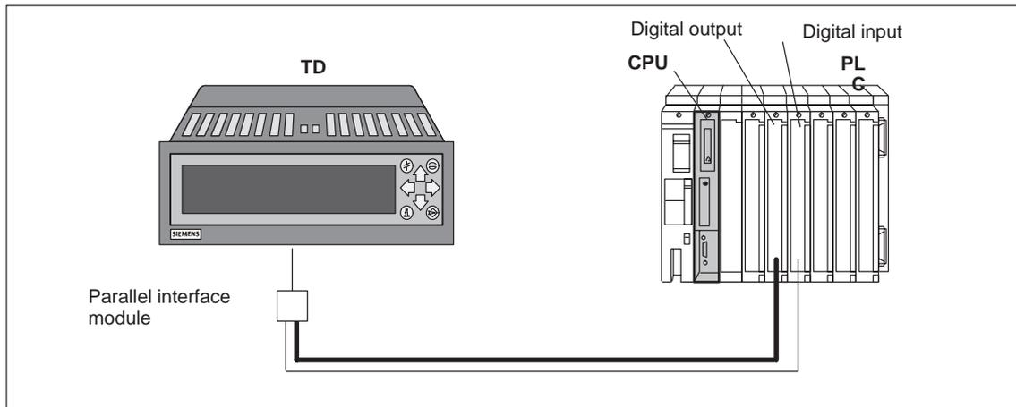
Figure 1-6 Parallel Connection
