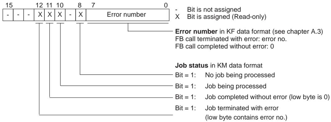
Figure 4-4 Contents of AKKU 1 after Invoking Standard FB
