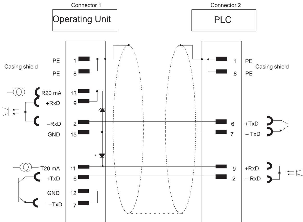
\* For TTY cables with special lengths > 10m, 2 Zener diodes (12 V) must be soldered in the 15-pin connector for the operating unit (TTY active):
