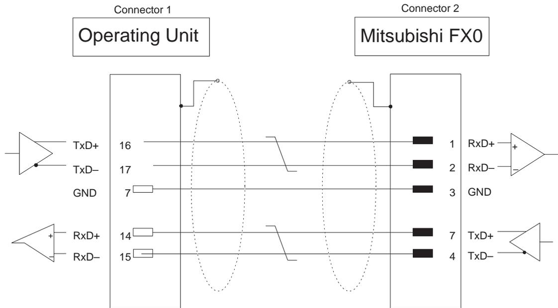
Cable: 3 x 2 x 0.14 mm<sup>2</sup>; max. length 500 m
