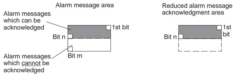
Figure 24-3 Reduced Acknowledgment Area
