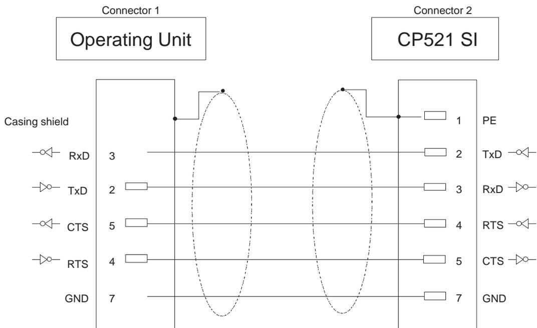
Cable: 5 x 0.14 mm<sup>2</sup>; shielded; max. length 15 m
