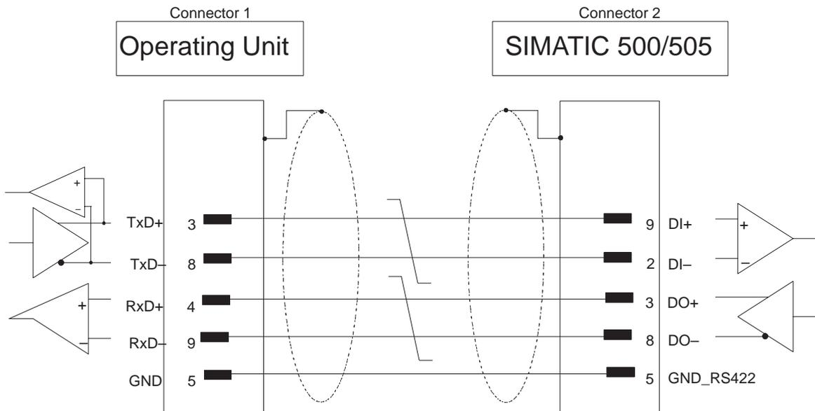
Shielding connected to casing with large contact area
