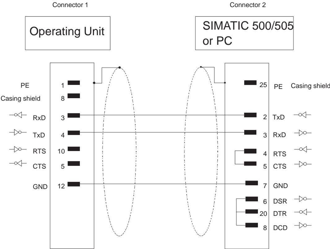
Shielding connected to casing with large contact area
