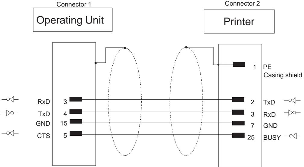
Cable: 5 x 0.14 mm<sup>2</sup>; shielded; max. length 15 m
