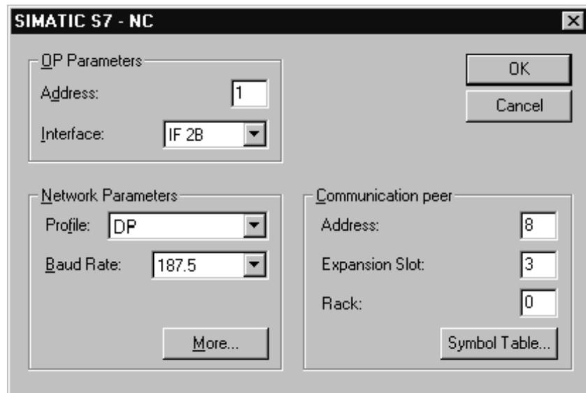
Figure 12-20 Configuring the FM-NC in ProTool – PROFIBUS-DP Profile
