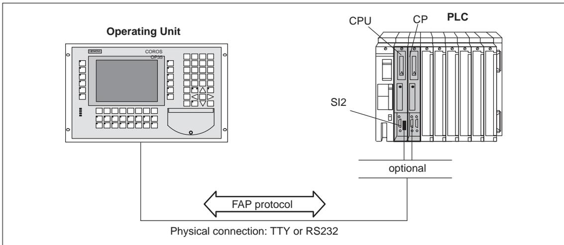
Figure 1-2 Connection using Free ASCII Protocol (FAP)
