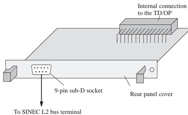
Figure C-4 Structure of the L2 interface module
