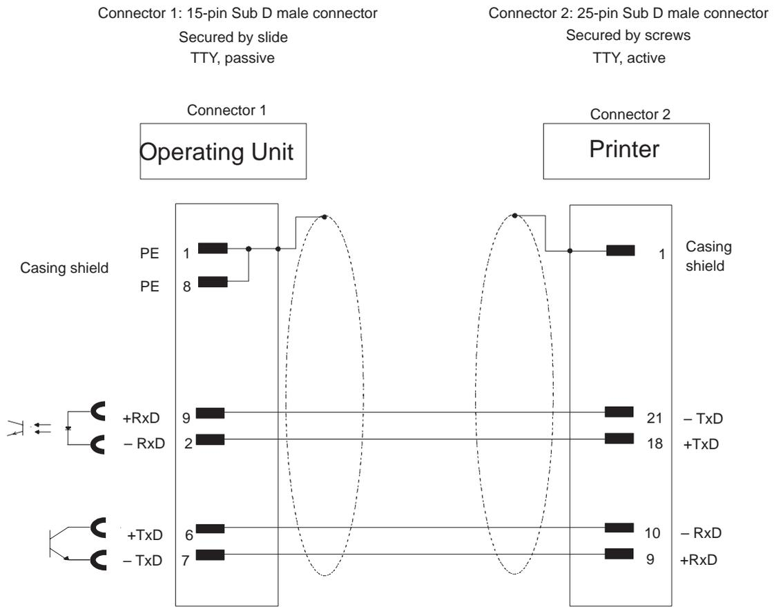
Cable: 5 x 0.14 mm<sup>2</sup>; shielded; max. length 1000 m
