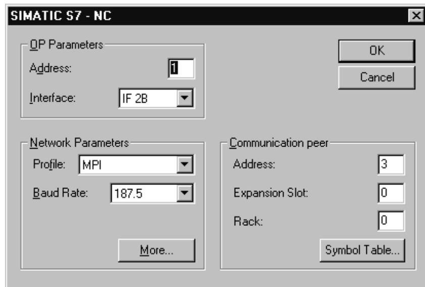
Figure 12-17 Configuring the FM-NC in ProTool – MPI Profile
