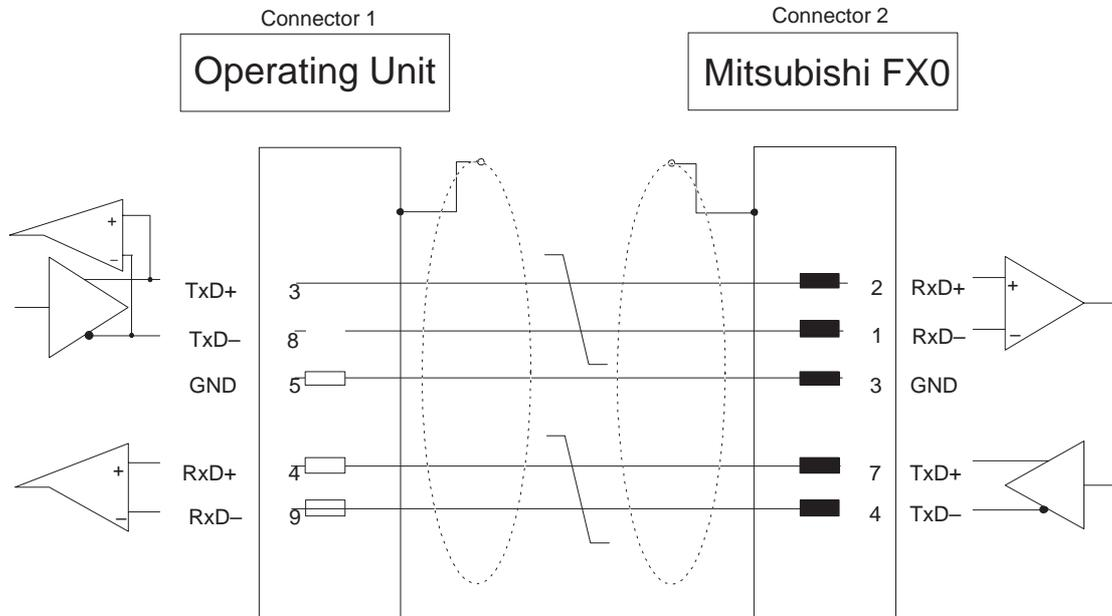
Cable: 3 x 2 x 0.14 mm<sup>2</sup>; shielded; max. length 500 m
