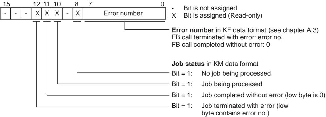
Figure 4-2 Contents of AKKU 1 after Invoking Standard FB
