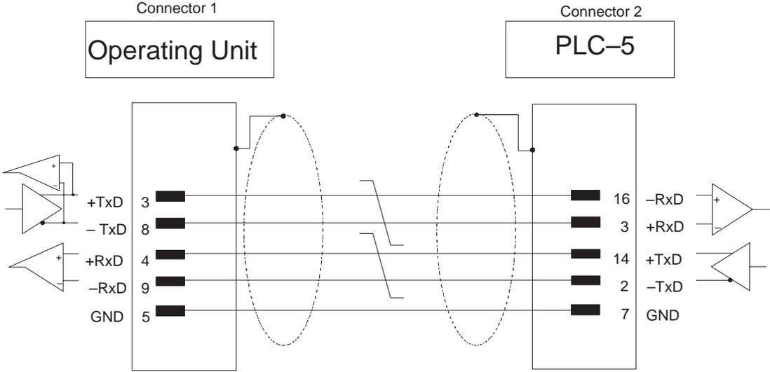
Cable 3 x 2 x 0.14 mm<sup>2</sup>; shielding contacts joined; max. length 60 m
