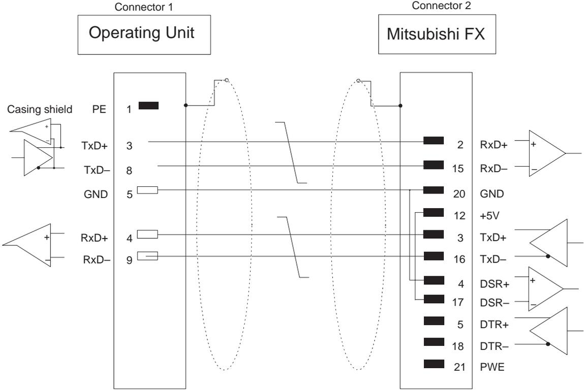
Cable: 3 x 2 x 0.14 mm<sup>2</sup>; max. length 500 m
