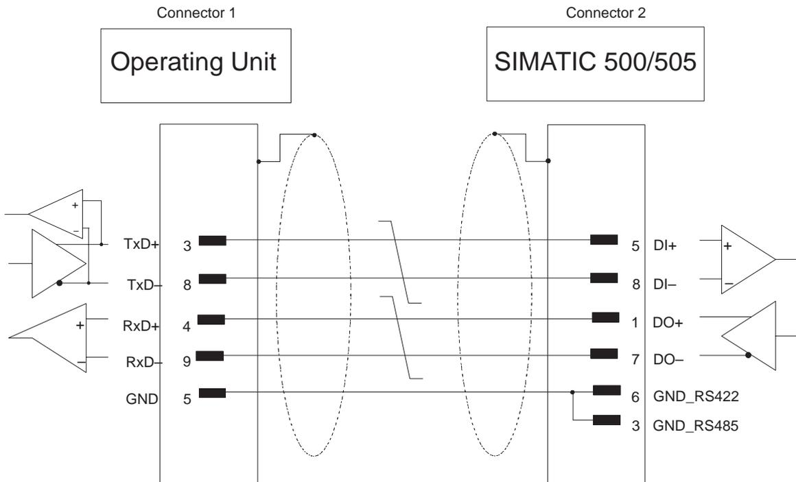
Shielding connected to casing with large contact area
