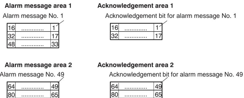
Figure 24-2 Acknowledgement Bit and Message Number Assignment
