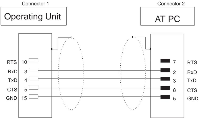
Cable: 5 x 0.14 mm<sup>2</sup>; shielded; max. length 32 cm
