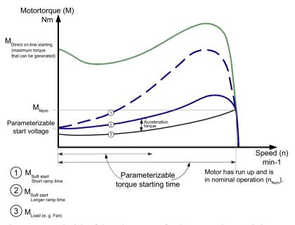
Figure 5-2 Principle of the voltage ramp for the torque characteristic
