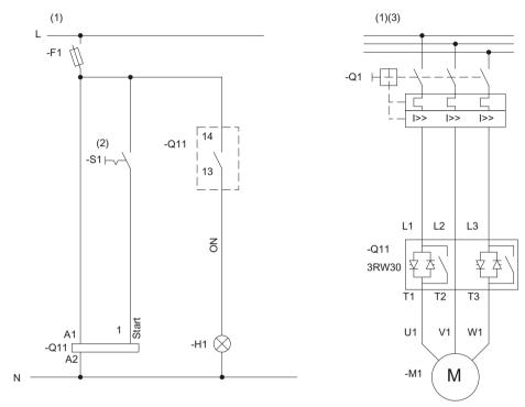
Figure 16-5 Wiring of the control and main circuits
