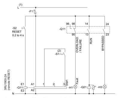
Figure 16-16 Wiring of the control circuit 3RW405 - 3RW407
