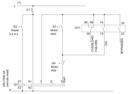
Figure 16-4 Wiring of the control circuit 3RW405 - 3RW407
