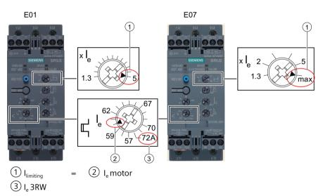
Figure 13-1 Optimized current limiting setting ranges
