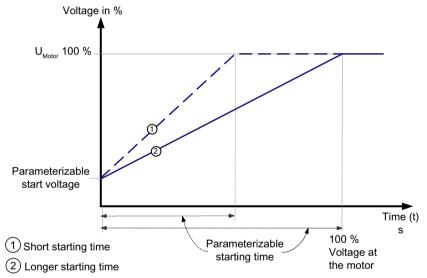
Figure 5-1 Principle of the voltage ramp
