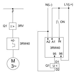
Figure 5-8 3RW40 wiring fault with 3RV
