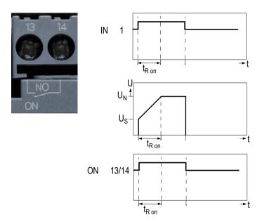
State diagram of the ON output contact
