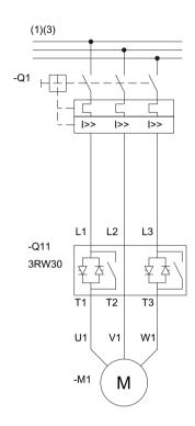
Figure 16-8 Wiring of the 3RW30 control and main circuits
