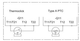
Figure 16-1 Optional thermistor motor protection evaluation
