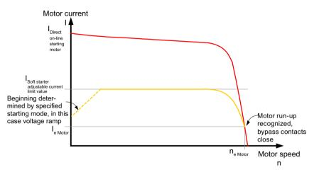
Figure 5-4 Current limiting with soft starter
