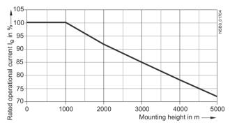
Figure 12-2 Reduction as a function of the installation altitude
