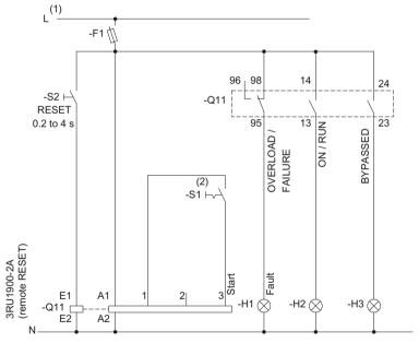
Figure 16-7 Wiring of the control circuit 3RW405 - 3RW407
