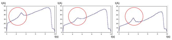
Figure 3-4 Current characteristic and occurrence of DC components in the three phases without "polarity balancing"
