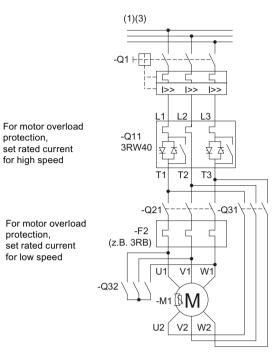
Figure 16-35 Wiring of the main circuit 3RW405 - 3RW407
