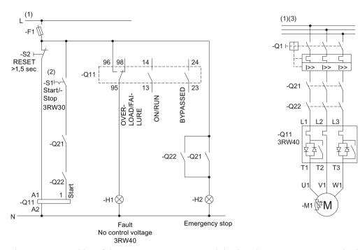
Figure 16-26 Wiring of the 3RW402 - 3RW404 control circuit and 3RW402 - 3RW407 main circuit (1) For permissible main and control voltage values (dependent on article number), refer to chapter Technical data (Page 133).
