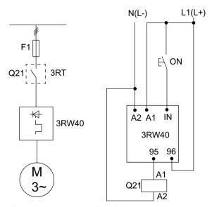
Figure 5-7 3RW40 wiring fault
