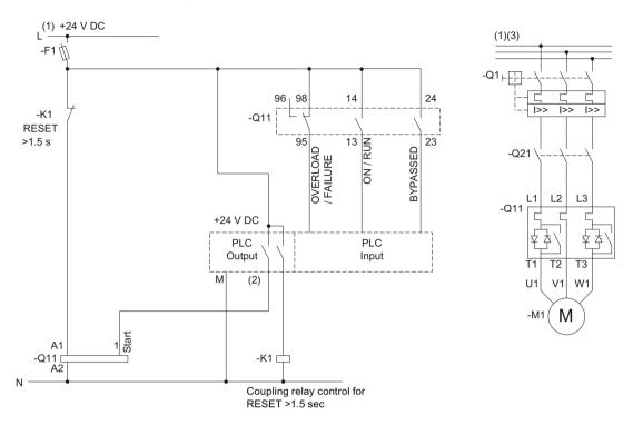
Figure 16-12 Emergency stop wiring of the 3RW402 - 3RW404 control circuit (with 24 V control voltage) and 3RW402 - 3RW407 main circuit
