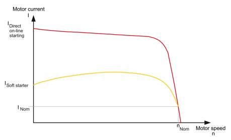
Figure 3-1 Reduced current characteristic of a three-phase induction motor during starting with a SIRIUS 3RW30 or 3RW40 soft starter
