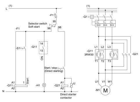
Figure 16-29 Wiring of the 3RW30 control and main circuits
