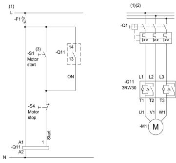
Figure 16-2 Wiring of the 3RW30 control and main circuits
