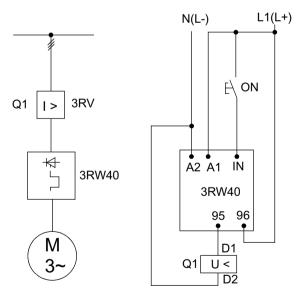
Figure 5-6 3RW40 wiring fault with 3RV
