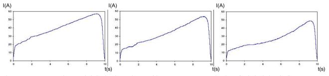
Figure 3-5 Current characteristic in the three phases without DC components thanks to "polarity balancing"
