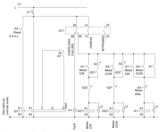
Figure 16-19 Wiring of the control circuit 3RW405 - 3RW407
