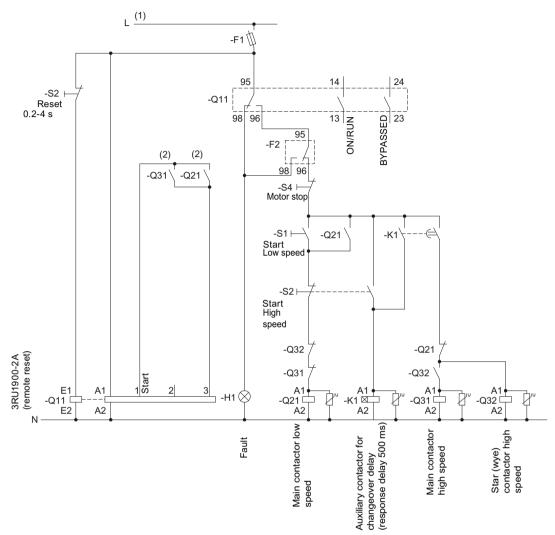
Figure 16-34 Wiring of the control circuit 3RW405 - 3RW407
