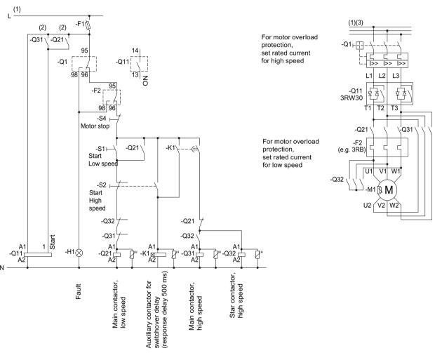
Figure 16-32 Wiring of the 3RW30 control and main circuits
