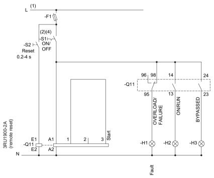
Figure 16-10 Wiring of the control circuit 3RW405 - 3RW407
