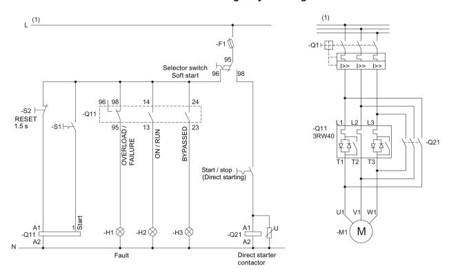
Figure 16-30 Wiring of the 3RW402 - 3RW404 control circuit and 3RW402 - 3RW407 main circuit
