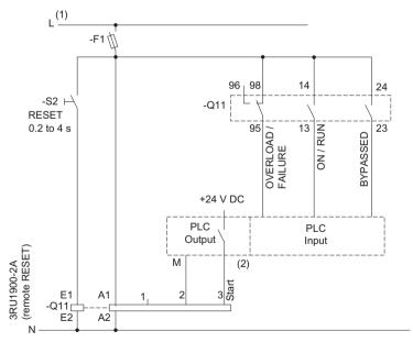
Figure 16-13 Wiring of the control circuit 3RW405 - 3RW407
