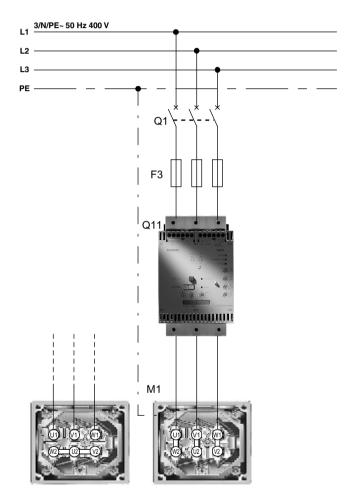
Figure 9-3 Block diagram of a feeder with semiconductor fuses
