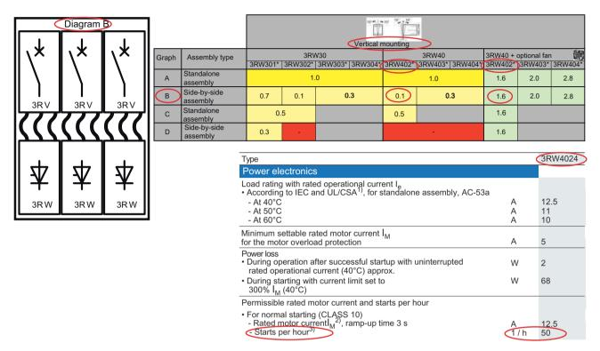
Assembly of a 3RV2021 motor starter protector and connection of a 3RW4024 soft starter with cables and vertical mounting for CLASS 10 starting:
