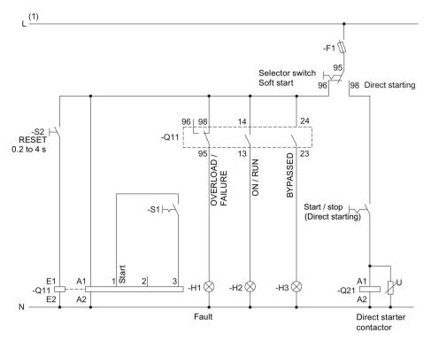
Figure 16-31 Wiring of the control circuit 3RW405 - 3RW407
