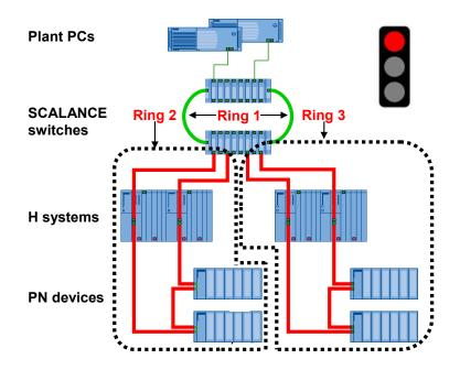
Rings 2 and 3 are not located within the open ring between PN device and H system (compare chapter 4.1.3, where the SCALANCE switch is located within an open ring which is not counted as a ring).
