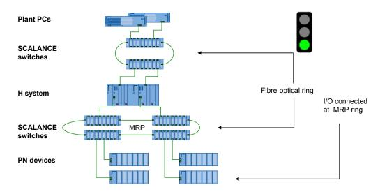
The SCALANCE switches above the H system for connecting the plant PCs are used for bridging the distance and can use the MRP (not mandatory). There are several possibilities of a redundancy mechanism for bridging occurring failures, such as
