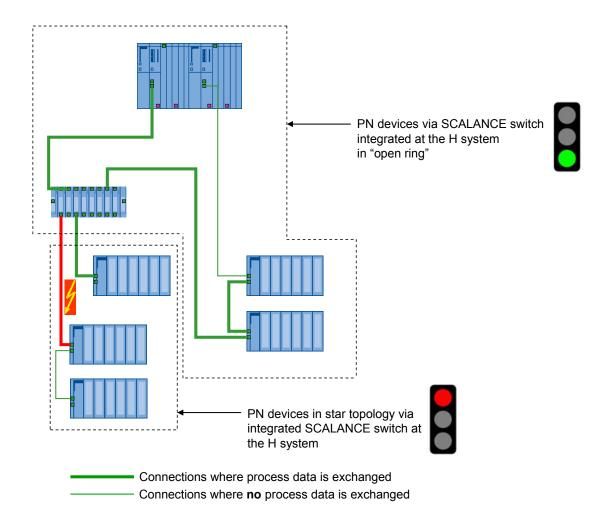
In this example, the central PN switch connected in star topology fails. The availability of the lower PN switch could be increased by connecting it directly to the SCALANCE switch instead of the central PN device.
