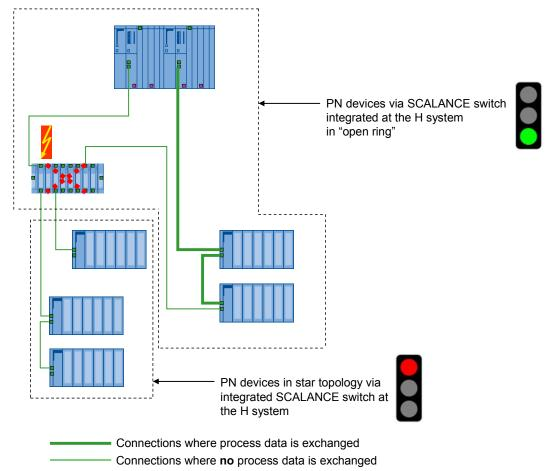
A failure of a SCALANCE switch causes the PN devices connected in star topology to fail. The PN devices in the open ring remain available.
