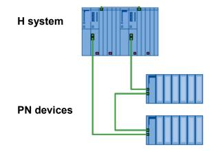
The IO devices need to support the system redundancy; otherwise, they can be operated in the same network, however only one of both H-CPUs can be assigned (unilateral periphery).
