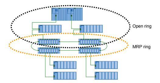
All ring nodes must be compatible with the media redundancy protocol (MRP). The hardware components that can be used as media redundancy manager (MRM) are available in the following entry:
