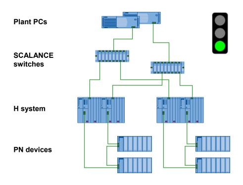
For this configuration, the CP 443-1 can be replaced by the PN interface.
