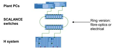
The application of two SCALANCE switches enables achieving media redundancy over larger distances (e.g. up to 26 km with SCALANCE X-200).
