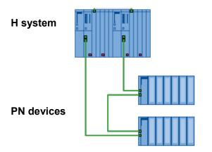
For the open ring, the PN devices are set up as single channel. After the H system has gone from single operation to redundant system state, both H-CPUs process the same program in synchronism. However, process data are only exchanged with the PN device by one H-CPU.
