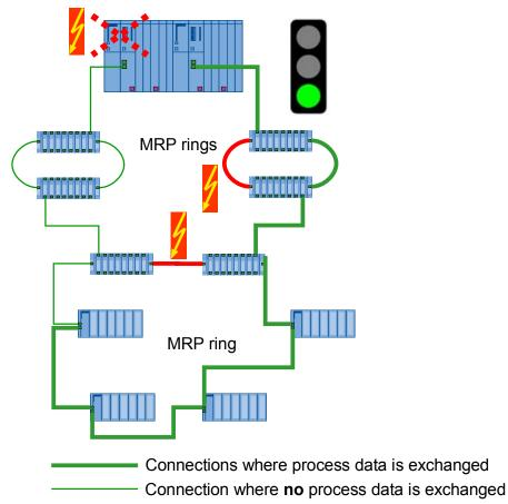
In addition to the failure of the master CPU, the following can fail in the line in which process data is exchanged:
