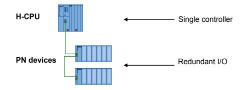
When an H-CPU (IO controller) fails, the entire process periphery is no longer available due to missing system redundancy.
