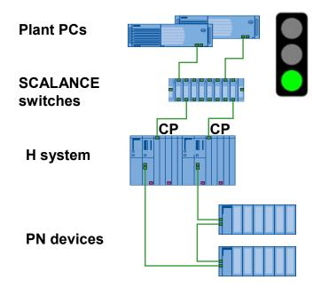
The SCALANCE switch is not integrated in any ring. If the CPs 443-1 are replaced by the PN interface, a ring is produced (next picture). For this configuration, the CP 443-1 can be replaced by the PN interface.
