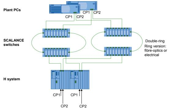
The application of two SCALANCE switches enables achieving media redundancy over larger distances (e.g. up to 26 km with SCALANCE X-200).
