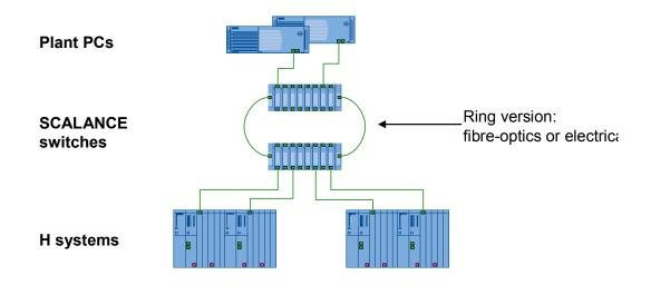
The application of two SCALANCE switches enables achieving media redundancy over larger distances (e.g. up to 26 km with SCALANCE X-200).
