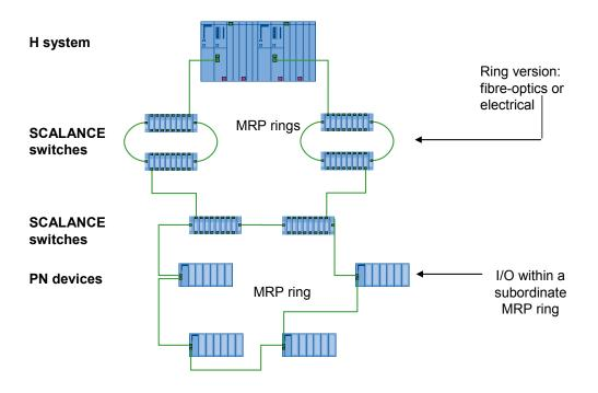
Each H-CPU is preceded by an MPR ring via the PROFINET interface (two SCALANCE switches per H-CPU). It only serves for bridging the distance to the sub-ordinate MRP ring.
