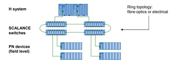
In this configuration, the system as well as the media redundancy can become effective:
