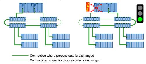
The process is maintained bumpless by means of the reserve CPU. The media redundancy is not required for the failure scenario.
