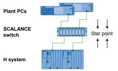
Additionally, a second SCALANCE switch (as in chapter 4.2.1 and 4.2.2) can be integrated. The higher procurement costs are countered by the option of reaching media redundancy across larger distances (e.g. up to 26 km with SCALANCE X-200).
