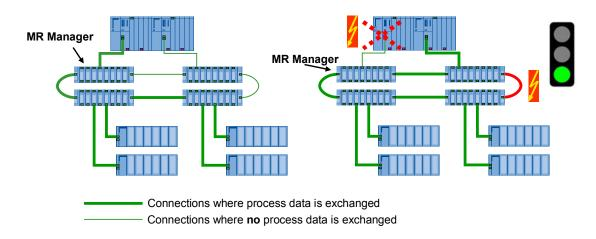
The availability remains due to the media and system redundancy. Despite of the failure of the master CPU and the failure of a ring-connection, the demanded functionality is maintained.
