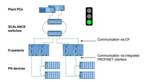
Each SCALANCE switch is located in a ring. If the CPs 443-1 are replaced by the PN interface, a total of three rings is produced (next picture). For this configuration, the CP 443-1 cannot be replaced by the PN interface.
