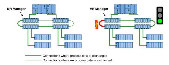
The master CPU exchanges process data with the PN devices (left picture).
