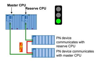
To maintain the functionality by the system redundancy it is unnecessary here which of the three connections fails. Both PN devices can exchange process data with the respective controller process data.
