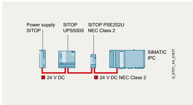
24 V power supply according to NEC Class 2 via a high-performance power supply unit with capacitor-based DC UPS SITOP UPS500S and redundancy module SITOP PSE202U with NEC Class 2
