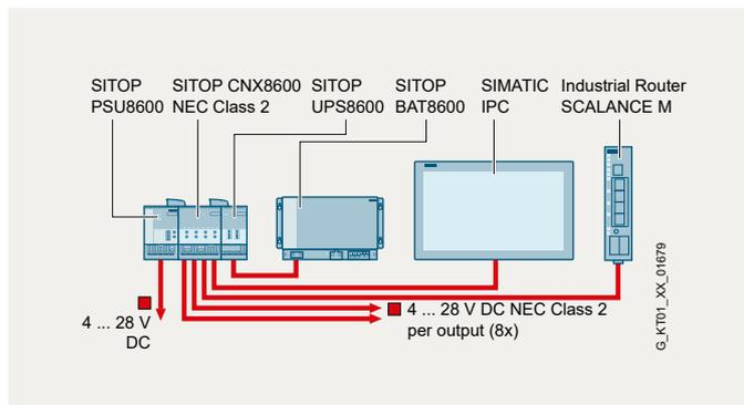
24 V power supply according to NEC Class 2 via power supply system SITOP PSU8600 with expansion module CNX8600 with NEC Class 2 and buffering of the output via DC UPS UPS8600 with battery module BAT8600
