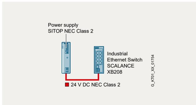
Power supply unit with NEC Class 2, e.g., PSU6200 24 V/3.7 A
