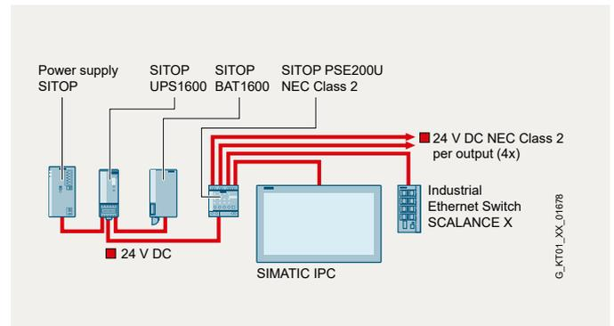
24 V power supply according to NEC Class 2 via a high-performance power supply unit with DC UPS module SITOP UPS1600 and battery module BAT1600 as well as selectivity module SITOP PSE200U with four NEC Class 2 outputs
