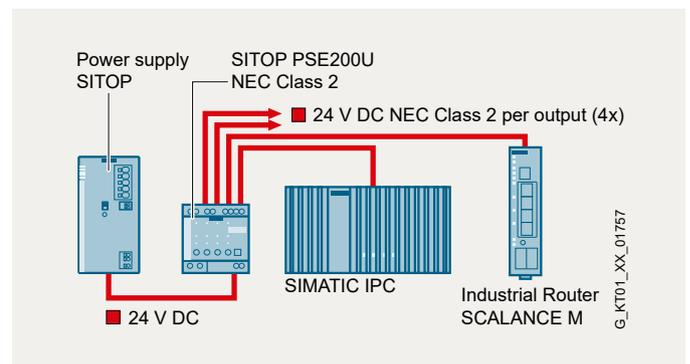
High-performance power supply unit and the selectivity module SITOP PSE200U with NEC Class 2
