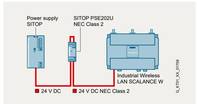
High-performance power supply unit and redundancy module with NEC Class 2
