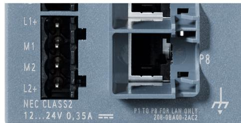
SCALANCE devices with a maximum supply of 100 VA are labeled "NEC CLASS 2" at the 24 V input.
