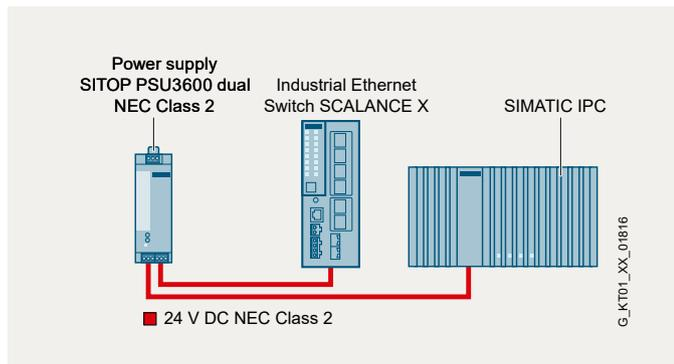
Power supply module SITOP PSU3600 dual with two NEC Class 2 outputs, each adjustable from 12 to 28 V DC
