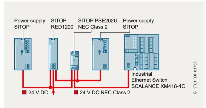
Redundant 24 V supply via two power supply units and redundancy module SITOP PSE202U with NEC Class 2
