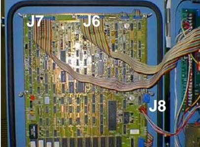
A close-up photograph of the EC board. Three ribbon cables are connected to the board. The cables are labeled J6, J7, and J8. J6 and J7 are at the top, and J8 is at the bottom right. The board is green and populated with various components. |
