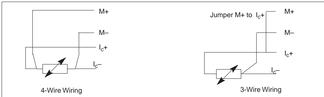
Figure 5 4-Wire and 3-Wire Wiring Diagram
