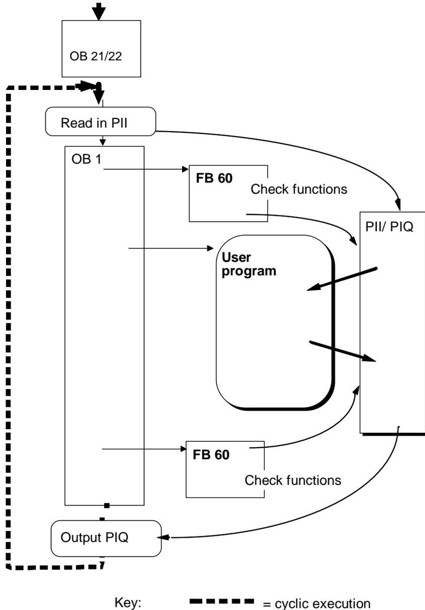
Fig. 2-11 How the Interface Functions in Extended Operation
