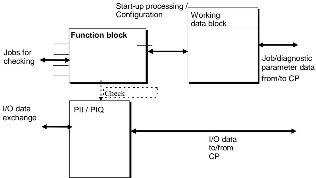
Fig. 2-10 Interface Elements for Extended Operation
