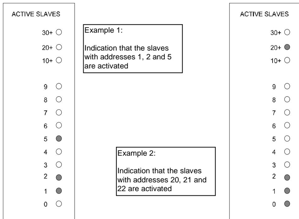
Fig. 2-9 Examples of Indicators on the CP Front Panel
