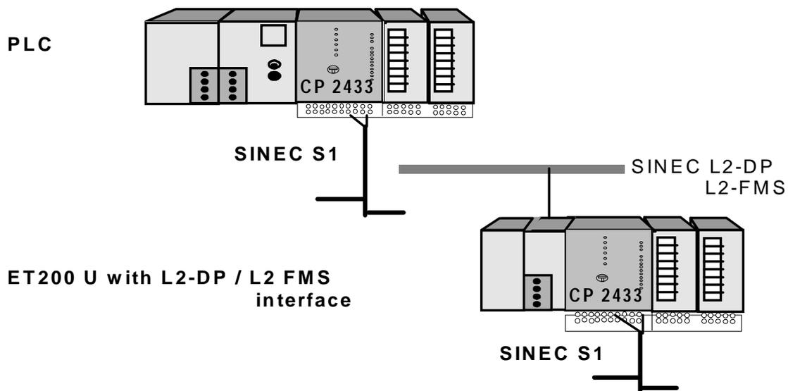
Fig. 2-1 Possible Uses of the SINEC S1 Module CP 2433
