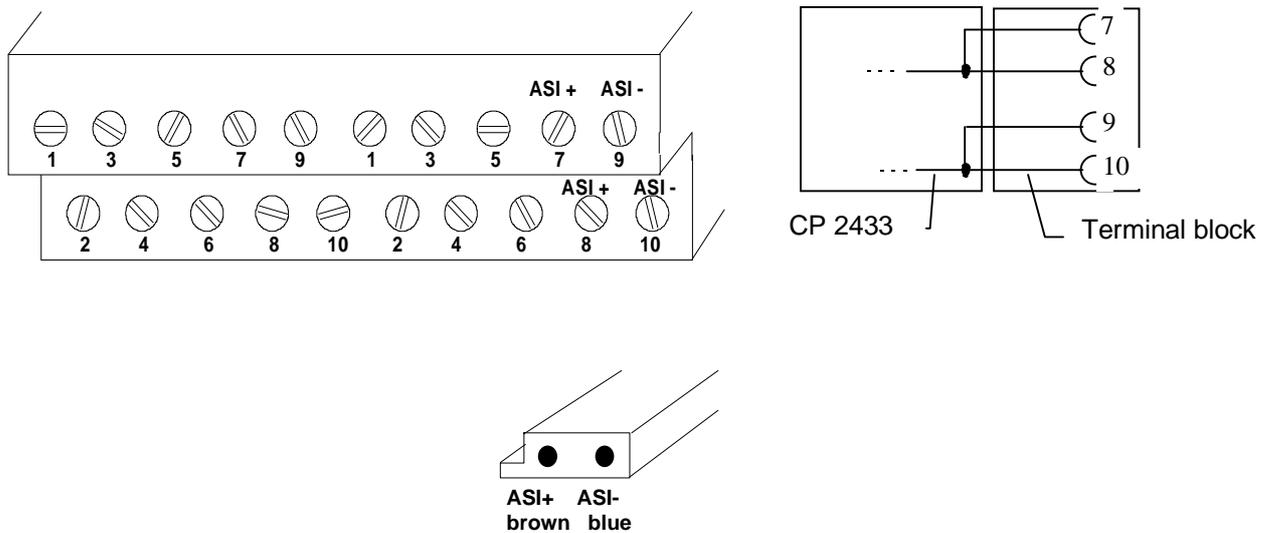
Fig. 2-6 Terminal Block with Connections and AS-I Cable
