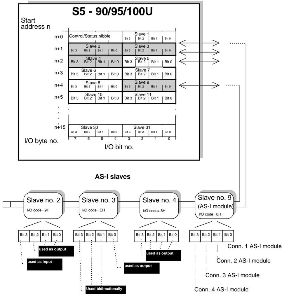
Fig. 2-7 Simulation of the Slave Addresses on the PLC Slots
