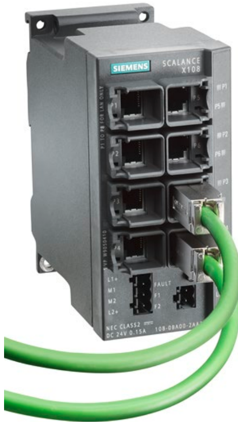
Figure 5-2 Plugging in the IE FC RJ45 Plug 180
