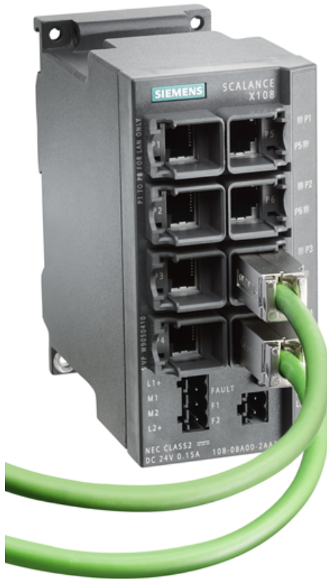
Figure 5-2 Plugging in the IE FC RJ45 Plug 180
