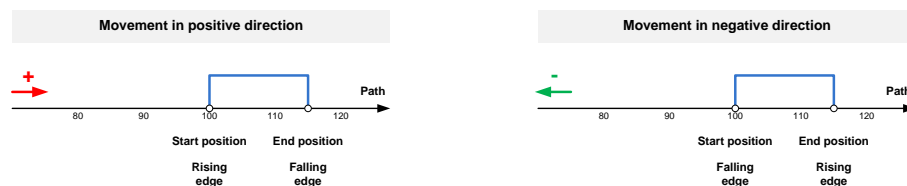
Figure 6-2 Direction-dependency of distance output (position-based) cams
