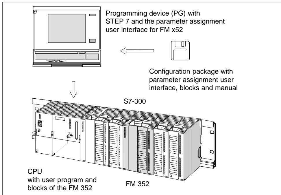
Figure 1-1 Structure of a SIMATIC S7-300 PLC with an FM 352
