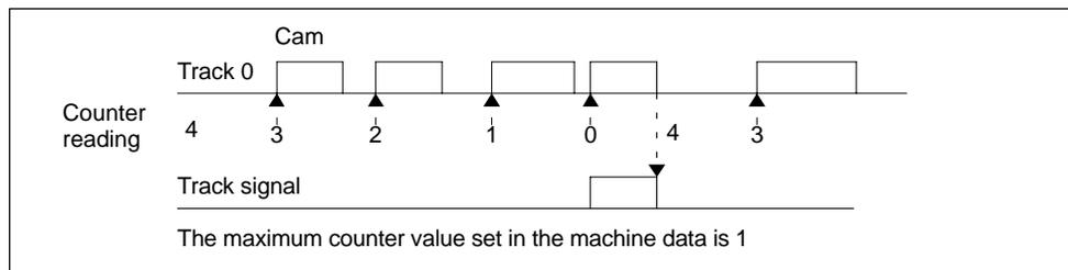
Figure 2-2 Switching a Counter Cam Track
