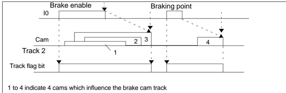
Figure 2-3 Response of a Brake Cam Track
