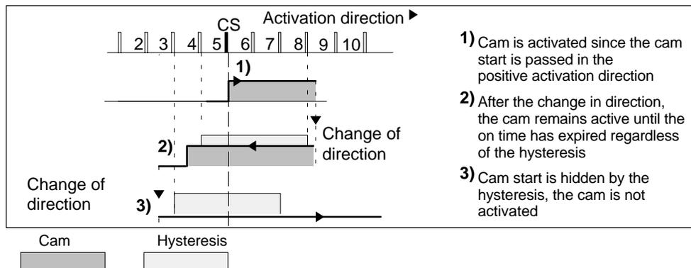
Figure 8-2 Activation of a Time Cam with Hysteresis
