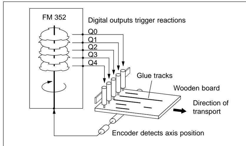
Figure 1-2 Example of an Electronic Cam Control Application
