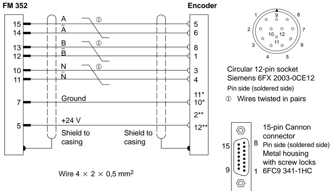
\* Pins 10 and 11 are jumpered internally.
