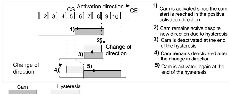
Figure 8-1 Activation of a Distance Cam with Hysteresis
