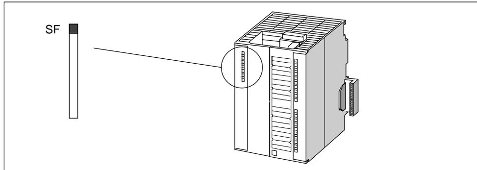
Figure 11-1 Status and Fault/Error Indicator of the FM 352
