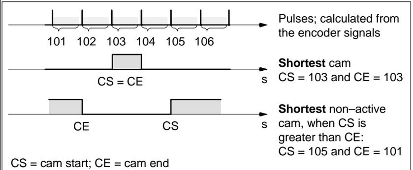
Figure 8-3 Shortest Cam with the Axis Moving in the Positive Direction
