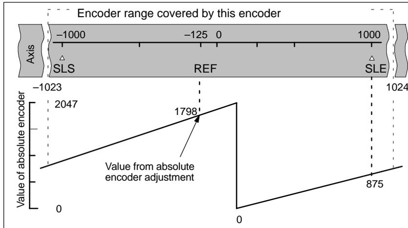
The encoder supplies 2048 defined values. The working range is defined by the software limit switches. Due to the selected resolution of 1 mm per pulse, the encoder can, however, cover a larger working area than intended with the software limit switches.
