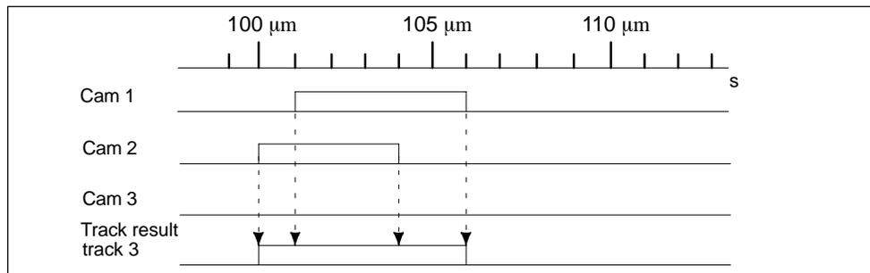
Figure 2-1 Calculating the Track Result
