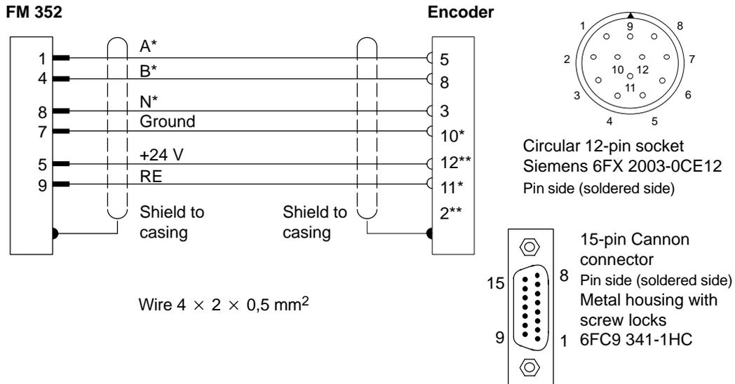
\* Pins 10 and 11 are jumpered internally.
