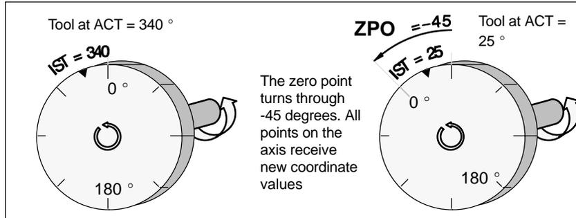
Figure 9-1 Rotation of the Coordinate System Resulting from a Zero Offset
