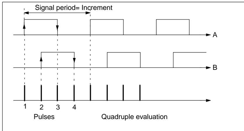
Figure 10-2 Increments and Pulses
