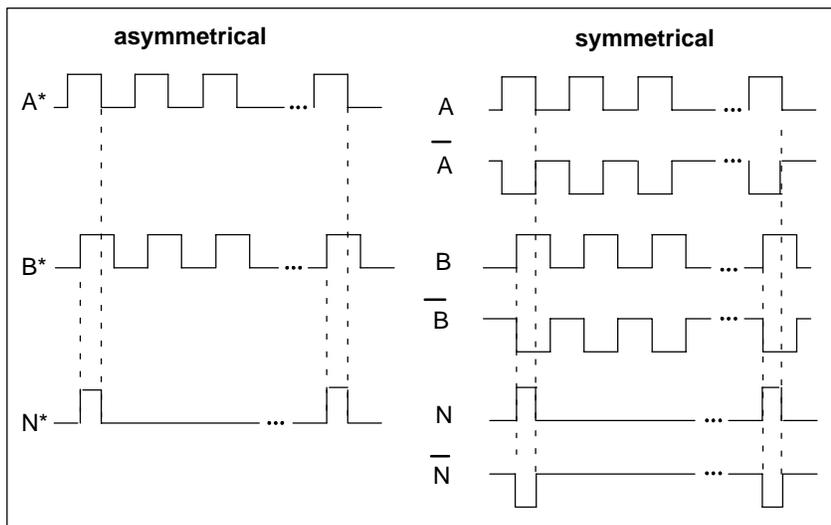
Figure 10-1 Signal Shapes from Incremental Encoders
