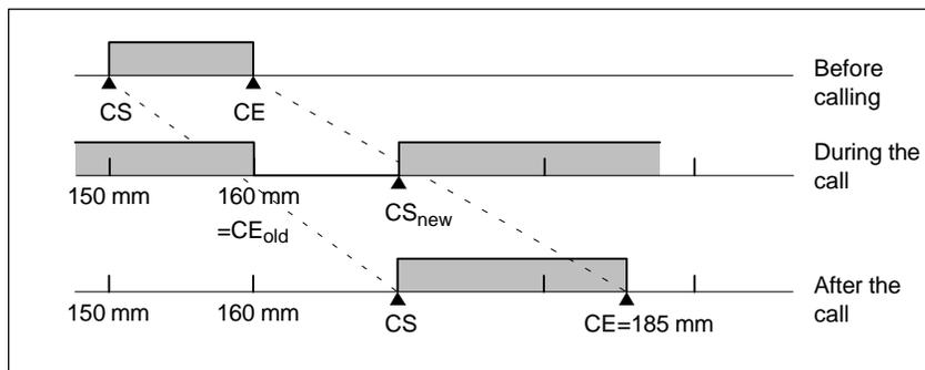
Figure 9-2 Changes in the Cam Edges in Individual Steps
