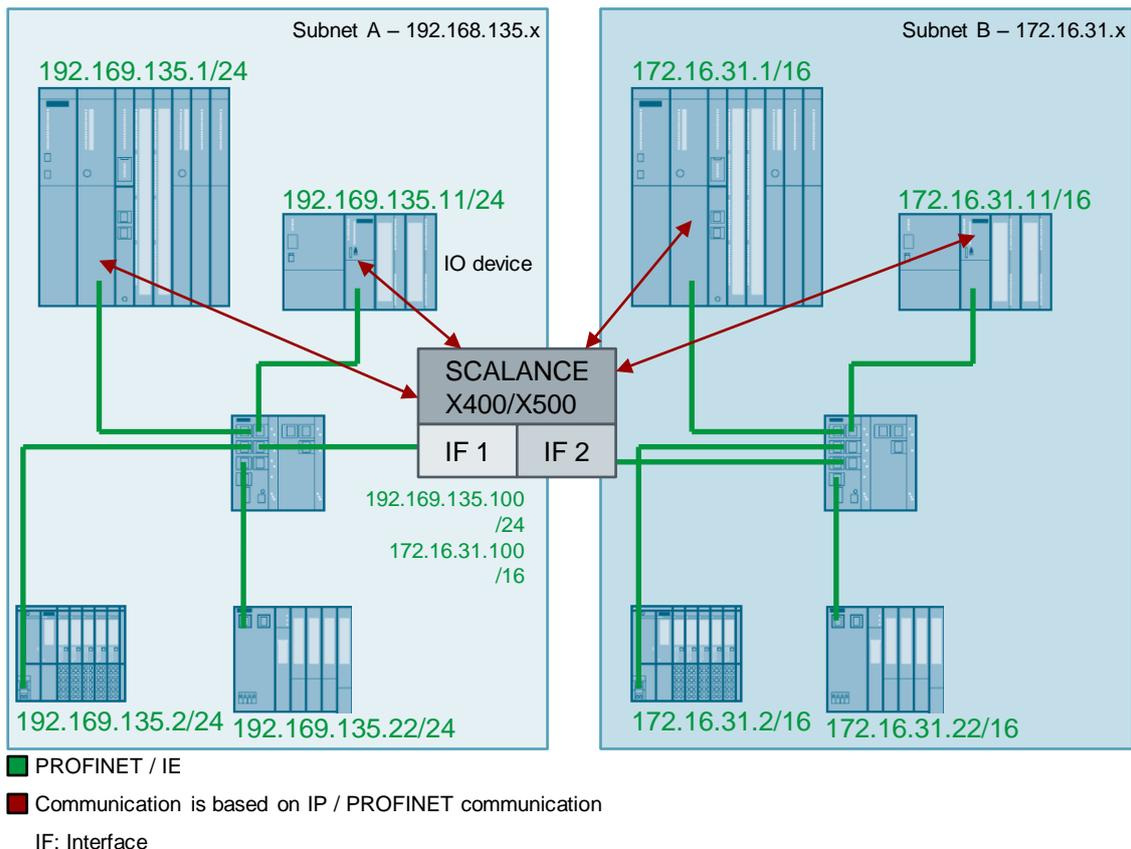
When you connect two IP subnets with each other via a SCALANCE X-400/SCALANCE X-500, you can use the following communication services for data exchange between Subnet A and Subnet B:
