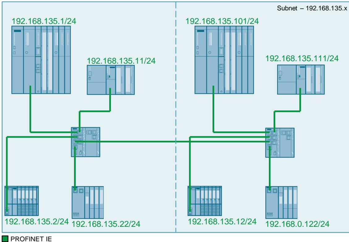
If all the devices are in the same IP subnet you can use the following communication services for data exchange between the devices:
