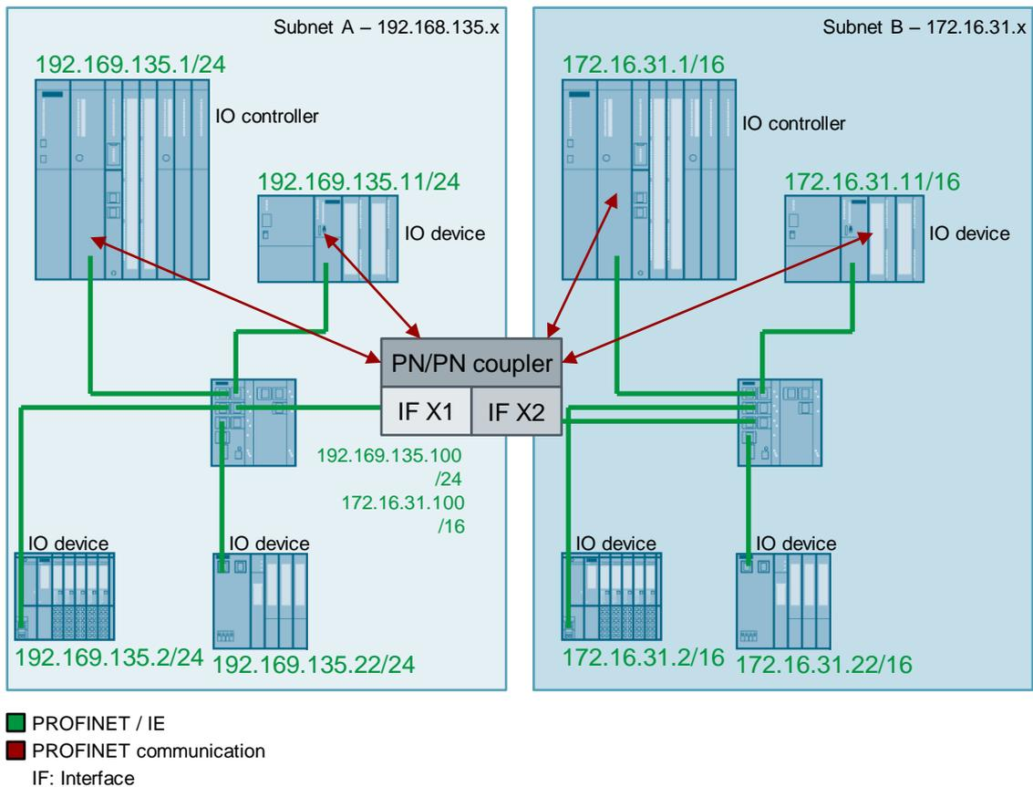
The PN/PN coupler has two interfaces (IF X1 and IF X2). Each interface has 2 ports. IF X1 and IF X2 can be either in the same IP subnet or in two different IP subnets.
