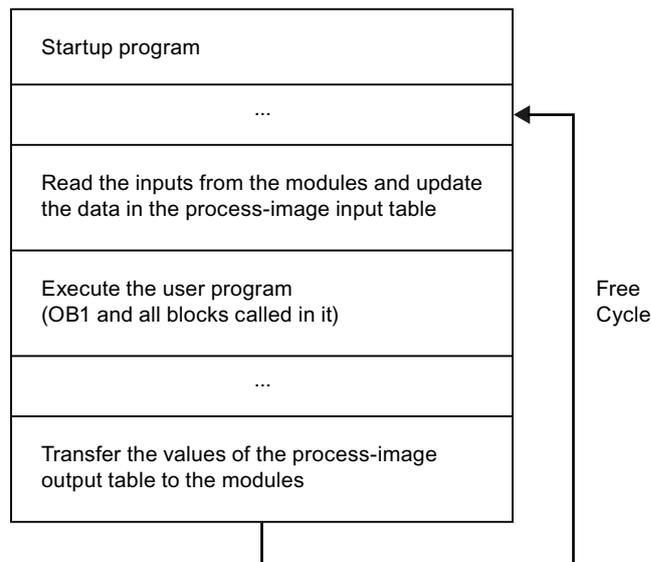
When modifying variables in a simulated CPU from a STEP 7 variable table, you must ensure that process image updates do not overwrite or overlay your intended modification. Set the trigger points for modifying variables as follows:
