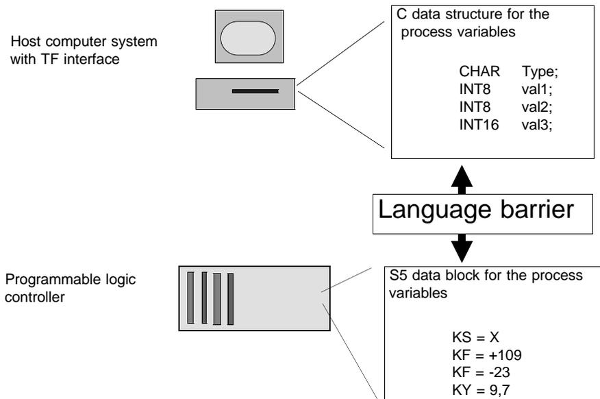
Fig. 2.9: Language Barriers in Communication Between Heterogeneous Devices
