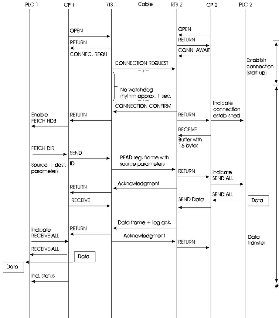
Fig. B.8: Chronological Sequence of WRITE-ACTIVE/PASSIVE
