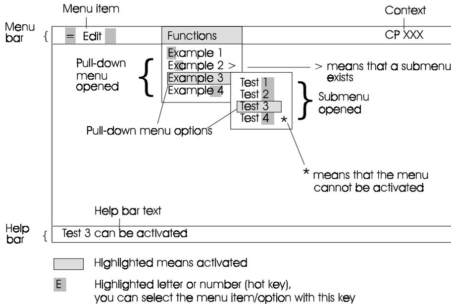
Fig. 5.1: Layout of the SINEC NCM Screen
