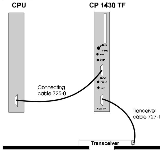
Fig. 4.6: Connecting the PLC with a Swing Cable
