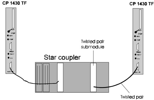
Fig. 4.4: Connecting the CP 1430 TF to SINEC H1 with TP/Star Coupler or Hub
