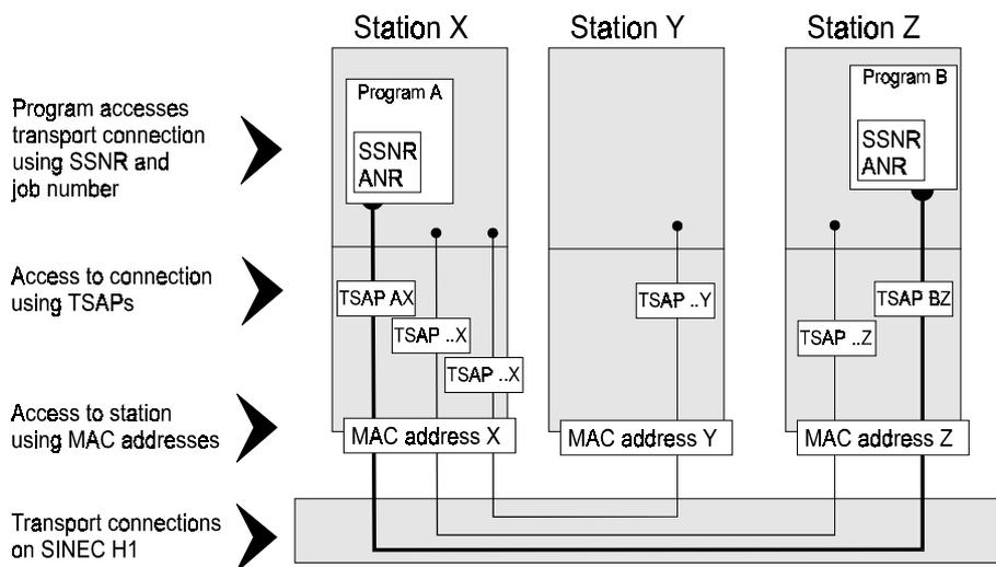
Fig. 2.3: Transport Connections and Addressing
