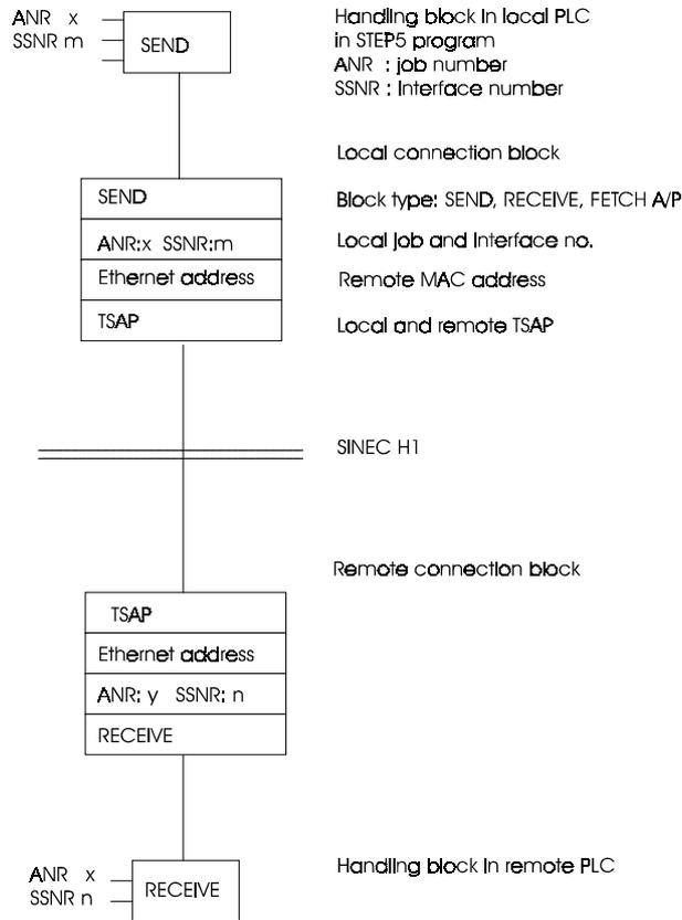
Fig. 7.2: Principle of Transport Connections
