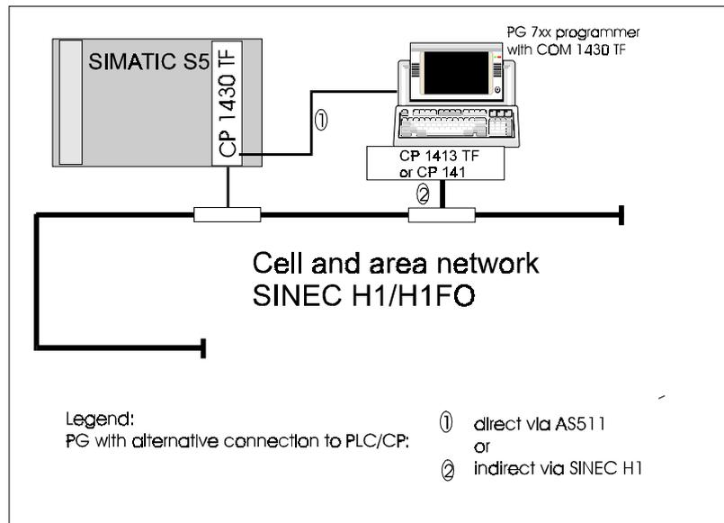
Fig. 1.1: Integration of the CP 1430 TF and COM 1430 TF Configuration Software
