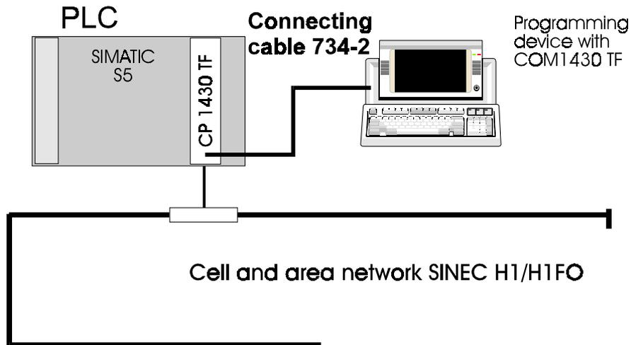
Fig. 4.9 PG Connection using the AS511 Interface
