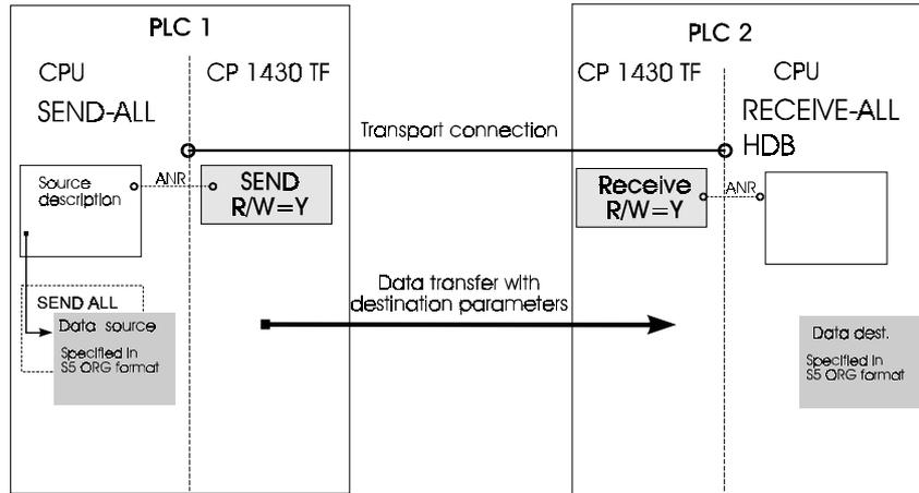
Fig. 3.7: Half Duplex Transmission WRITE Job
