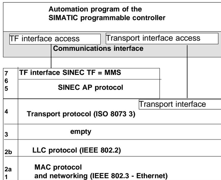
Fig. 1.2: Protocol Profile of the SINEC CP 1430 TF Communications Processor
