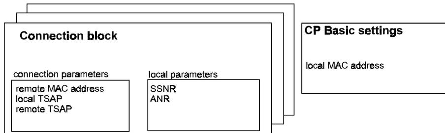
Fig. 2.5: Connection Block and SYSID Block with Transport Parameters
