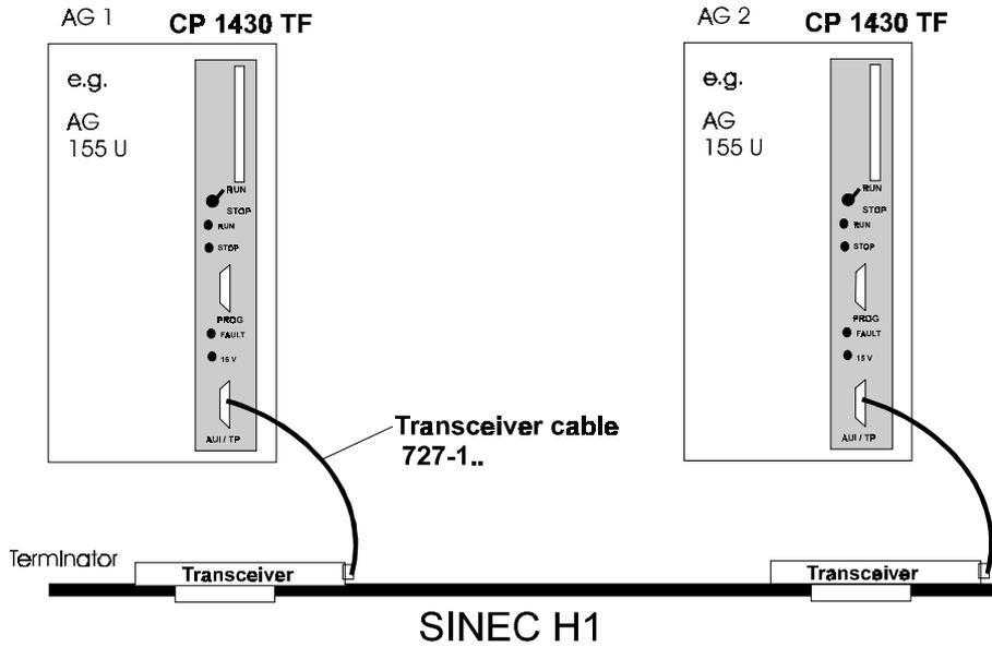
Fig. A.1: System Structure in the Example of Transport Connections
