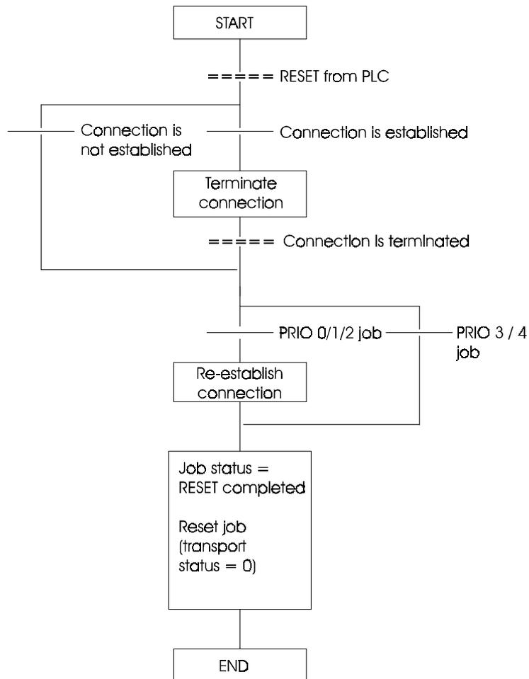
Fig. 3.10: Processing RESET
