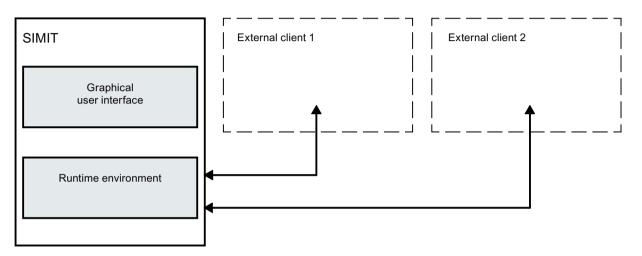
This enables other simulators to be coupled to SIMIT. The operation of the simulation can then be performed by SIMIT or the external simulator.
