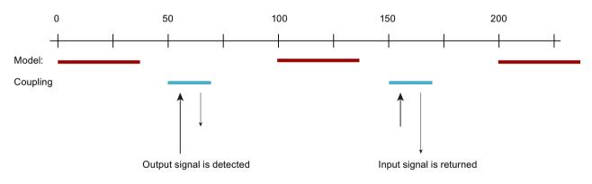
If the model calculation or the data communication of couplings takes longer than half of the cycle time, this time offset does not result in optimization.
