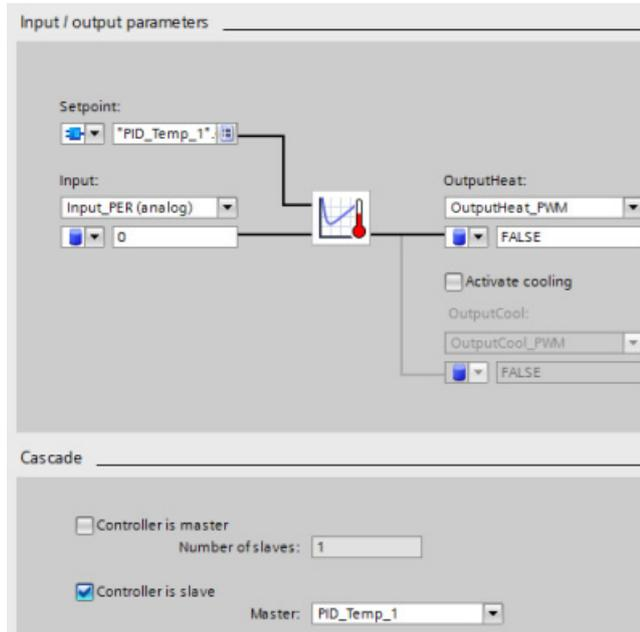
Network 1: In these networks, you make the connection between the "PID\_Temp\_1" master and the "PID\_Temp\_2" slave in the programming editor:
