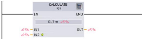
The unconfigured Calculate instruction provides two input parameters and an output parameter.
