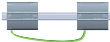
For a direct connection between two CPUs:
