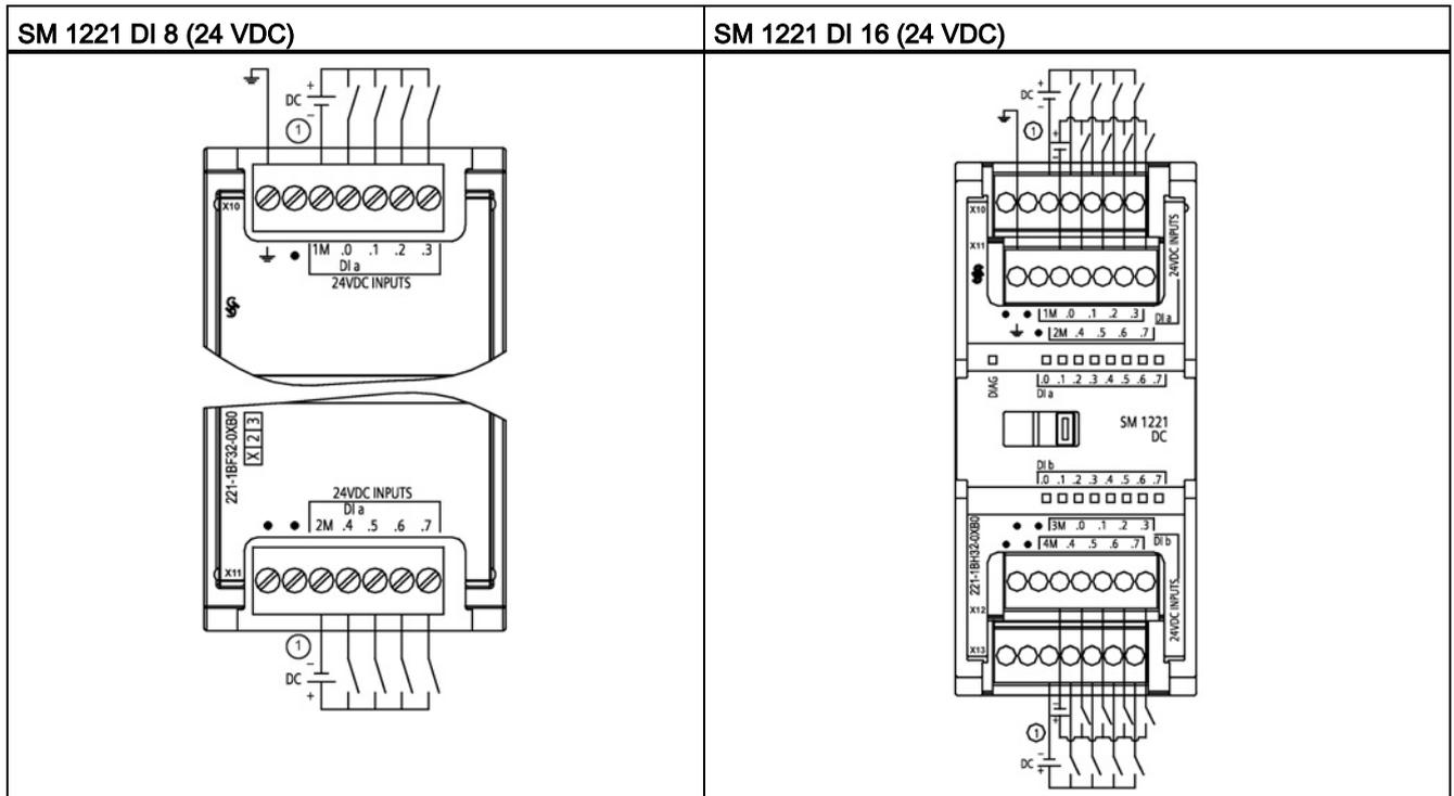
① For sinking inputs, connect "-" to "M" (shown). For sourcing inputs connect "+" to "M".
