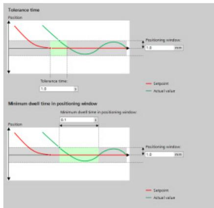
"Positioning monitoring": You can configure tolerance time as well as minimum dwell time for the positioning window.
