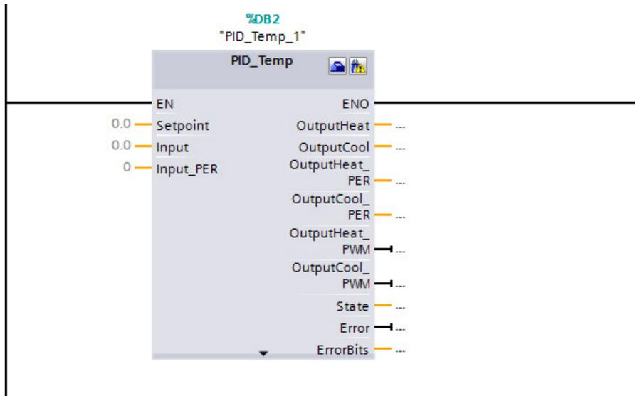
Network 2: You make the connection between the "PID\_Temp\_1" master's "OutputHeat" and "Slave" parameters to the "PID\_Temp\_2" slave's "Setpoint" and "Master" parameters, respectively:
