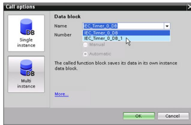
The "Call options" dialog allows you to select a single-instance or multi-instance DB. You can also select specific DBs from a drop-down list of available DBs.
