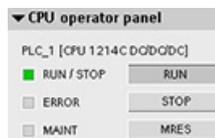
Use the button on the operator panel to change the operating mode (STOP or RUN). The operator panel also provides an MRES button for resetting the memory.
