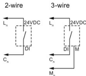
The following illustration shows the configuration for DQ operating mode (2-wire and 3-wire), where  $n$  = port number:
