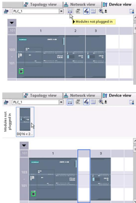
STEP 7 provides a storage area for "unplugged" modules. You can drag a module from the rack to save the configuration of that module. These unplugged modules are saved with your project, allowing you to reinsert the module in the future without having to reconfigure the parameters.
