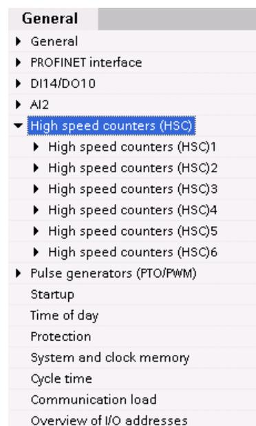
You may configure up to 6 high-speed counters. Edit the CPU device configuration and assign the HSC properties of each individual HSC.
