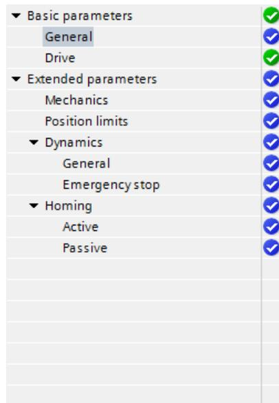
The tree selector for the PTO axis does not include the Encoder, Modulo, Position monitoring, and Control loop configuration menus.
