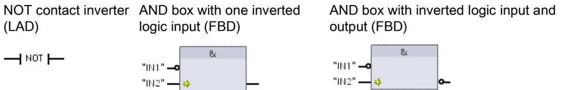
The LAD NOT contact inverts the logical state of power flow input.
