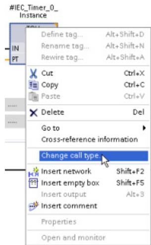
STEP 7 allows you to easily create or change the association of a DB for an instruction or an FB that is in an FB.
