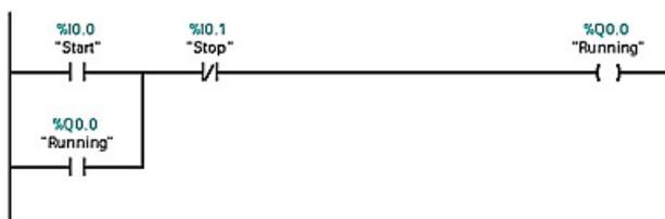
Contacts test the binary status of the bit, with the result being "power flow" if on (1) or "no power flow" if off (0).
