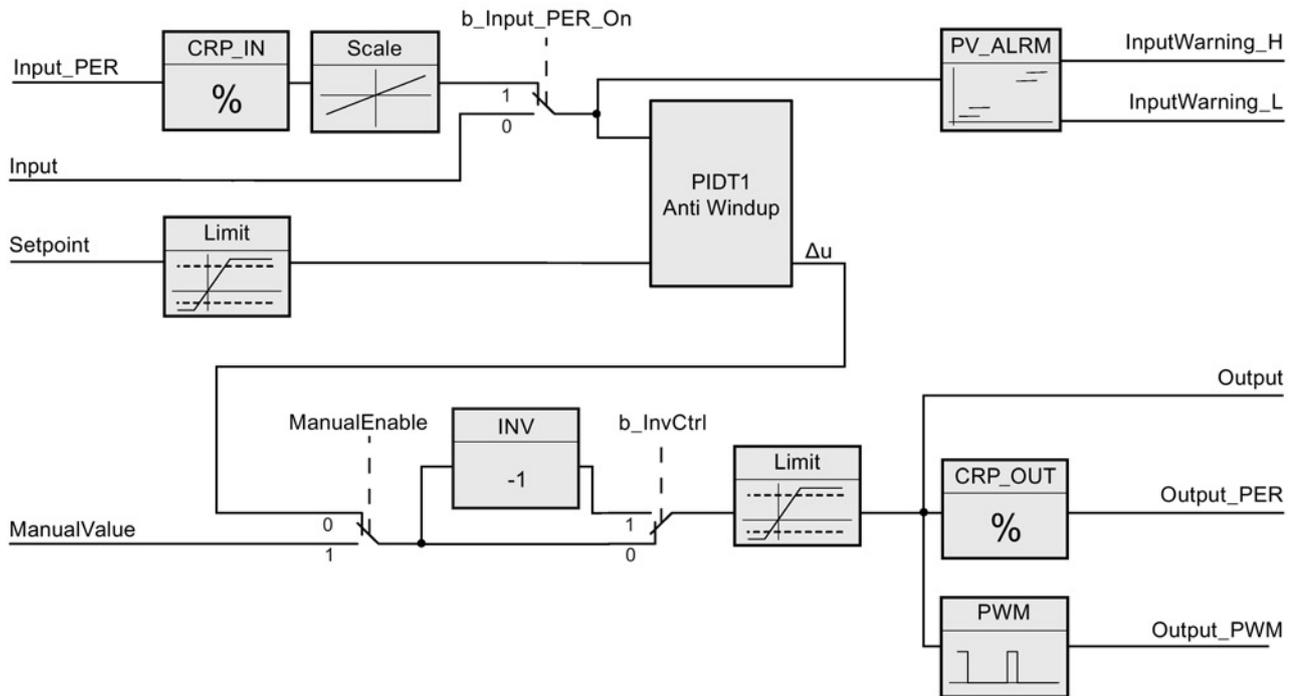
Figure 8-1 Operation of the PID\_Compact controller
