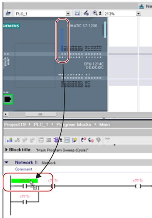
To help you perform tasks quickly and easily, STEP 7 allows you to drag and drop elements from one editor to another. For example, you can drag an input from the CPU to the address of an instruction in your user program.
