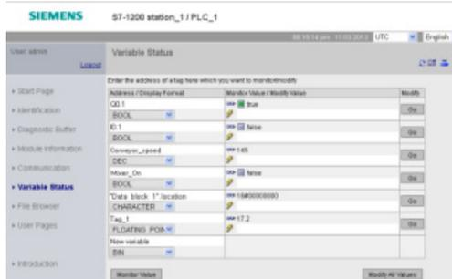
The Variable Status page allows you to monitor or modify any of the I/O or memory data in your CPU. You must have the "read variable status" privilege to monitor values, and the "write variable status" privilege to modify values. You can enter a direct address (such as I0.0), a PLC tag name, or a tag from a specific program block. The data values automatically refresh until you disable the automatic refresh option.
