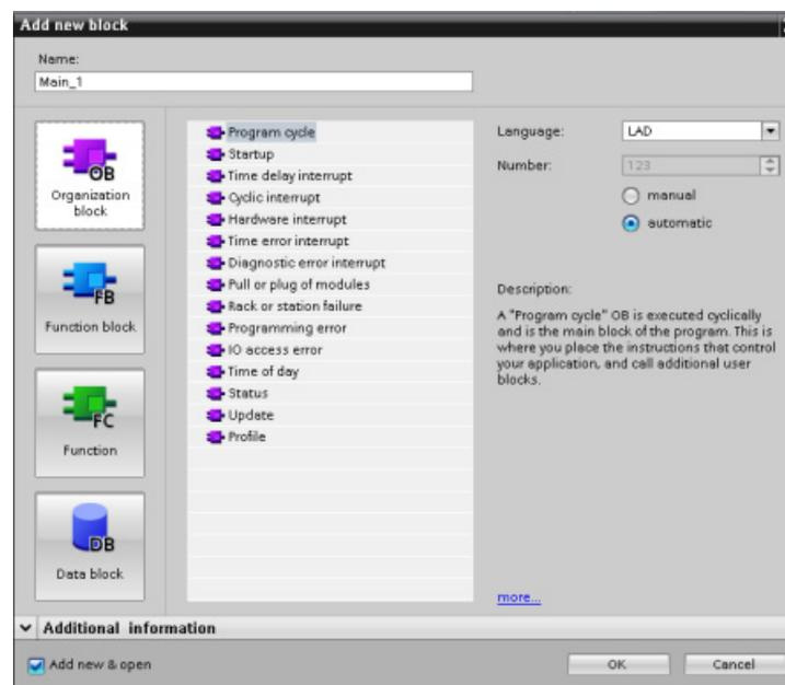
Interrupt handling is always event-driven. When such an event occurs, the CPU interrupts the execution of the user program and calls the OB that was configured to handle that event. After finishing the execution of the interrupting OB, the CPU resumes the execution of the user program at the point of interruption.
