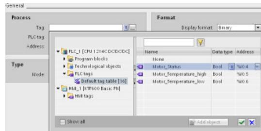
You can also drag and drop PLC tags from the Project tree to the HMI screen. Display the PLC tags in the "Details" view of the project tree and then drag the tag to the HMI screen.
