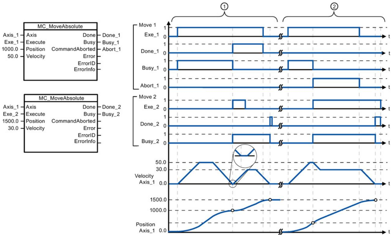
The following values were configured in the "Dynamics > General" configuration window: Acceleration = 10.0 and Deceleration = 10.0
