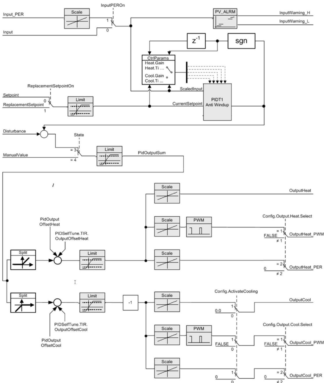
Figure 8-6 PID\_Temp\_Operation\_Block\_Diagram
