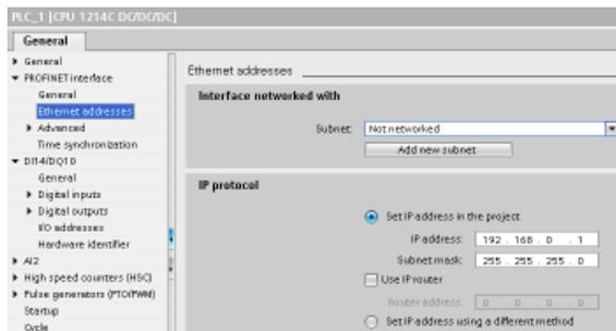
Selecting the CPU in the Device view displays the CPU properties in the inspector window. Use these properties to configure the operational parameters of the CPU (Page 80).
