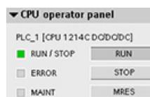
The CPU does not provide a physical switch for changing the operating mode. To change the operating mode of the CPU, STEP 7 provides the following tools:
