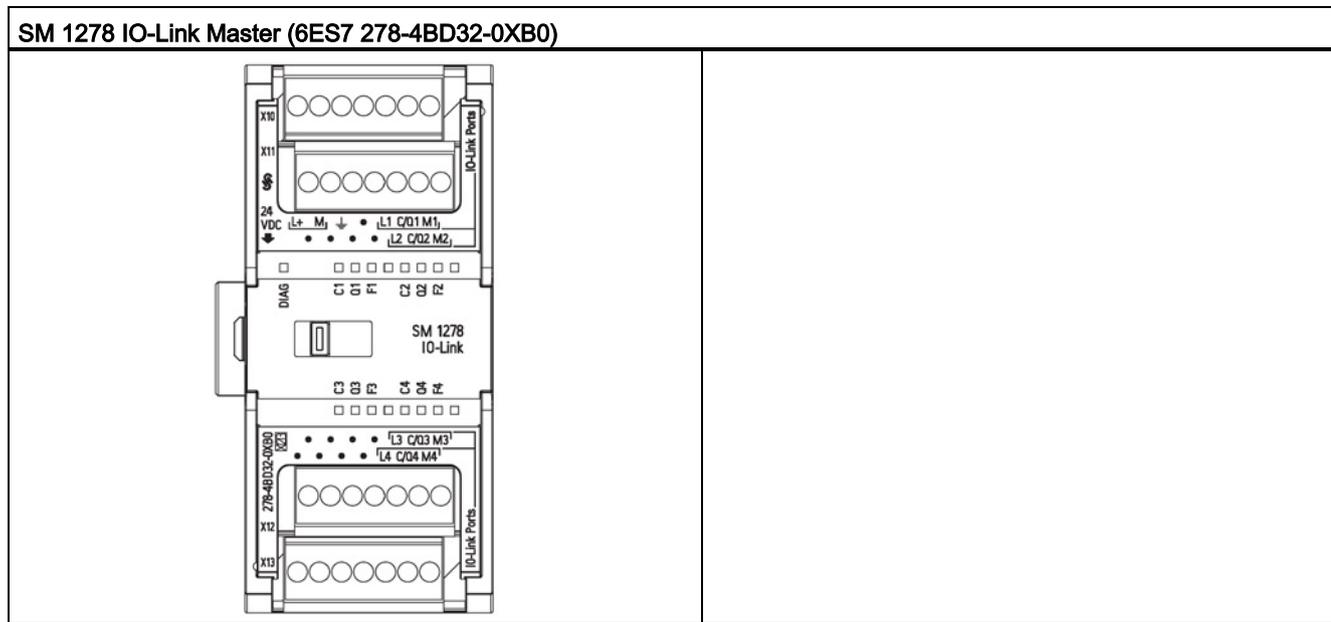
Table A- 79 Connector pin locations for SM 1278 IO-Link Master (6ES7 278-4BD32-0XB0)
