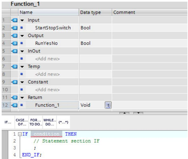
In the Interface section of the SCL code block you can declare the following types of parameters:
