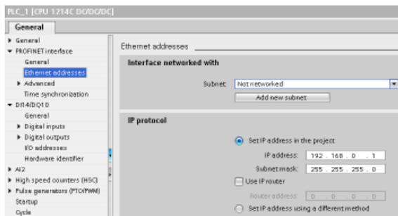
After determining the IP address and subnet mask for the CPU, enter the IP address for the CPU and for the router (if applicable). Refer to the *S7-1200 Programmable Controller System Manual* for more information.
