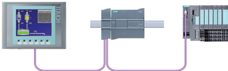
If a CM 1242-5 and a CM 1243-5 are installed together, an S7-1200 can perform as both a slave of a higher-level DP master system and a master of a lower-level DP slave system, simultaneously:
