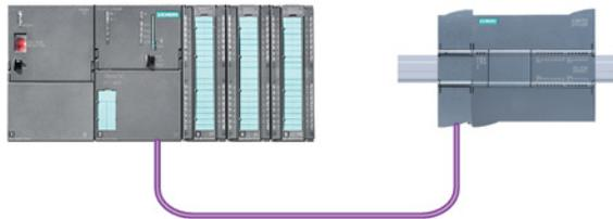
The S7-1200 is connected to a PROFIBUS network as a DP master with the CM 1243-5 communication module. The CM 1243-5 (DP master) module can be the communications partner of DP V0/V1 slaves. In the figure below, the S7-1200 is a master controlling an ET200S DP slave:
