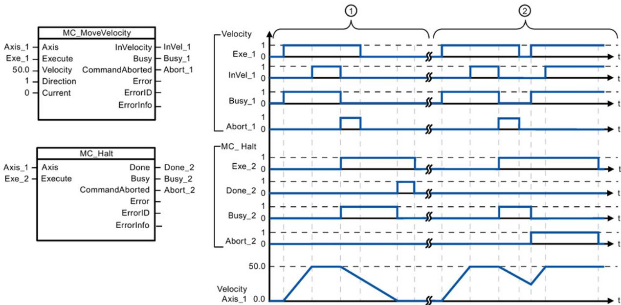
The following values were configured in the "Dynamics > General" configuration window: Acceleration = 10.0 and Deceleration = 5.0
