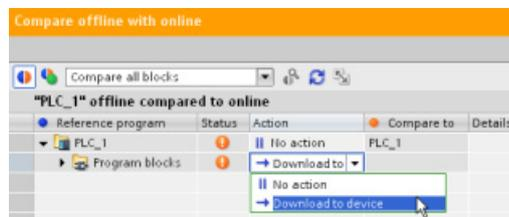
Click in the "Action" column for an object to select whether to delete the object, take no action, or download the object to the device.
