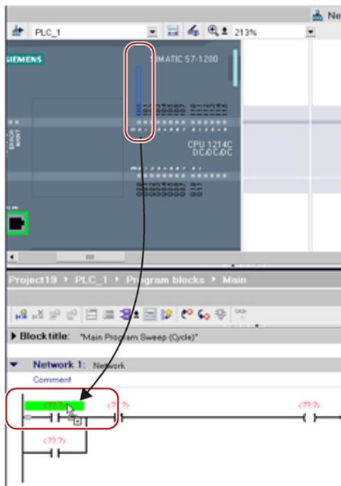
You can also drag the I/O addresses directly from the CPU. Simply split the work area of the Project view (Page 34).
