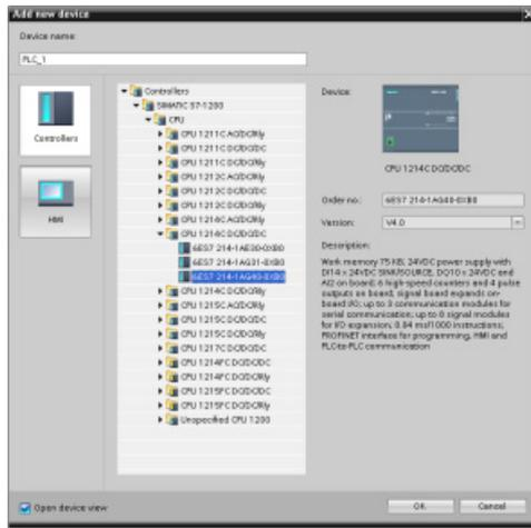
You create your device configuration by inserting a CPU into your project. Select the CPU in the "Add a new device" dialog and click "OK" to add the CPU to the project.
