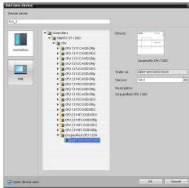
In the device configuration (Project view or Portal view), add a new device, but select the "unspecified CPU" instead of selecting a specific CPU. STEP 7 creates an unspecified CPU.
