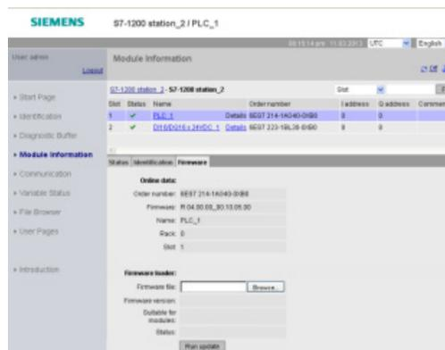
The Module Information page in addition to displaying information about the modules in your station allows you to update the version of firmware in your CPU or other modules that support firmware update. Users with privileges to query diagnostics can view the module information page. Users with privileges to perform a firmware update can update firmware.
