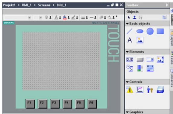
STEP 7 provides a standard set of libraries for inserting basic shapes, interactive elements, and even standard graphics.
