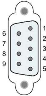
Table A- 63 Pinout of the D-sub socket
