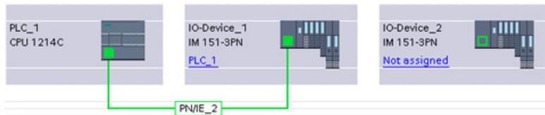
When you download the new network connections, the CPU must be set to STOP mode.
