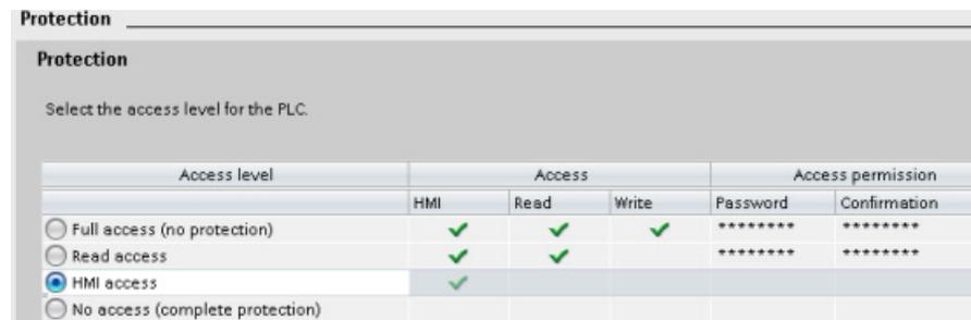
When you download this configuration to the CPU, the user has HMI access and can access HMI functions without a password. To read data, the user must enter the configured password for "Read access" or the password for "Full access (no protection)". To write data, the user must enter the configured password for "Full access (no protection)".
