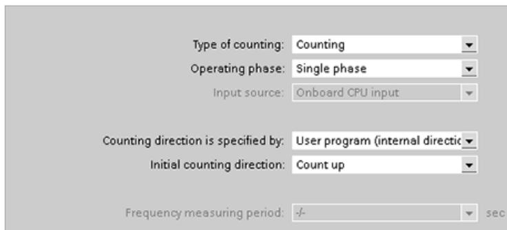
The image shows a configuration window for a High-Speed Counter (HSC). It contains several dropdown menus and a text input field. The parameters are as follows:
