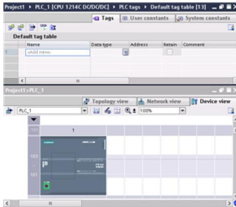
STEP 7 displays both the tag table and the device editor together.
