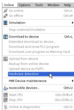
After creating the unspecified CPU, you can upload the hardware configuration for the online CPU.
