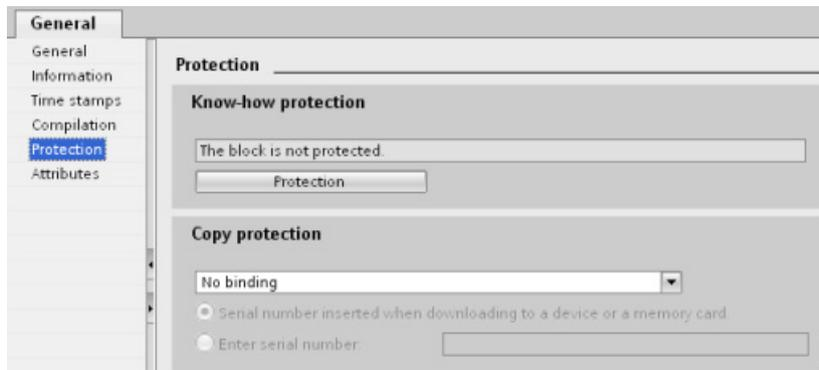
1. In the Properties for the code block, click the "Protection" button to display the "Know-how protection" dialog.
