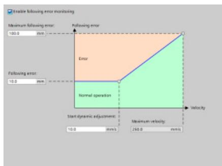
"Following error": You can configure the difference of the allowed error distance over a velocity range. You check the "Enable following error monitoring" check box to activate following error. You can configure the following the parameters:
