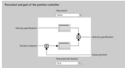
"Control loop": You can configure the velocity gain known as "Precontrol (Kv factor)".
