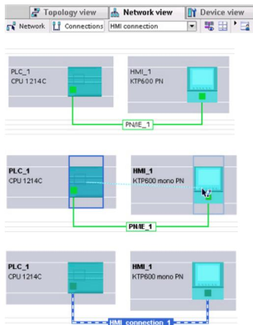
By creating an HMI connection between the two devices, you can easily share the tags between the two devices.
