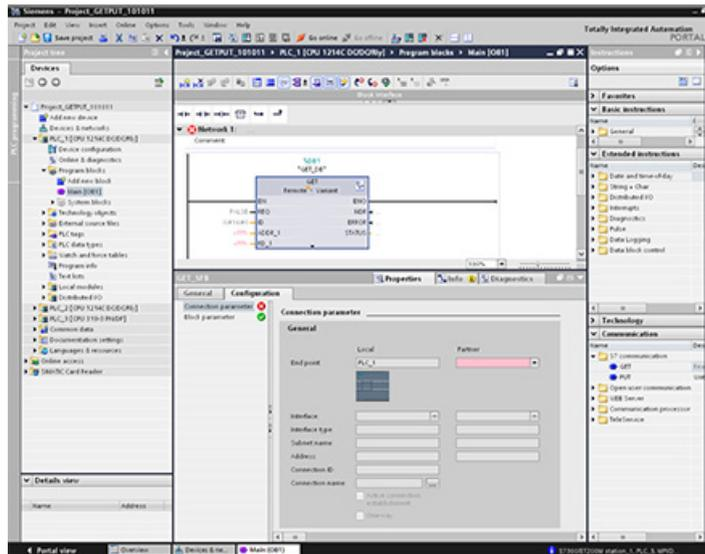
The inspector window displays the properties of the connection whenever you have selected any part of the instruction. Specify the communication parameters in the "Configuration" tab of the "Properties" for the communication instruction.
