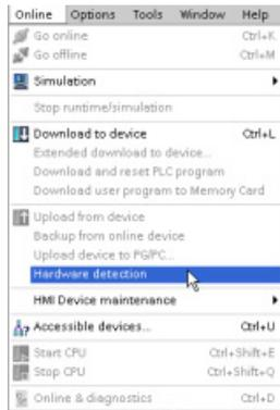
If you are connected to a CPU, you can upload the configuration of that CPU, including any modules, to your project. Simply create a new project and select the "unspecified CPU" instead of selecting a specific CPU. (You can also skip the device configuration entirely by selecting the "Create a PLC program" from the "First steps". STEP 7 then automatically creates an unspecified CPU.)
