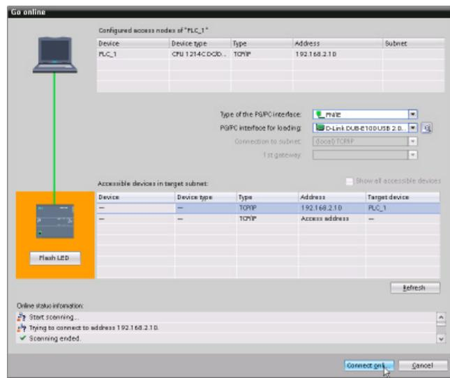
If this is the first time to go online with this CPU, you must select the type of PG/PC interface and the specific PG/PC interface from the Go Online dialog before establishing an online connection to a CPU found on that interface.
