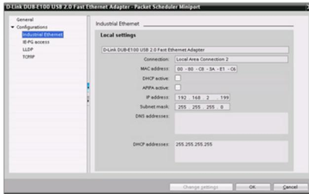
The "Properties" window displays the settings for the programming device.
