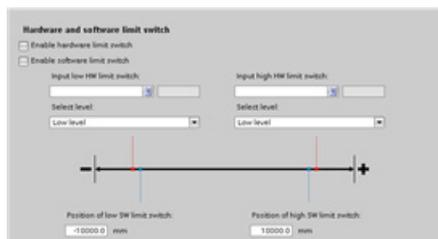
**Position limits:** You can configure the properties for the drive signals, drive mechanics, and position monitoring (hardware and software limit switches).
