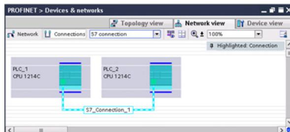
Click the "Highlighted: Connection" button to access the "Properties" configuration dialog of the communication instruction.
