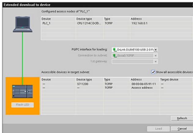
After completing the configuration, download the project to the CPU. The IP addresses for the CPU and for the router (if applicable) are configured when you download the project.
