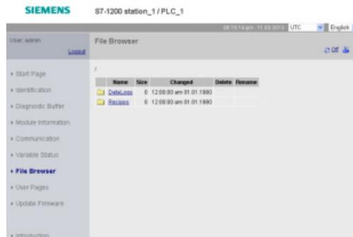
The File Browser page allows you to view, download, or edit files in the load memory of the CPU such as data logs (Page 122) and recipes. Unless the CPU has Level 4 protection, all users can view the files from the File Browser page. Users with privileges to modify files can delete, edit and rename files.
