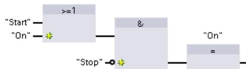
To create the logic for complex operations, insert parallel branches between the boxes.
