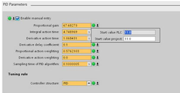
The figure above shows the PID parameter screen with compare icons showing which values are different between online and offline projects. A green icon indicates that the values are the same; a blue/orange icon indicates that the values are different.
