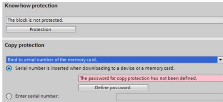
3. For binding to the serial number of a CPU or memory card, select either to insert the serial number when downloading, or enter the serial number for the memory card or CPU.
