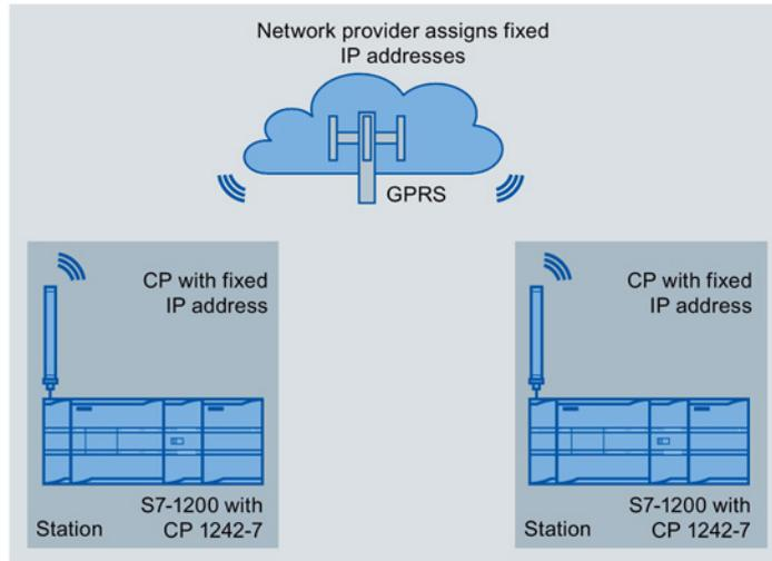
Figure 7-2 Direct communication between two S7-1200 stations
