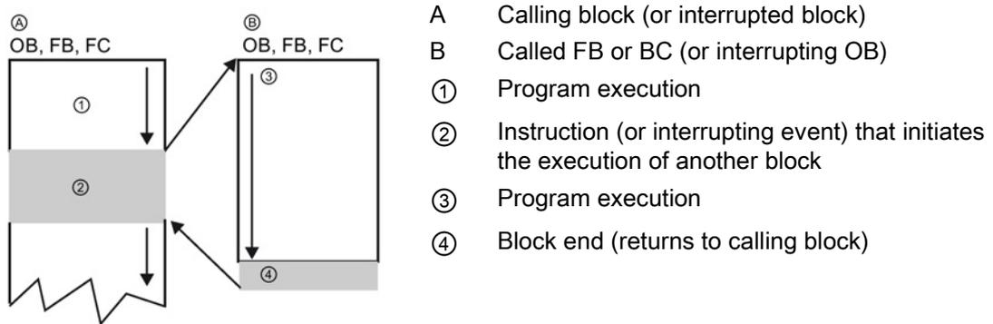
You can nest the block calls for a more modular structure. In the following example, the nesting depth is 3: the program cycle OB plus 3 layers of calls to code blocks.
