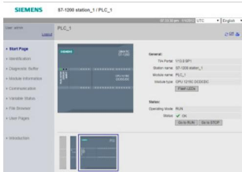
The Start page displays a representation of the CPU to which you are connected and lists general information about the CPU. If you have Web-server enabled CPs the Start page also displays them and allows you to connect to Web pages through those CPs.
