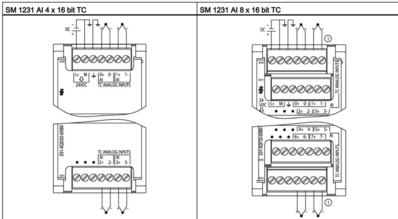
① SM 1231 AI 8 TC: For clarity, TC 2, 3, 4, and 5 are not shown connected.
