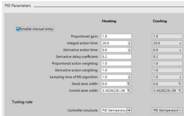
The figure above shows the PID parameter screen with compare icons showing which values are different between online and offline projects. A green icon indicates that the values are the same; a blue/orange icon indicates that the values are different.
