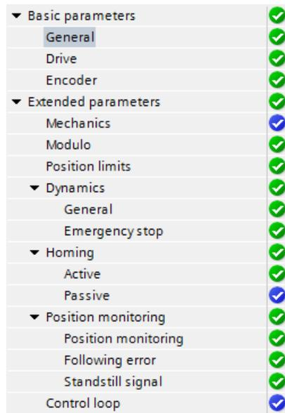
The tree selector for the analog drive or PROFIdrive connection includes the Encoder, Modulo, Position monitoring, and Control loop configuration menus.
