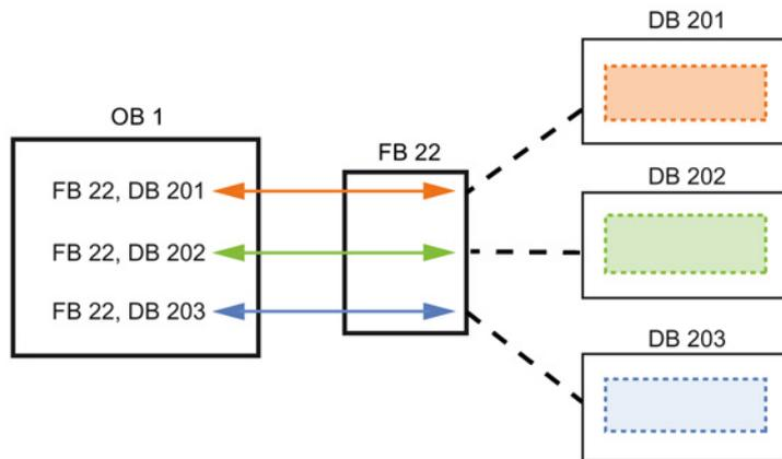
Each instance DB stores the data (such as speed, ramp-up time, and total operating time) for an individual device. In this example, FB 22 controls three separate devices, with DB 201 storing the operational data for the first device, DB 202 storing the operational data for the second device, and DB 203 storing the operational data for the third device.
