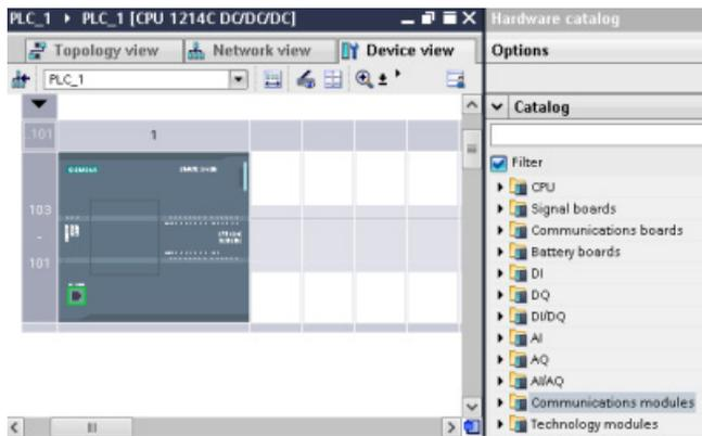
The Device view shows the CPU and rack.
