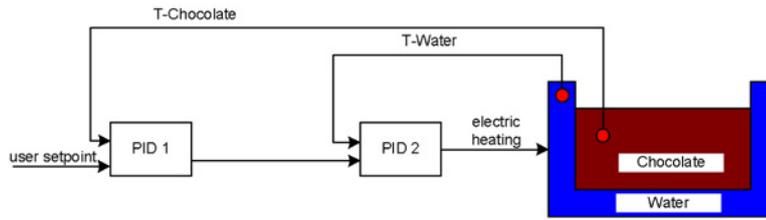
Figure 8-7 PID\_Temp\_Cascade\_Operation\_Block\_Diagram
