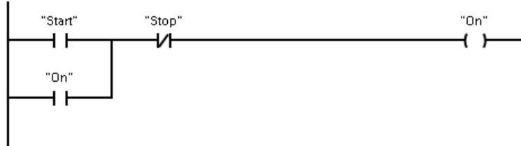
To create the logic for complex operations, you can insert branches to create the logic for parallel circuits. Parallel branches are opened downwards or are connected directly to the power rail. You terminate the branches upwards.
