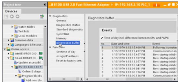
While the CPU maintains power, up to 50 most recent events are available in this log. When the log is full, a new event replaces the oldest event in the log.
