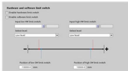
Configure the properties for the drive signals, drive mechanics, and position monitoring (hardware and software limit switches).
