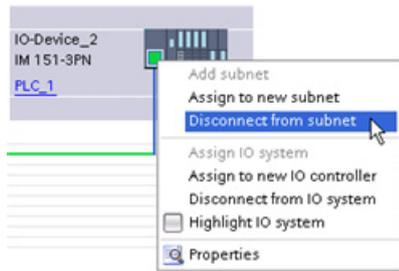
Right-click the interface port of the network device and select the "Disconnect from subnet" command from the context menu.
