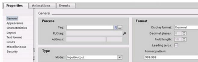
You can also create elements on your screen by dragging and dropping PLC tags either from the Project tree or the program editor to the HMI screen. The PLC tag becomes an element on the screen. You can then use the properties to change the parameters for this element.
