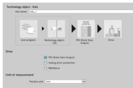
After you create the technology object for the axis, you configure the axis by defining the basic parameters, such as the PTO and the configuration of the drive interface. You also configure the other properties of the axis, such as position limits, dynamics, and homing.
