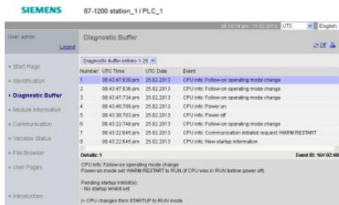
The Diagnostic Buffer page displays the diagnostic buffer, and is accessible to users with privileges to query diagnostics. You can select the range of diagnostic entries to be displayed.
