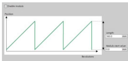
**Modulo:** You can configure a "Modulo" axis to move the load in a cyclic area which has a start value/start position and a given length. If the position of the load reaches the end of this area, it is automatically set to the start value again. You enable the "Length" and "Modulo start value" fields when you check the "Enable Modulo" check box.
