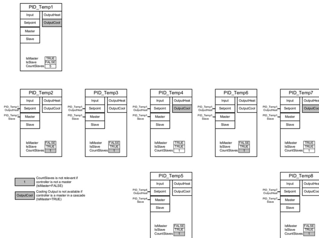
Figure 8-8 PID\_Temp\_Cascading\_communication\_connection
