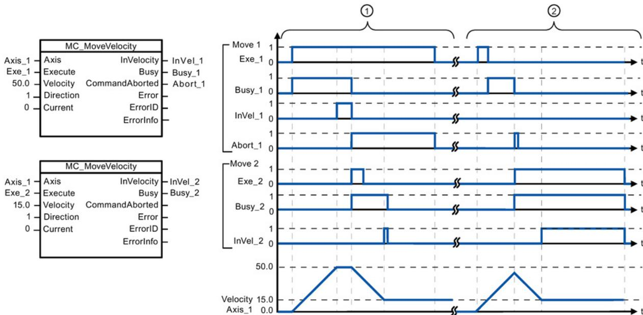
The following values were configured in the "Dynamics > General" configuration window: Acceleration = 10.0 and Deceleration = 10.0
