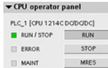
The color of the RUN/STOP indicator shows the current operating mode of the CPU: yellow indicates STOP mode, and green indicates RUN mode.
