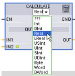
Click the "???" and select the data types for the input and output parameters. (The input and output parameters must all be the same data type.)
