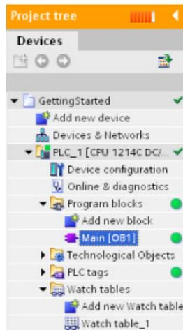
When you have connected to the CPU, STEP 7 turns the headers of the work areas orange.
