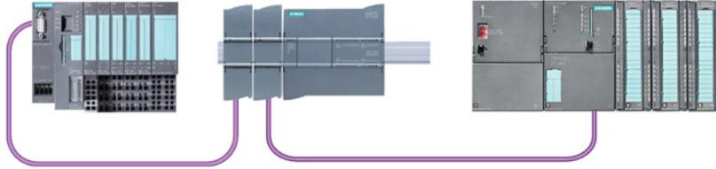
For V4.0, you can configure a maximum of three PROFIBUS CMs per station, in which there can be any combination of DP master or DP slave CMs. DP masters in a V3.0 or greater CPU firmware implementation can each control a maximum of 32 slaves.
