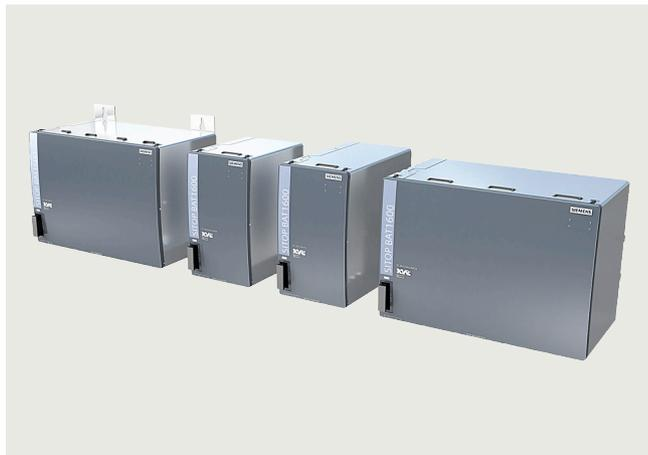
The intelligent UPS1600 battery management charges the BAT1600 with the optimum temperature-controlled charging characteristics and monitors the status (operating data and diagnostic information) of the connected battery modules via the energy storage link. For longer buffer times, up to six battery modules can be connected in parallel. These can be mounted onto a DIN rail or directly on the wall.
