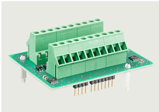
**IO shield for SIMATIC IOT2000 industrial IoT gateway**
