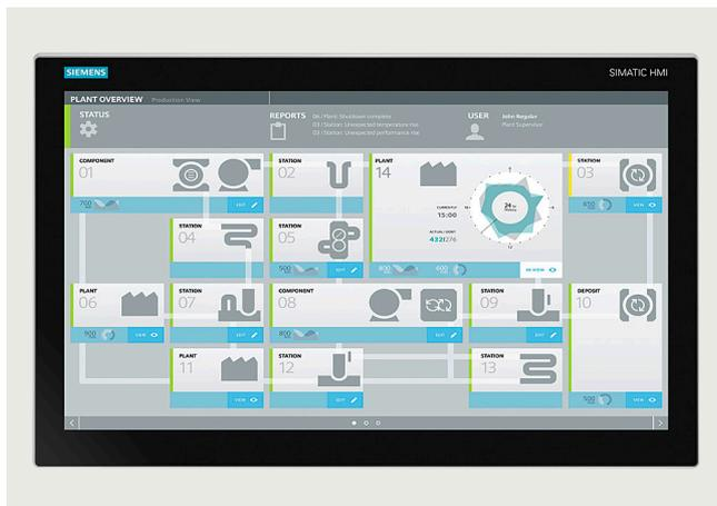
**SIMATIC IPC277G: The Panel PC with optimized performance – flexible in respect of interfaces and expansions with multi-touch displays from 7" to 24"**
