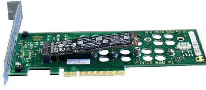
2. Carefully press down the M.2 NVMe SSD and secure it on the PCIe adapter card with the screw.
