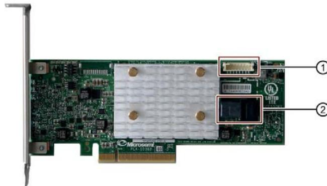
7. Insert the adapter cable at the marked position ②.
