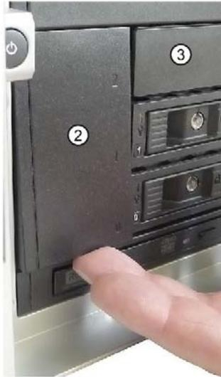
4. Remove the blanking plates ③ which may be located to the right of the cover at the front of the drive cage.
