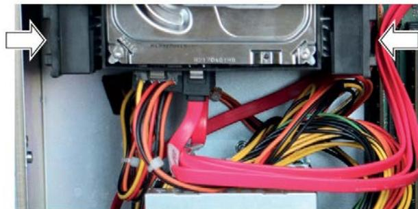
3. Remove the left and right drive mounting bars ② and the drive bay cover ③ from the drive.
