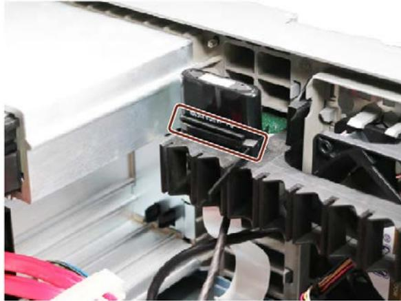
6. Insert the connector of the capacitor block cable at the marked position ①.
