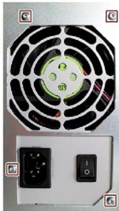
4. Pull the power supply upward and out of the housing.
