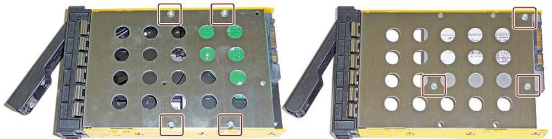
6. Carefully insert the new drive into the removable tray.
