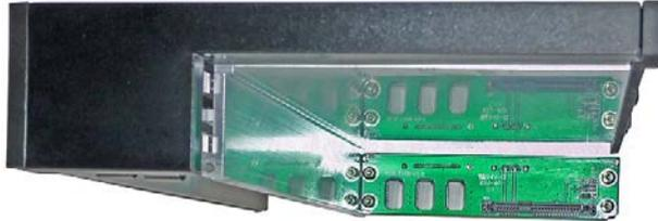
4. Attach the data cables to the desired connectors on the motherboard or the hardware RAID controller and to the adapter module.
