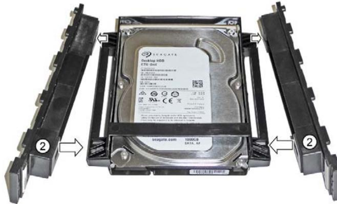
8. Slide the drive bay evenly into the guide rail of the drive cage 3/4 to the rear without tilting it left or right.
