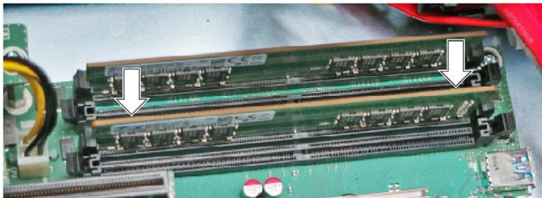
5. Evenly press on both sides of the memory module to avoid tilting until the two locks audibly engage.
