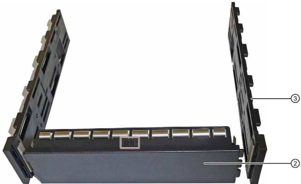
3. Remove the left and right drive mounting bars ③ and the blanking plate ②.
