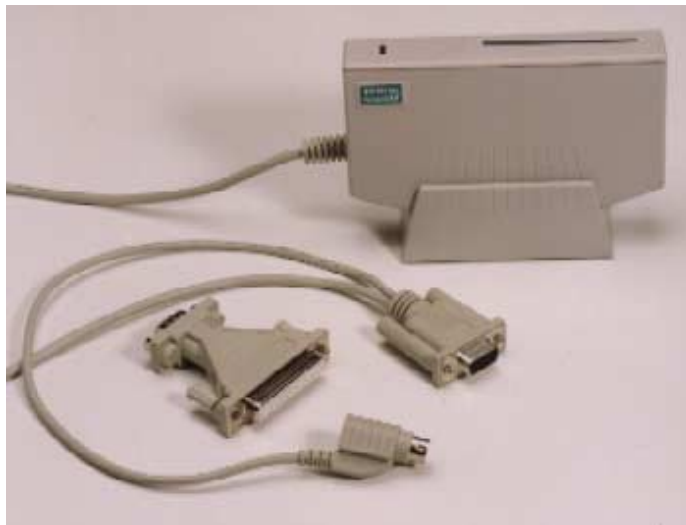
Chipcard reader B1 Snuggle is powered by the PS2 port
