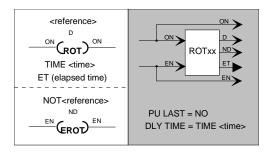
initialized to FALSE and the elapsed timer will be initialized to 0. *{This function and its associated EROT corresponds to a ROT function block with the PU LAST set to NO, the left horizontal shunt connected to the ON input, and the D output corresponding to the reference. The left horizontal shunt of the corresponding EROT coil is connected to the EN input. }*
