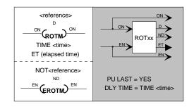
timer will be initialized to their previous values. {This function and the matching EROTM corresponds to a ROT function block with the PU LAST set to YES, the left horizontal shunt connected to the ON input, and the D output corresponding to the reference. The left horizontal shunt of the associated EROTM coil is connected to the EN input. }
