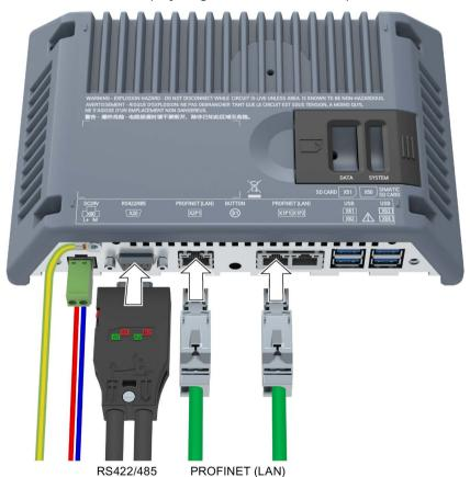
Use the PROFINET (LAN) X1 or X2 interface for SIMATIC process connection. Use the RS 422/485 interface for controllers from other manufacturers that are connected at the serial interface. Additional information on compatible controllers is available in the section "Communication with controllers (Page 187)".
