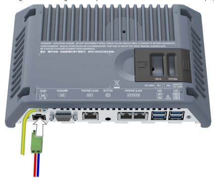
4. Verify the correct polarity of the cables using the interface labeling on the back of the HMI device.
