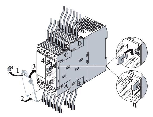
Figure 4-4 Mounting accessories for sealing the device
