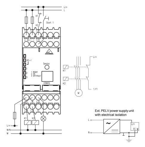
Figure 5-2 Connection overview of AS-Interface safety monitor type 1 and type 3
