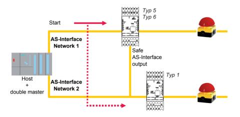
Figure 1-3 Example - Safe coupling of two AS-Interface networks
