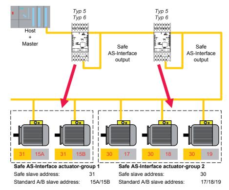
Figure 1-2 Example - Monitoring of 2 decentral AS-Interface actuator groups
