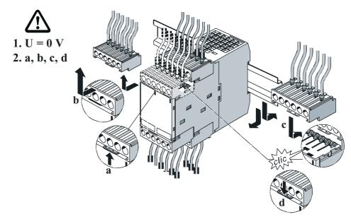
Figure 4-3 Removing and mounting encoded connection terminals
