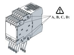
Figure 4-2 Removable connection terminals
