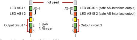
Figure 9-1 Overview of device LEDs
