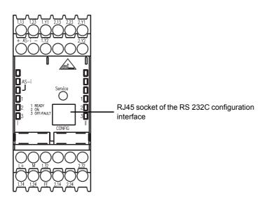
Figure 8-2 Location of the RS 232C configuration interface
