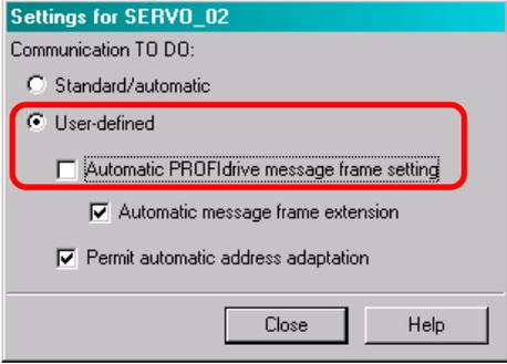
11. The correct message frames must be selected for the cyclic communication to the CU and to the two servo motors. Because the “Standard telegram 1” does not support any IRT communication, at least “Standard telegram 2” must be selected for SERVO\_02 and SERVO\_03!
