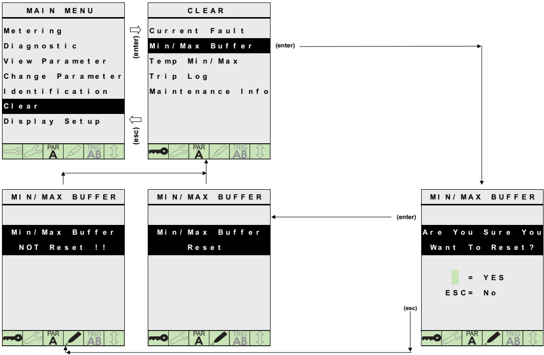
Example 13: Resetting the measured minimum and maximum values
