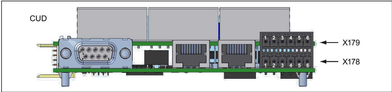
Figure 6-52 Arrangement X178 and X179
