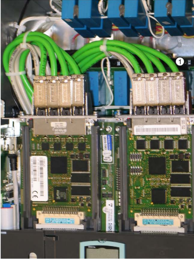
Figure 6-13 Routing PROFINET cables in devices >280 A
