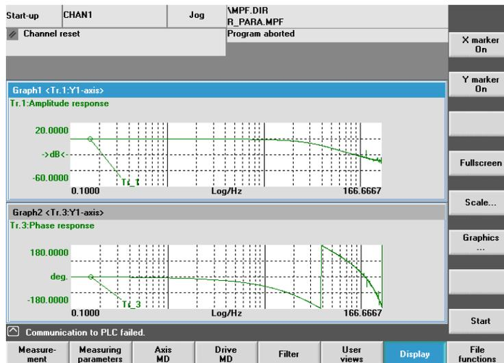
Figure 11-7 Optimized position control loop
