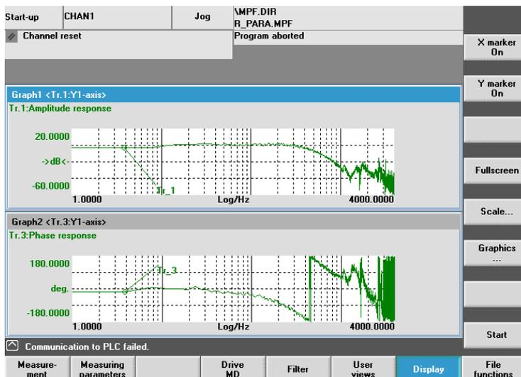
Figure 11-6 Optimized speed control loop
