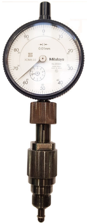
Figure 5-19 Example calibration tool with dial gauge, from Comau
