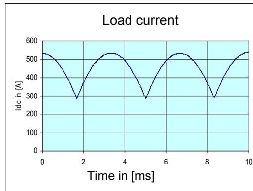
Without smoothing reactor, current at point of transition from discontinuous to continuous current, i.e. current maximum values just touch the zero line; point of transition from discontinuous to continuous current (example half motor nominal speed) is 31 % of  $I_N$ .
