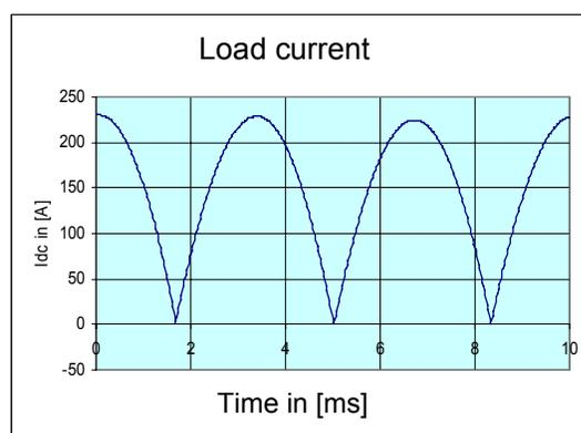
Discontinuous current, half rated motor speed, without smoothing reactor
