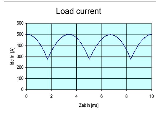
When motor speed is zero,  $I_N \rightarrow \alpha = 88$  degrees; the resulting current ripple is 19% rms
