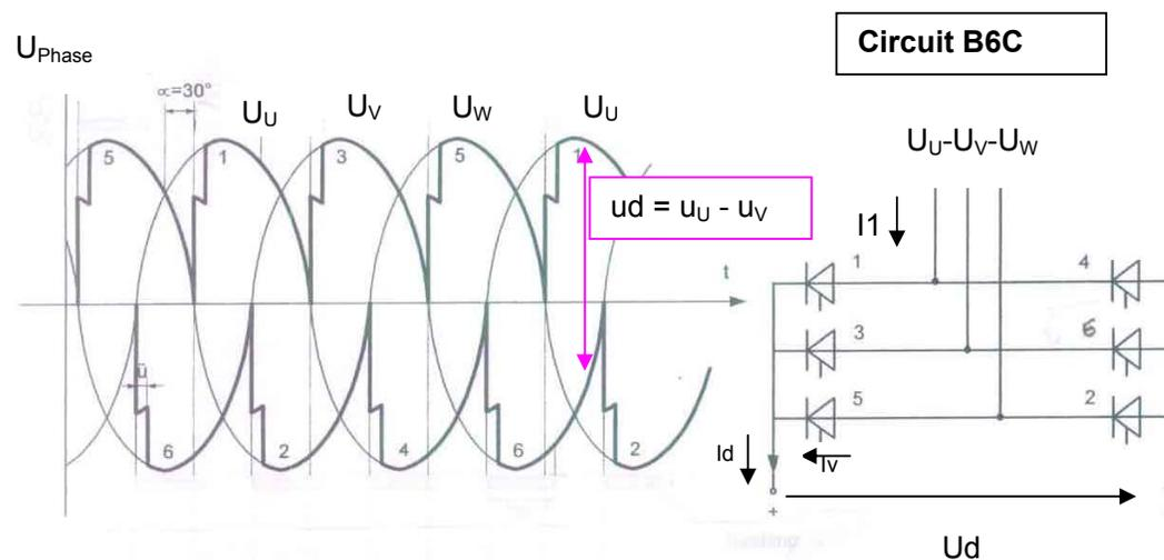
The momentary value of the output direct voltage can be read from the voltage characteristic above for the delay angle  $\alpha = 30$  degrees.
