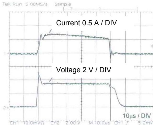
Check the firing trigger:
