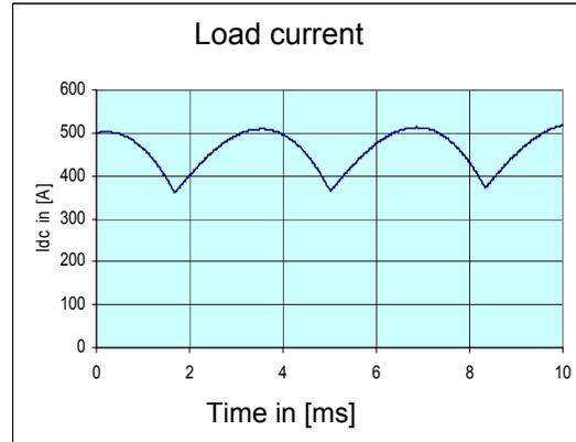
As above for smoothing reactor 1.5 mH, the resulting current ripple is 4.5 % rms
