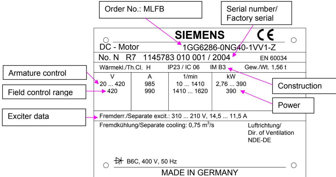
Rated motor voltage: 420 V, rated motor current 985 A
