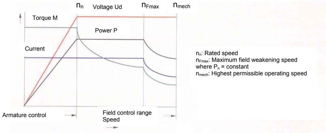
**Armature control range:** The armature and the power at constant current increase proportionally to the speed. The rated motor voltage is reached when the rated speed is at nominal flux.
