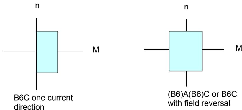
The converter generates a variable direct voltage a function of a variable firing angle by rectification of the line voltage. The firing angle determines the firing time of the thyristor and thus the magnitude of the variable output direct voltage.
