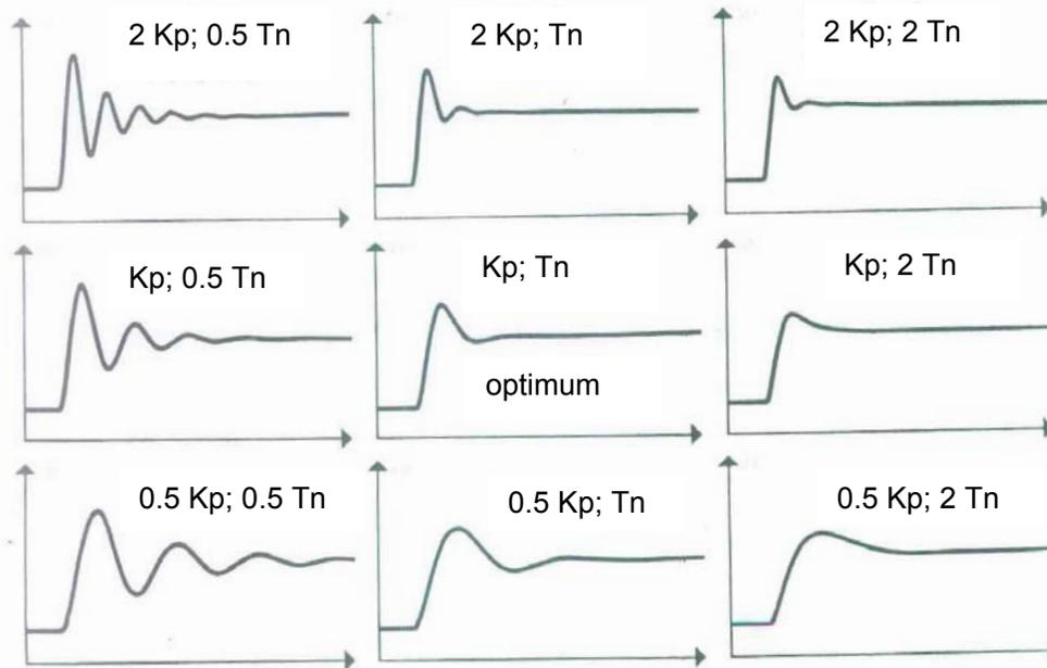
Adjustment according to the symmetrical optimum
