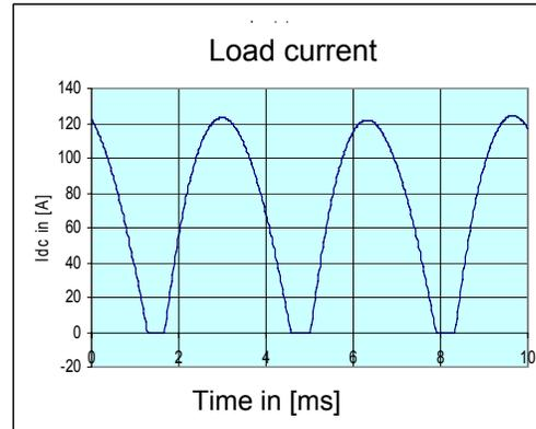
**Measurement of current characteristic of line-side current:** During the positive half-wave of the line-to-line line voltage, two positive current peaks occur, then a pause for the duration of the current maximum value, then two negative current maximum values during the negative half-wave of the line voltage. If the two positive or negative current maximum values are missing, the thyristor does not fire.
