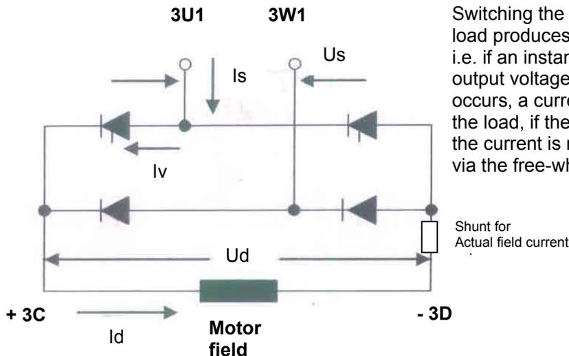
Switching the diodes parallel to the load produces a free-wheeling arm, i.e. if an instantaneous value of the output voltage greater than zero occurs, a current flow builds up via the load, if the output voltage is zero, the current is reduced toward zero via the free-wheeling arm.
