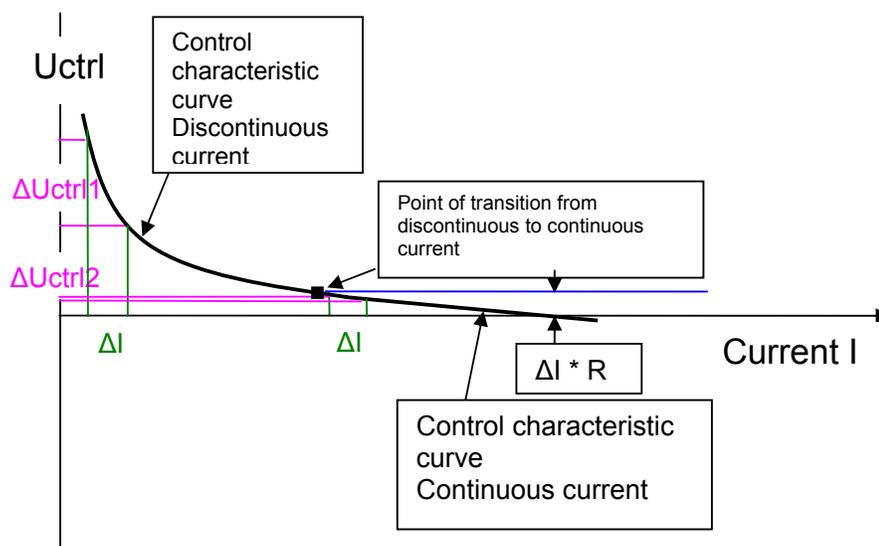
To effect a current change  $\Delta I$  a firing angle change  $\Delta U_{ctrl}$  must be applied. If  $\Delta I$  is equal, the necessary control firing angle  $\Delta U_{ctrl1}$  in the discontinuous current range is much higher than  $\Delta U_{ctrl2}$  in the continuous current range. The firing angle change only has to take account of the armature-current-related linear voltage drop  $I * R$  in the continuous current range.
