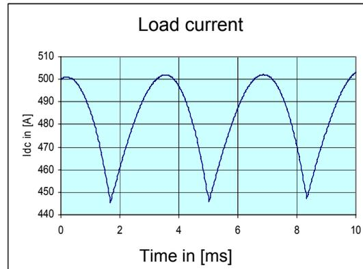
Half the rated motor speed, without smoothing reactor,  $I_N$  →  $\alpha = 65$  degrees
